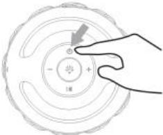
**ON/OFF Button:** Long press this button for 2 seconds to turn ON/OFF the Bluetooth speaker; short press button to connect with the other Bluetooth speaker; LED light flashes means Bluetooth is turned on, steady light means Bluetooth connection successful.
