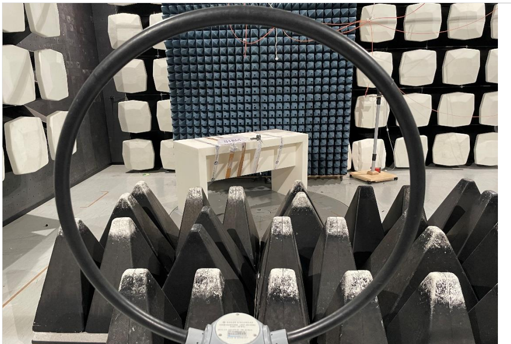
Photograph 4: H-field EUT test setup in the semi anechoic chamber, overview
