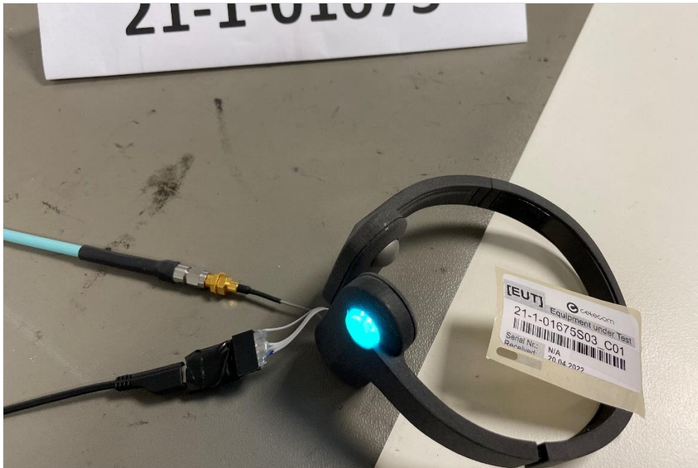
Photograph 7: EUT setup conducted measurement, close up view
