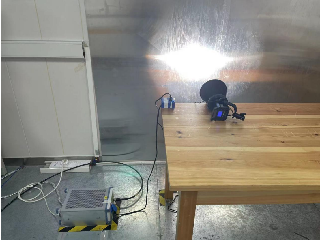
Conducted emission test setup
