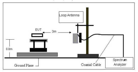
(B) Radiated Emission Test-Up Frequency 30MHz~1GHz
