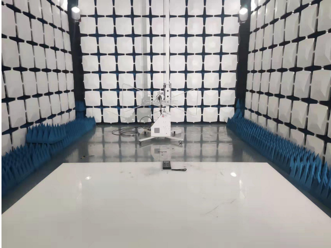
Above 1GHz for radiated emission test setup
