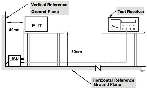
Note: 1.Support units were connected to second LISN.2.Both of LISNs (AMN) are 80 cm from EUT and at least 80 from other units and other metal planes
