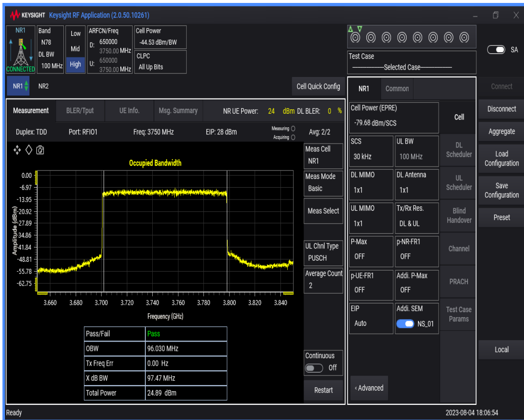
n78(3700-3800) SCS=30kHz DFT_BPSK BW=10MHz Channel=650000 RB=24@0
