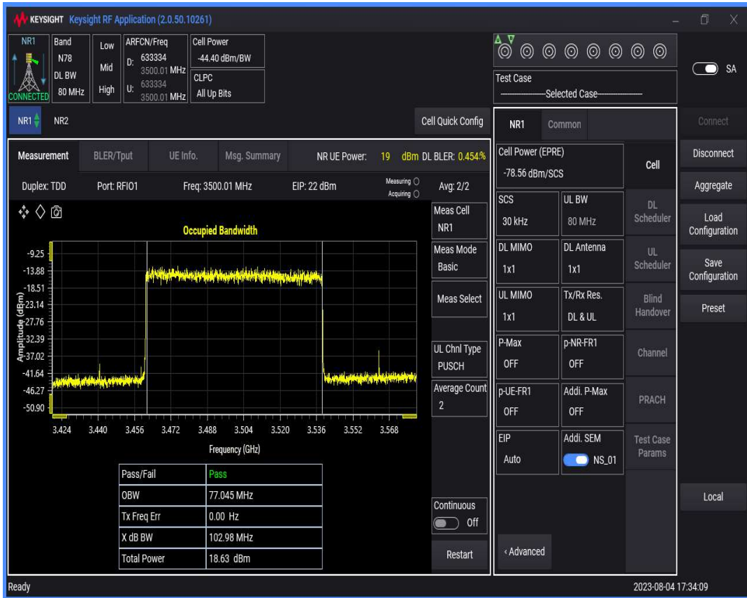
n78(3450-3550) SCS=30kHz DFT_QAM256 BW=90MHz Channel=633334 RB=240@0
