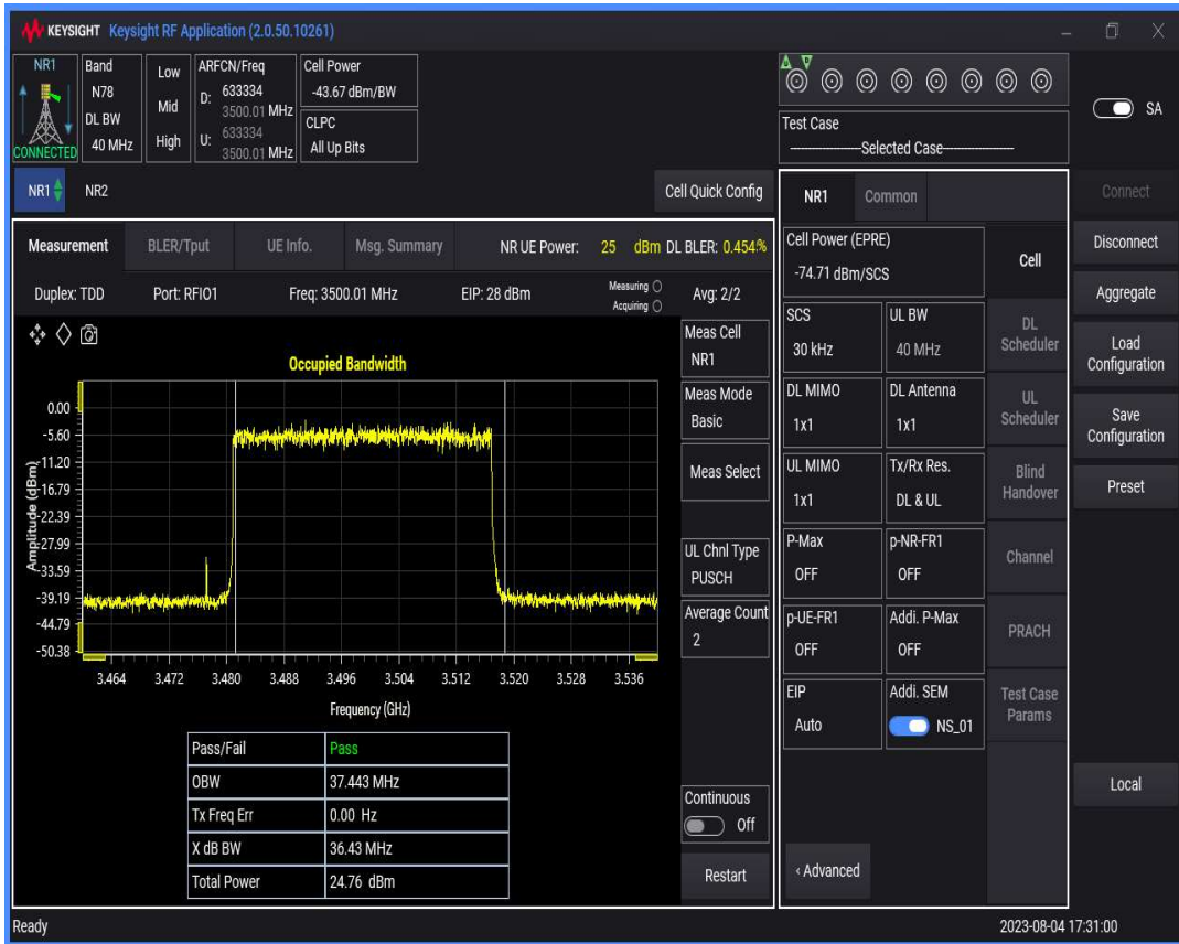
n78(3450-3550) SCS=30kHz DFT_QPSK BW=50MHz Channel=633334 RB=128@0
