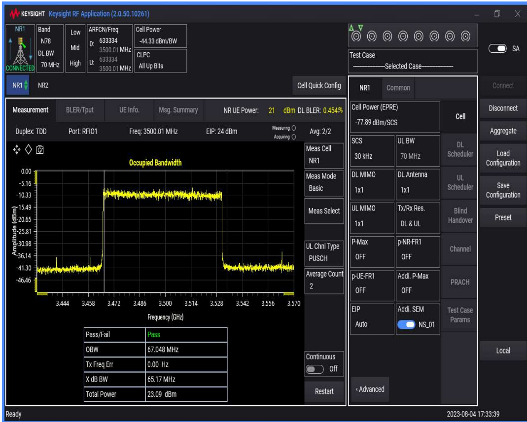
n78(3450-3550) SCS=30kHz DFT_QAM16 BW=80MHz Channel=633334 RB=216@0
