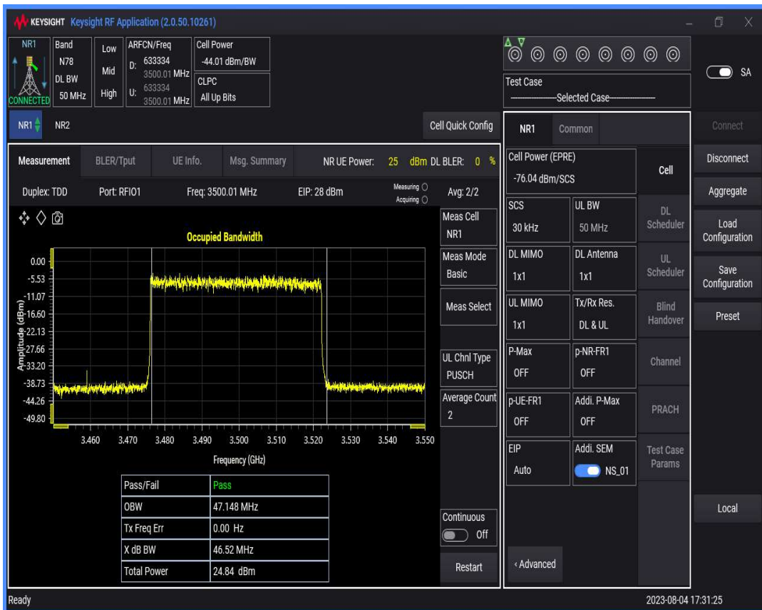
n78(3450-3550) SCS=30kHz DFT_QPSK BW=60MHz Channel=633334 RB=162@0
