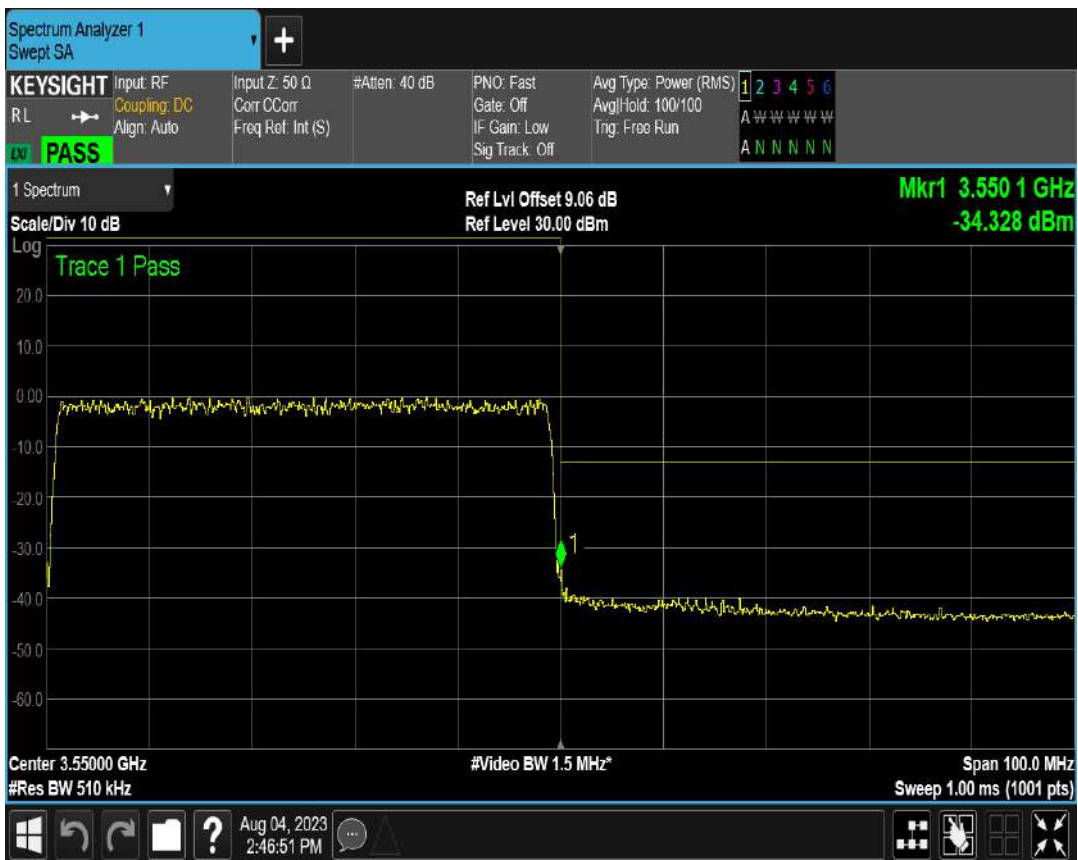
n78(3450-3550) SCS=30kHz CP_QPSK BW=50MHz Channel=635000 RB=1@0
