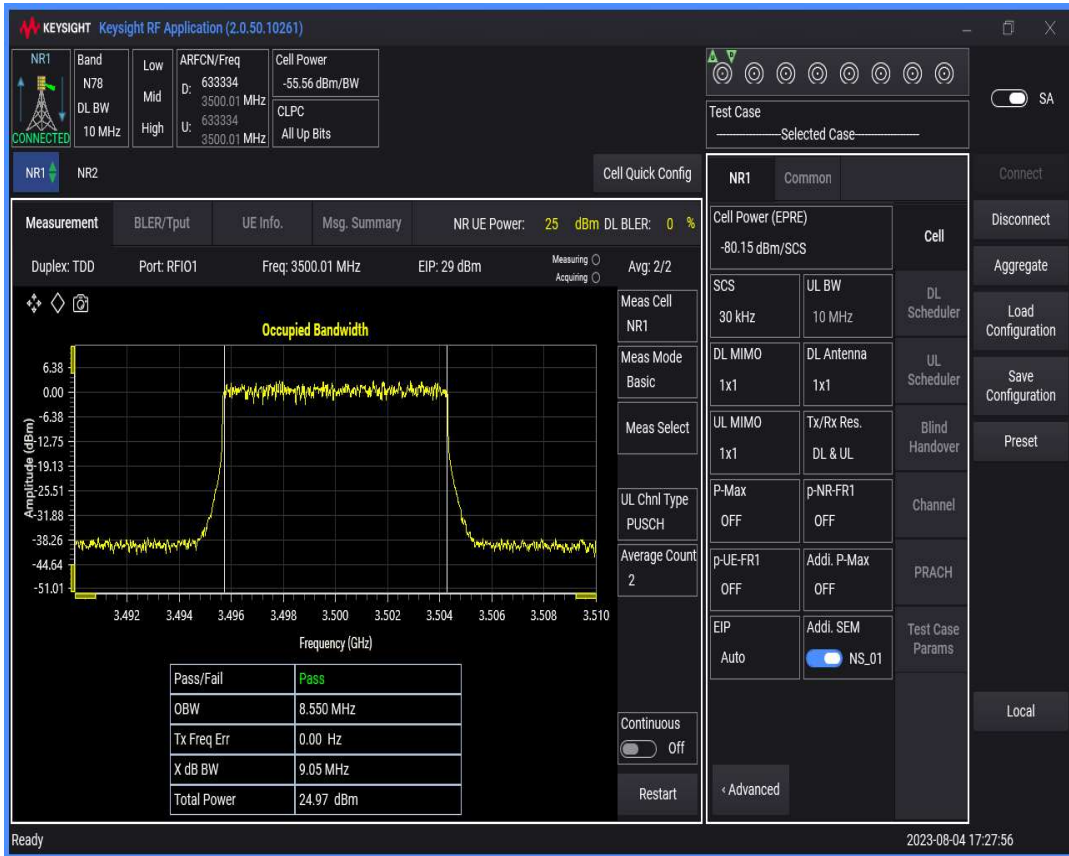
n78(3450-3550) SCS=30kHz DFT_BPSK BW=15MHz Channel=633334 RB=36@0
