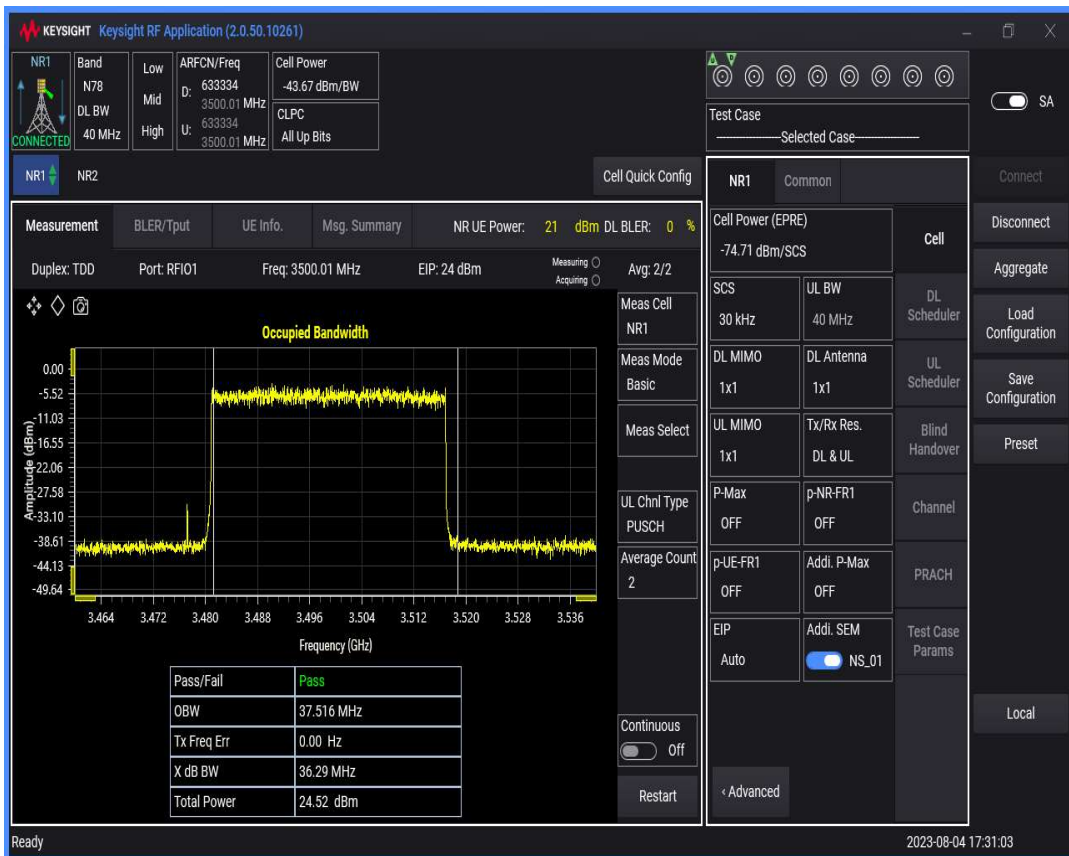
n78(3450-3550) SCS=30kHz DFT_QAM16 BW=50MHz Channel=633334 RB=128@0
