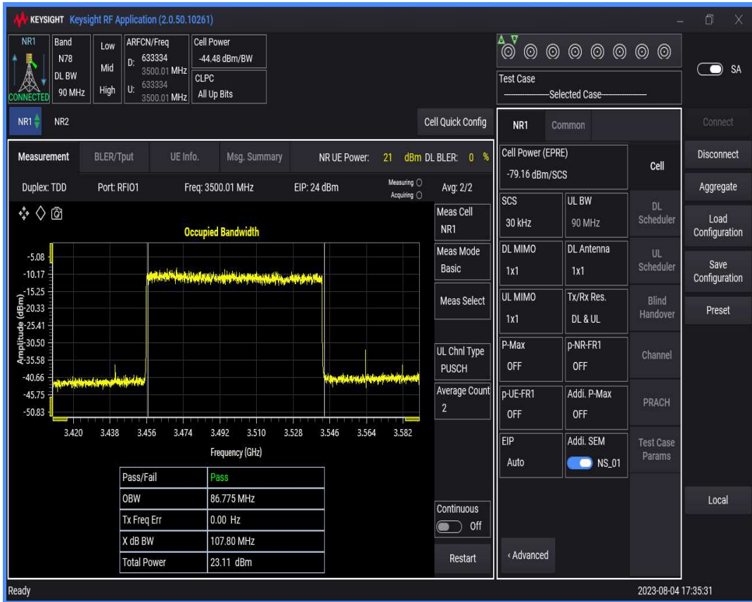
n78(3450-3550) SCS=30kHz DFT_QAM256 BW=100MHz Channel=633334 RB=270@0
