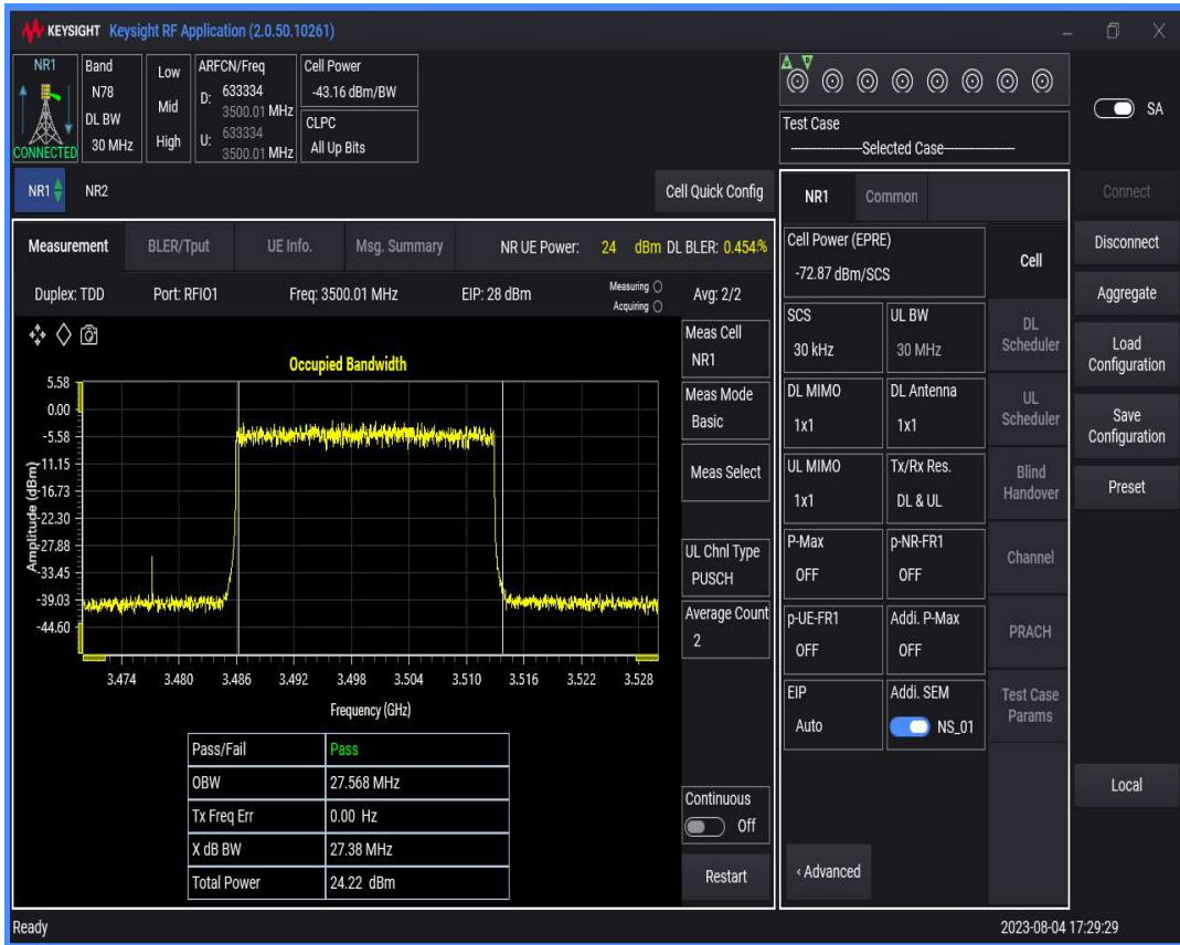
n78(3450-3550) SCS=30kHz DFT_QAM64 BW=40MHz Channel=633334 RB=100@0
