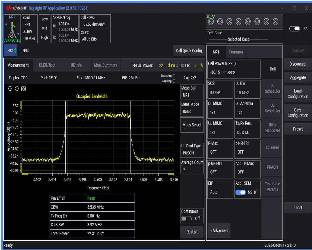
n78(3450-3550) SCS=30kHz DFT_QAM256 BW=15MHz Channel=633334 RB=36@0
