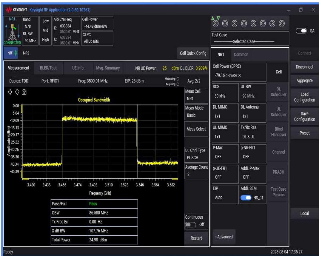
n78(3450-3550) SCS=30kHz DFT_QPSK BW=90MHz Channel=633334 RB=240@0
