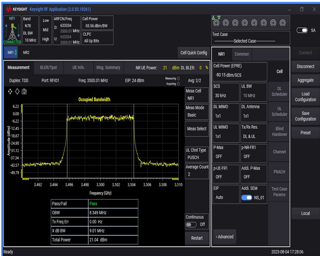
n78(3450-3550) SCS=30kHz DFT_QAM16 BW=15MHz Channel=633334 RB=36@0
