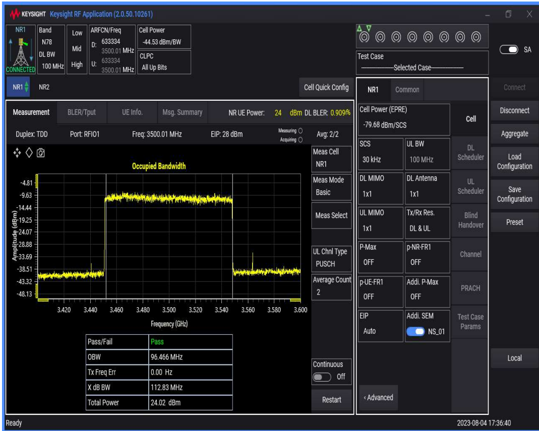
n78(3450-3550) SCS=30kHz DFT_QAM64 BW=10MHz Channel=633334 RB=24@0
