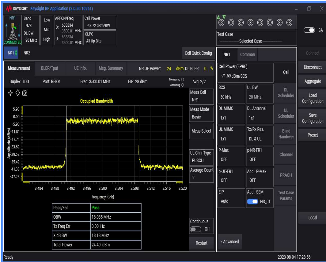
n78(3450-3550) SCS=30kHz DFT_QPSK BW=30MHz Channel=633334 RB=75 @0
