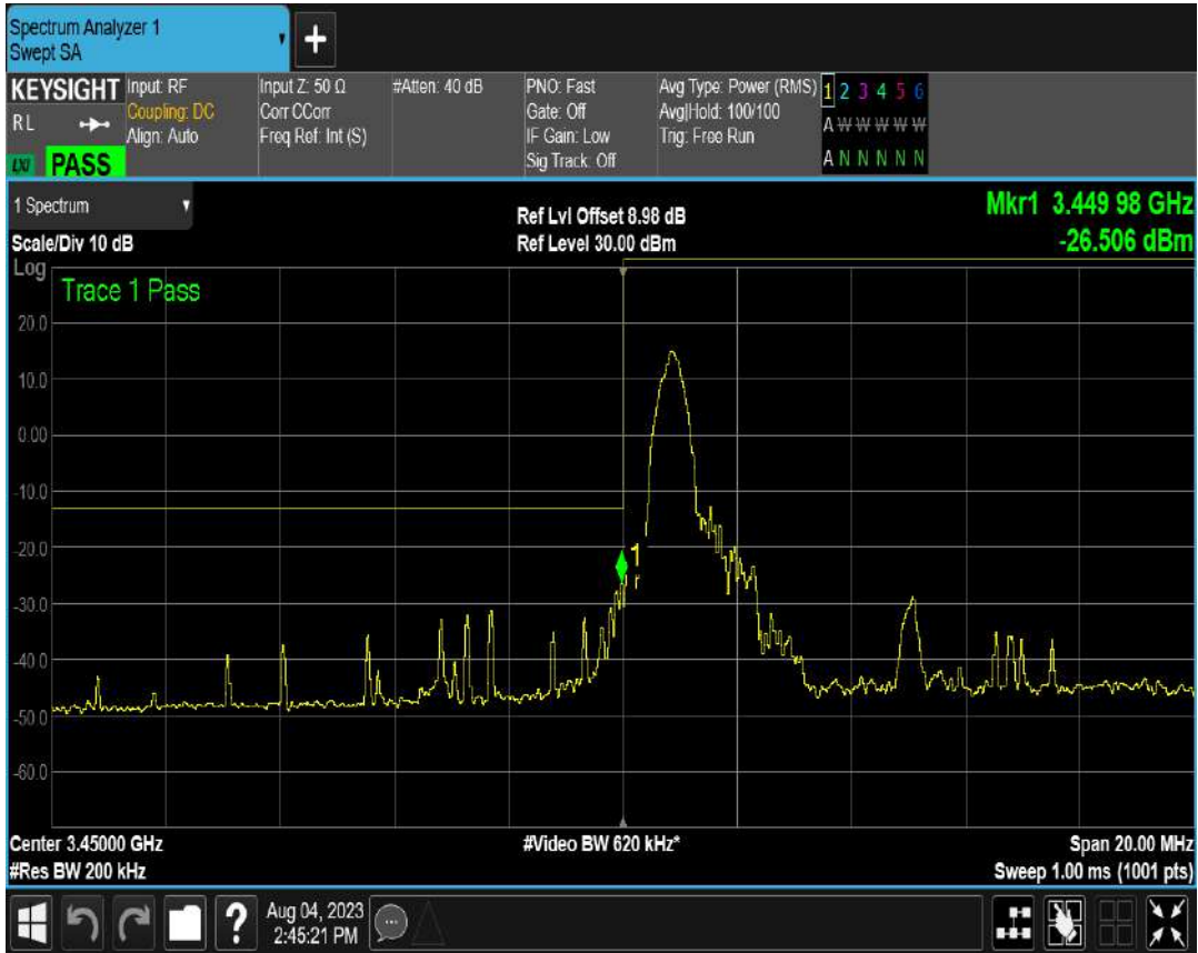
n78(3450-3550) SCS=30kHz CP_QPSK BW=10MHz Channel=630334 RB=1@23
