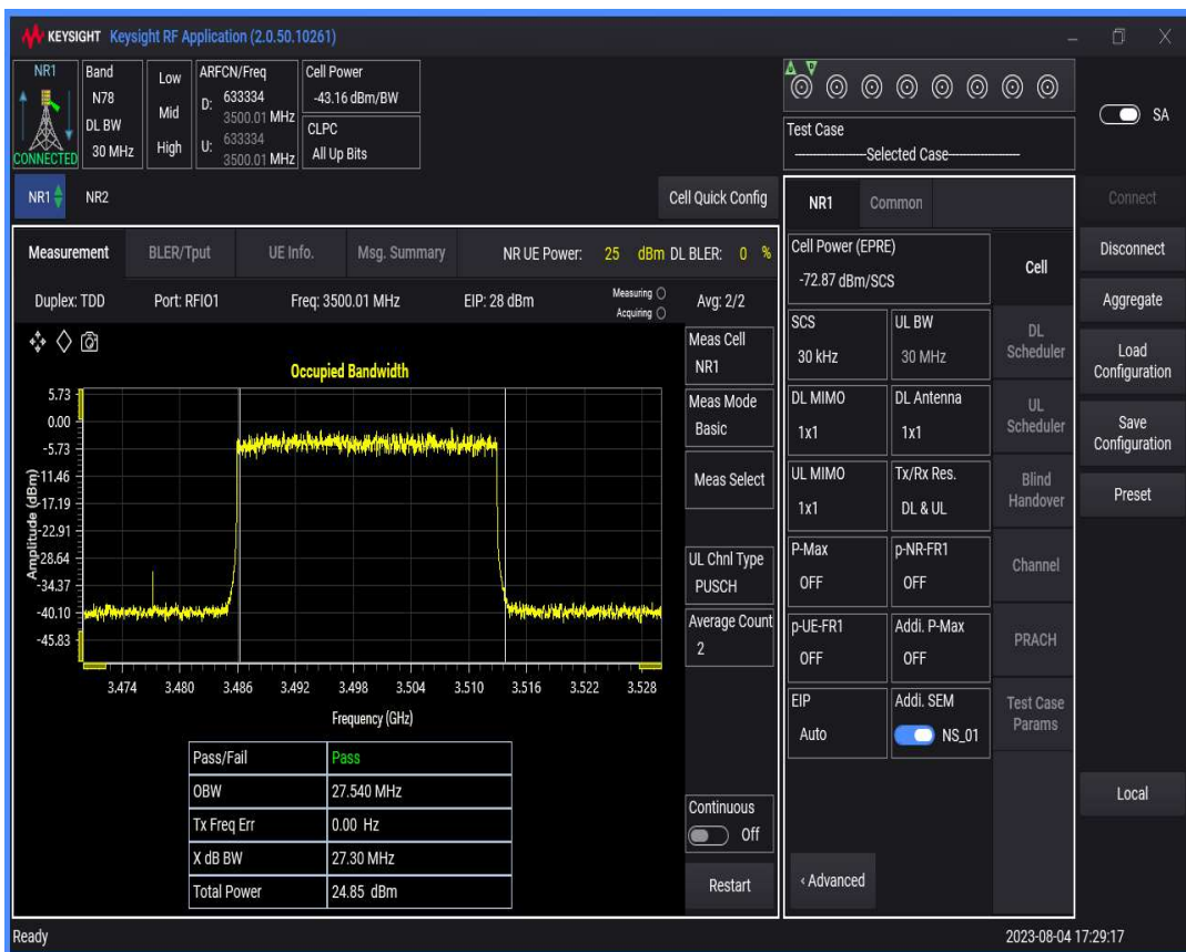
n78(3450-3550) SCS=30kHz DFT_BPSK BW=40MHz Channel=633334 RB=100@0
