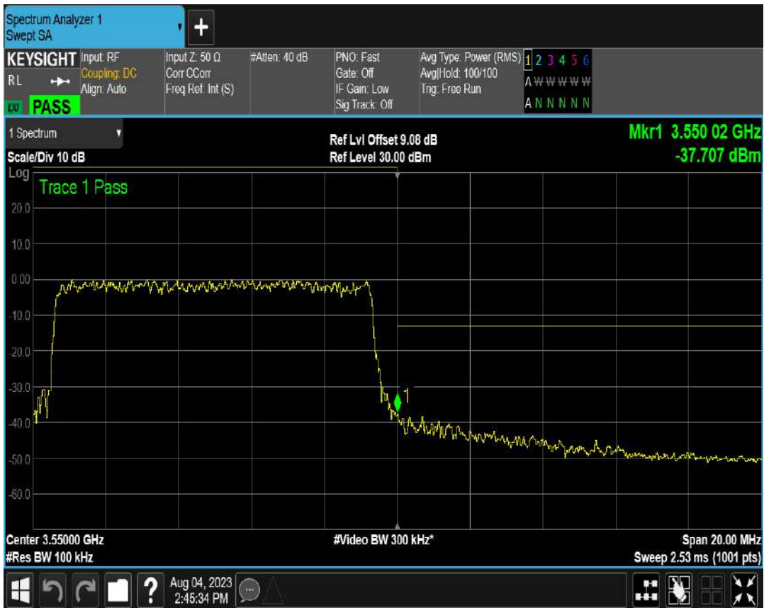
n78(3450-3550) SCS=30kHz CP_QPSK BW=50MHz Channel=631668 RB=133@0
