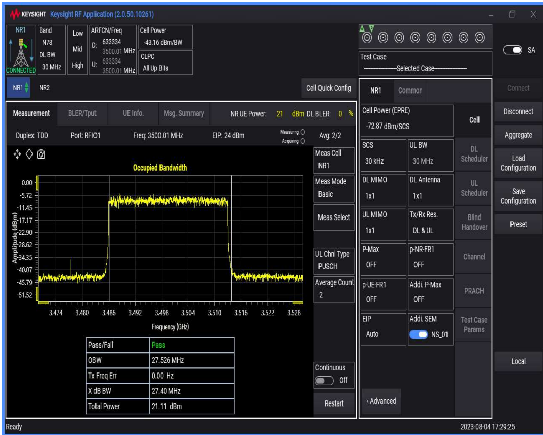
n78(3450-3550) SCS=30kHz DFT_QAM16 BW=40MHz Channel=633334 RB=100@0
