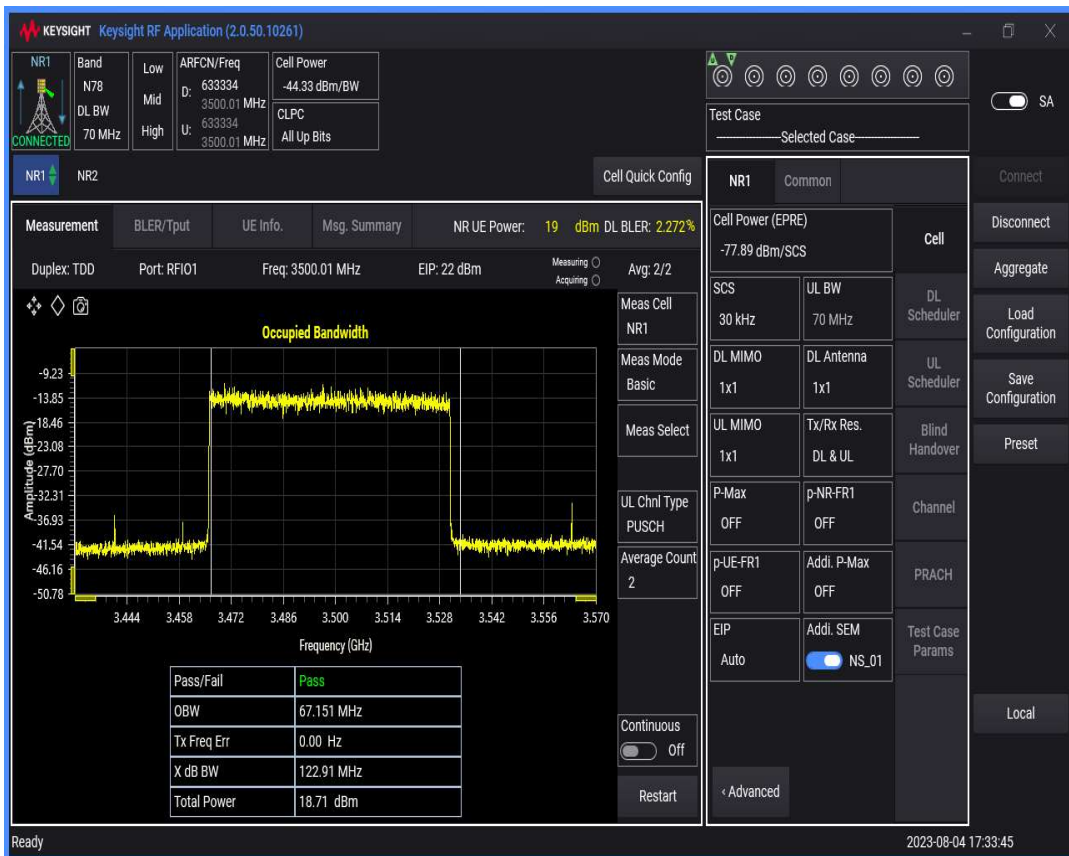
n78(3450-3550) SCS=30kHz DFT_QAM256 BW=80MHz Channel=633334 RB=216 @0
