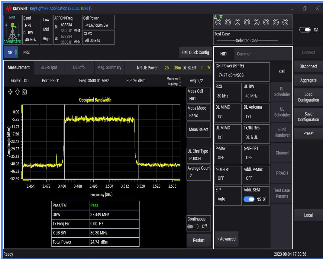
n78(3450-3550) SCS=30kHz DFT_BPSK BW=50MHz Channel=633334 RB=128@0
