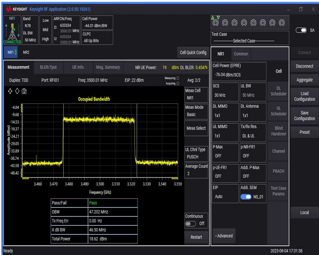
n78(3450-3550) SCS=30kHz DFT_QAM256 BW=60MHz Channel=633334 RB=162@0
