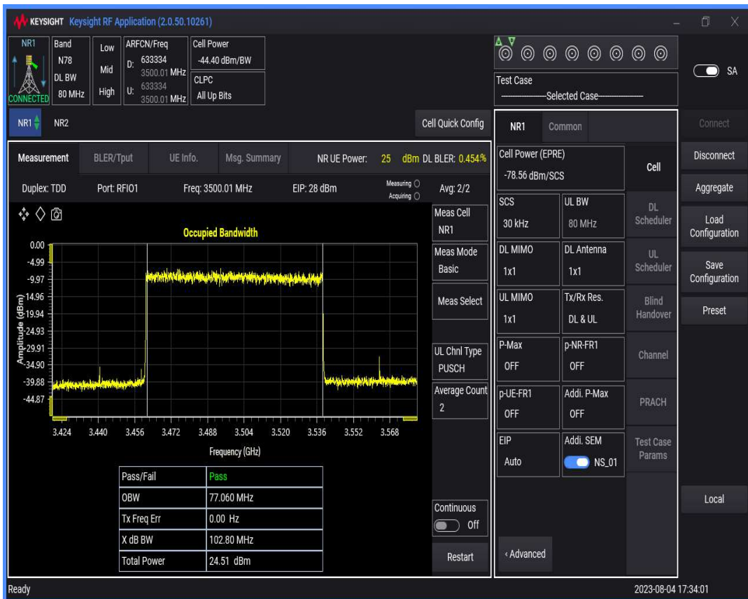
n78(3450-3550) SCS=30kHz DFT_QAM16 BW=90MHz Channel=633334 RB=240@0
