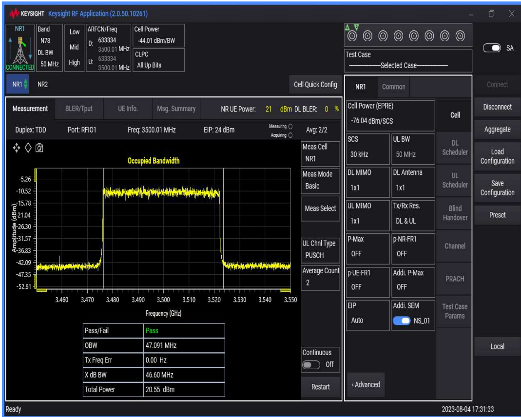
n78(3450-3550) SCS=30kHz DFT_QAM64 BW=60MHz Channel=633334 RB=162@0
