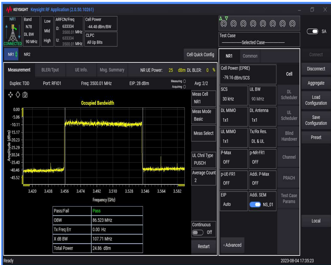
n78(3450-3550) SCS=30kHz DFT_QAM16 BW=100MHz Channel=633334 RB=270@0
