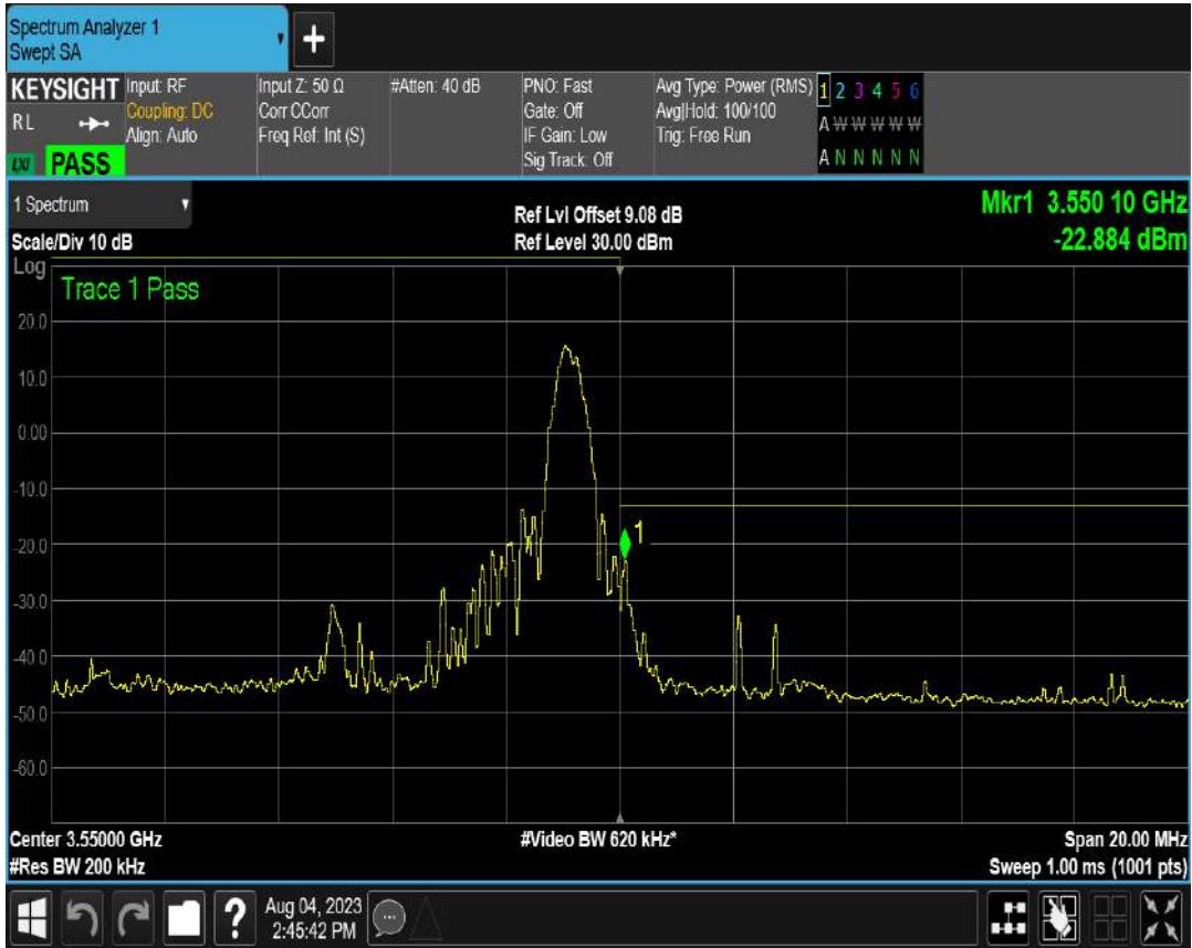
n78(3450-3550) SCS=30kHz CP_QPSK BW=10MHz Channel=636332 RB=24@0
