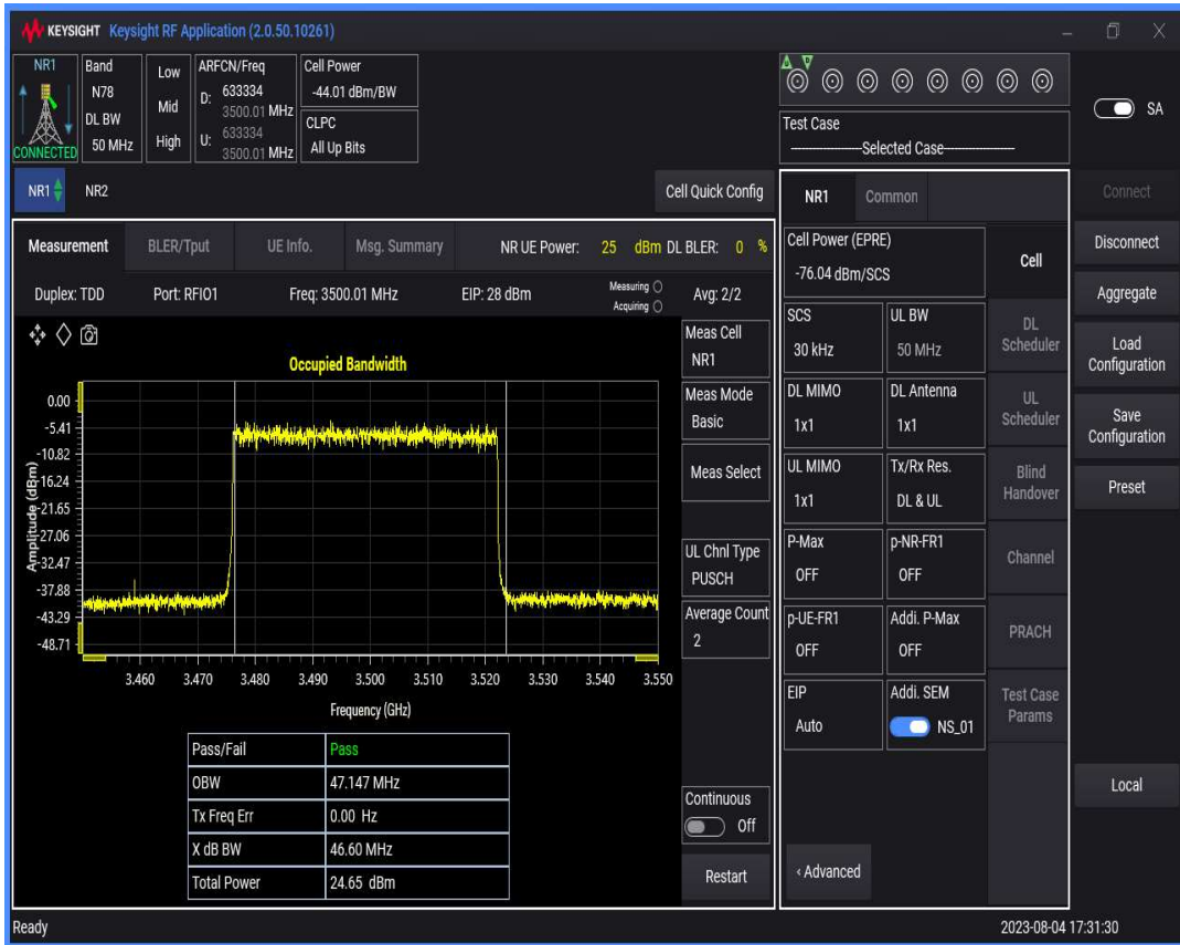
n78(3450-3550) SCS=30kHz DFT_QAM16 BW=60MHz Channel=633334 RB=162@0
