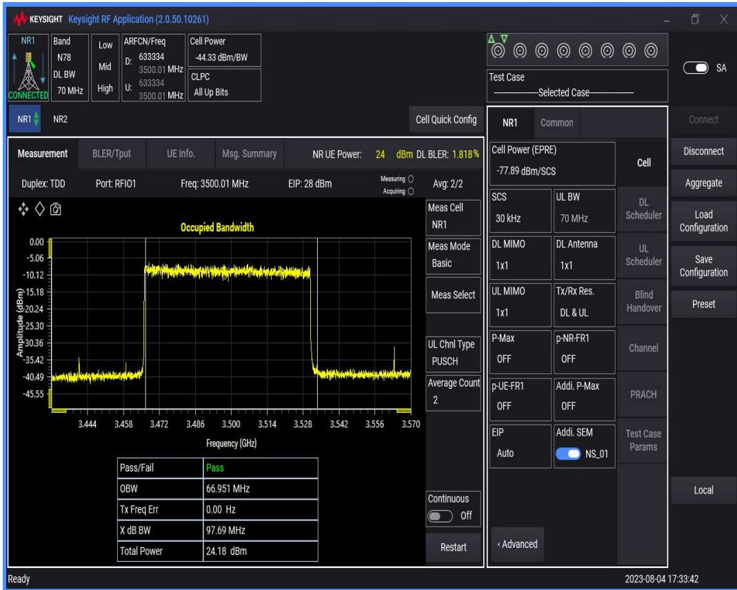
n78(3450-3550) SCS=30kHz DFT_QAM64 BW=80MHz Channel=633334 RB=216@0
