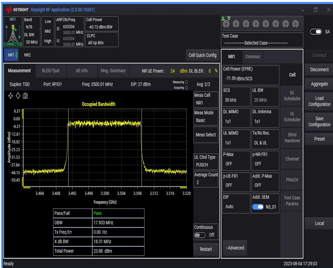
n78(3450-3550) SCS=30kHz DFT_QAM64 BW=30MHz Channel=633334 RB=75@0
