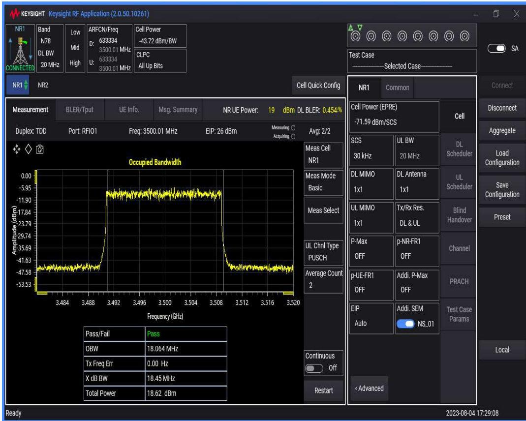
n78(3450-3550) SCS=30kHz DFT_QAM256 BW=30MHz Channel=633334 RB=75 @0
