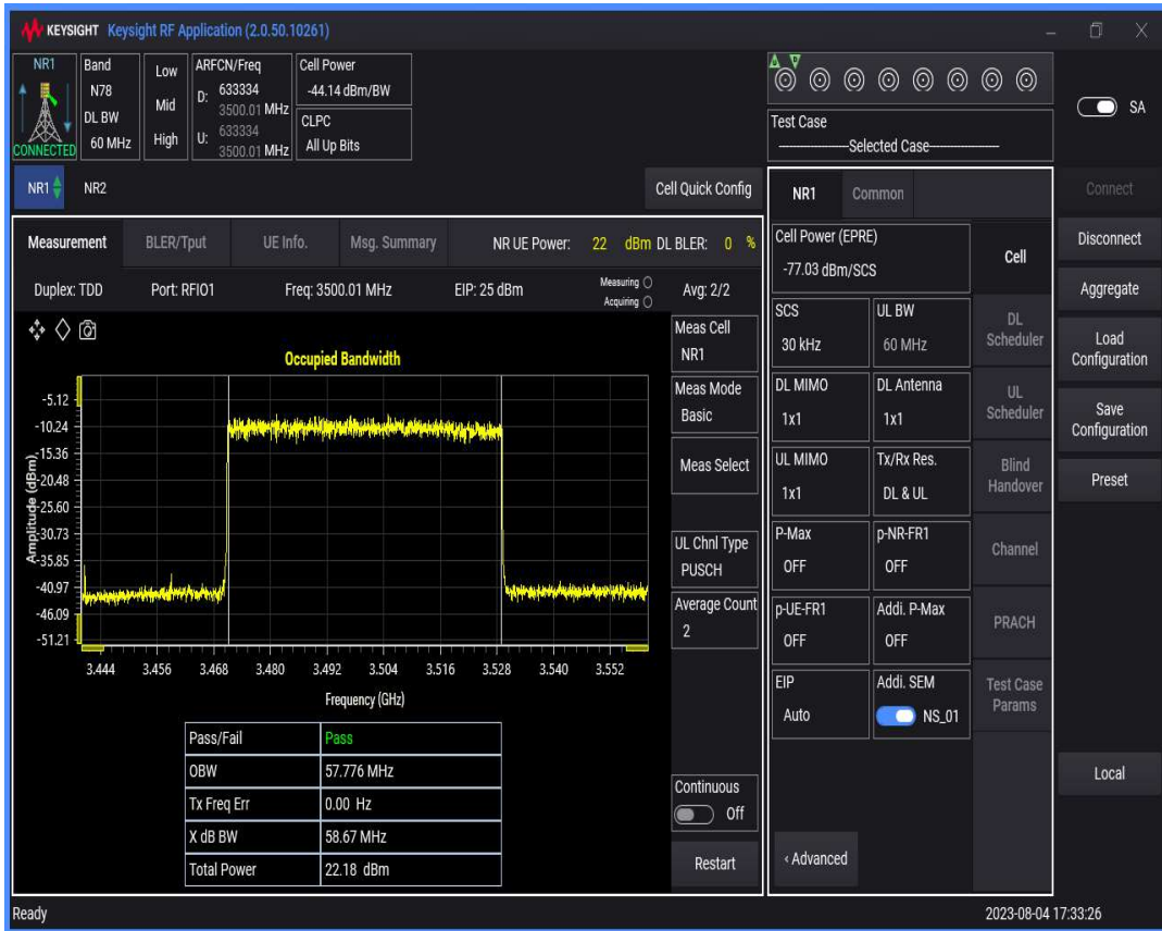
n78(3450-3550) SCS=30kHz DFT_QAM256 BW=70MHz Channel=633334 RB=
