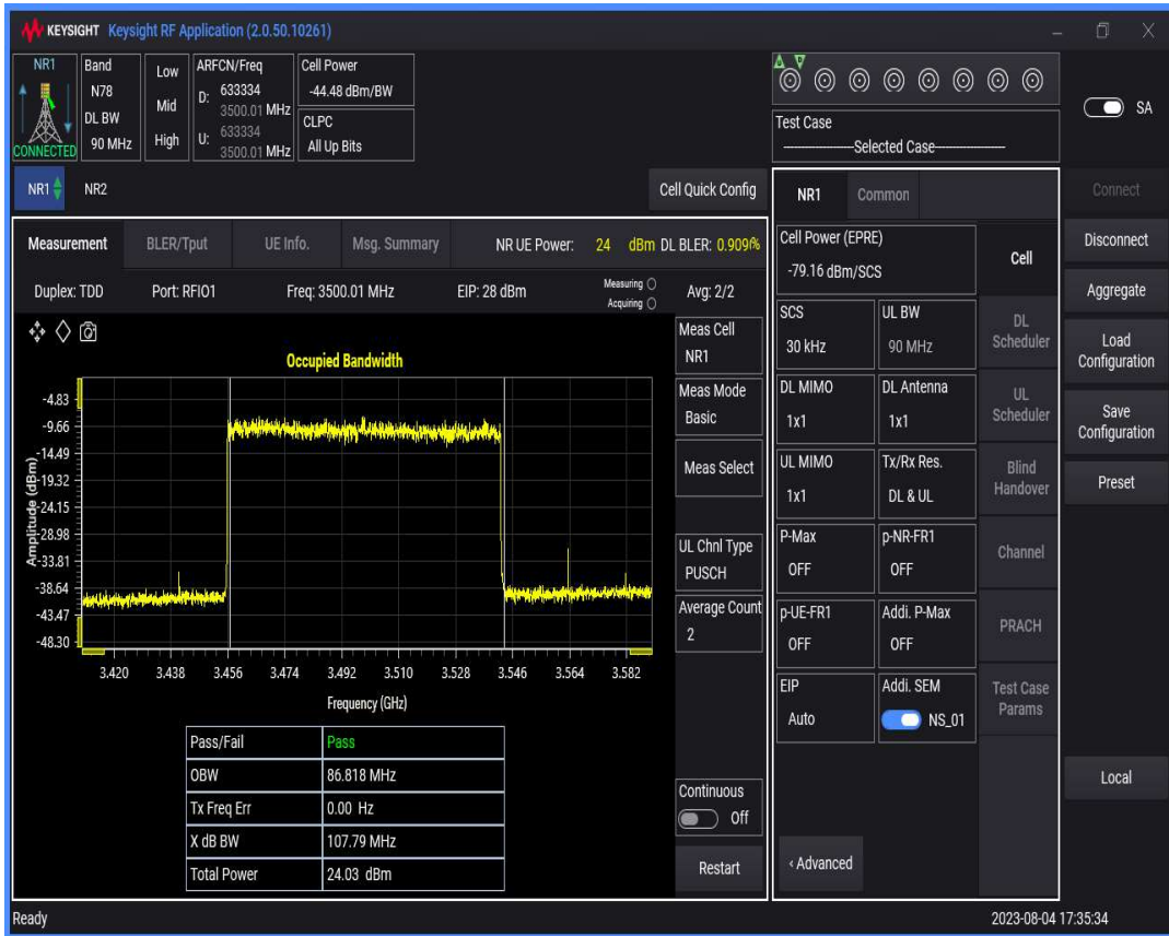
n78(3450-3550) SCS=30kHz DFT_QPSK BW=100MHz Channel=633334 RB=270@0
