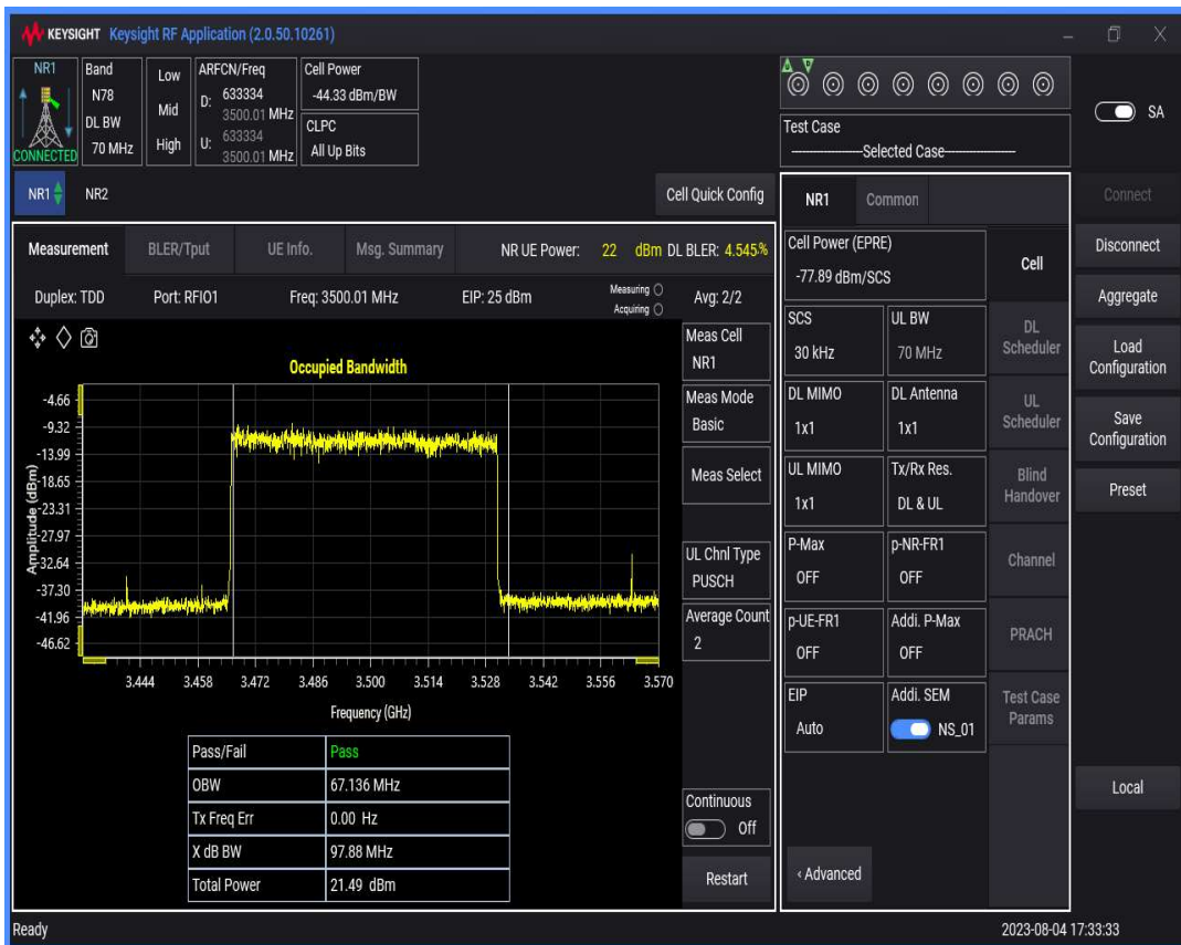
n78(3450-3550) SCS=30kHz DFT_BPSK BW=80MHz Channel=633334 RB=216 @0
