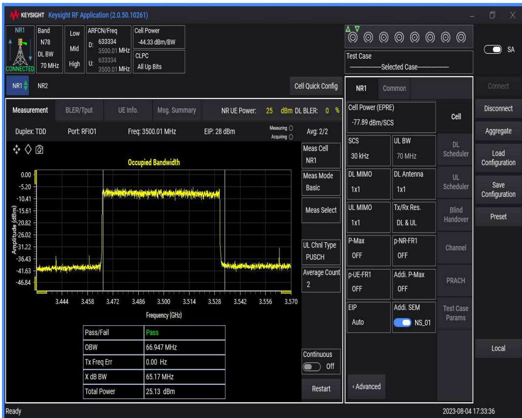
n78(3450-3550) SCS=30kHz DFT_QPSK BW=80MHz Channel=633334 RB=216 @0
