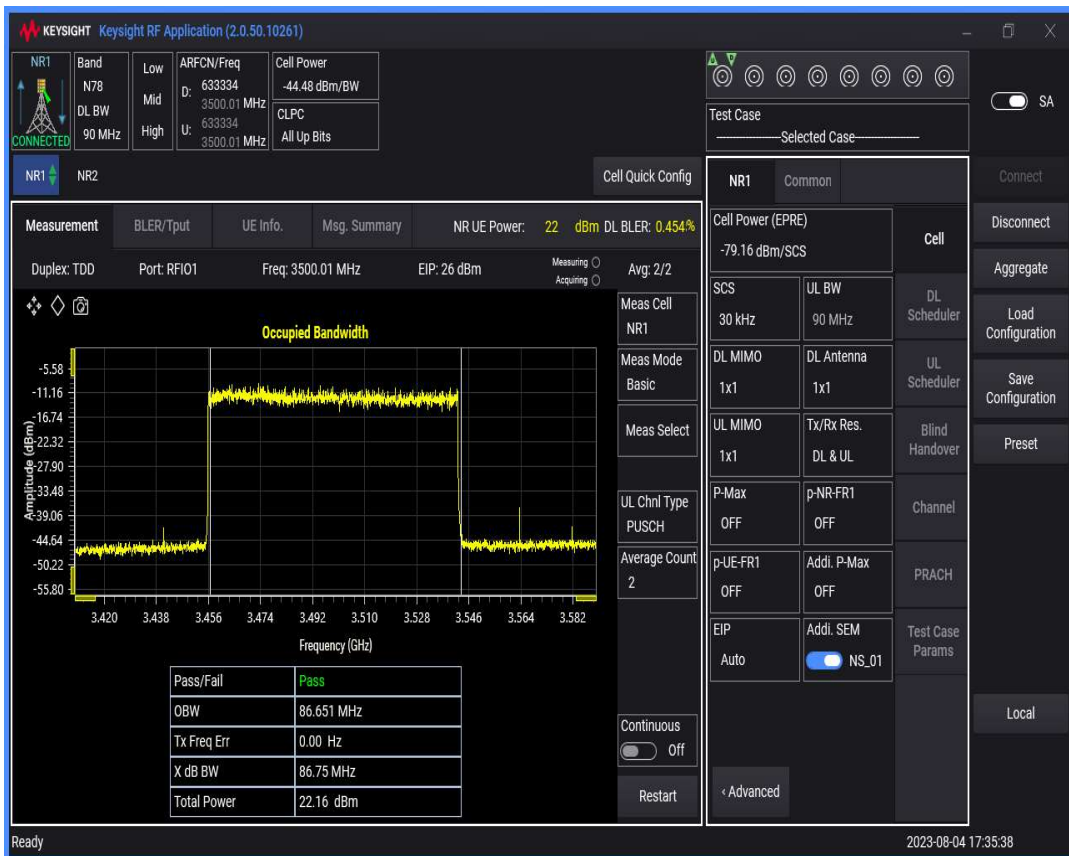
n78(3450-3550) SCS=30kHz DFT_QAM64 BW=100MHz Channel=633334 RB=270@0
