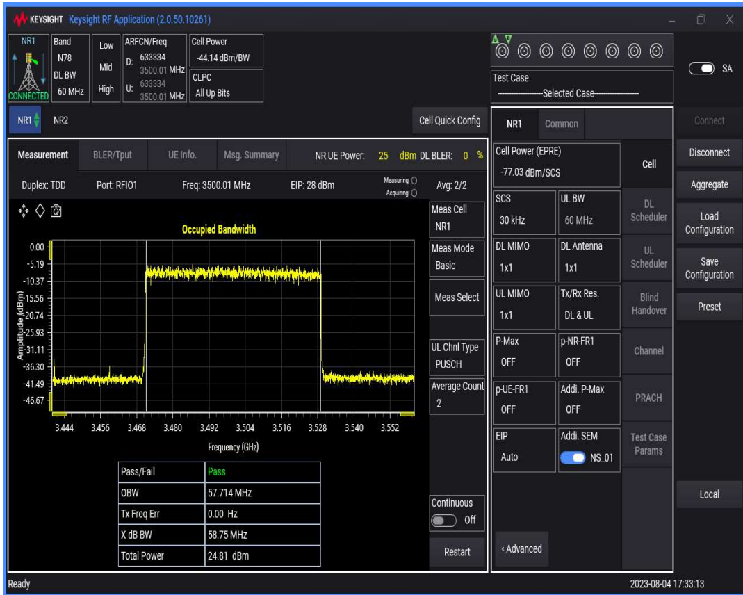
n78(3450-3550) SCS=30kHz DFT_QPSK BW=70MHz Channel=633334 RB=
