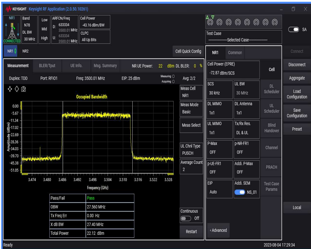
n78(3450-3550) SCS=30kHz DFT_QAM256 BW=40MHz Channel=633334 RB=100 @0
