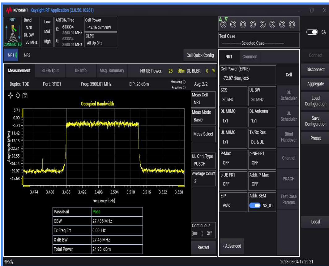
n78(3450-3550) SCS=30kHz DFT_QPSK BW=40MHz Channel=633334 RB=100 @0
