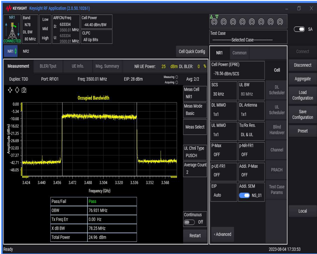
n78(3450-3550) SCS=30kHz DFT_BPSK BW=90MHz Channel=633334 RB=240@0
