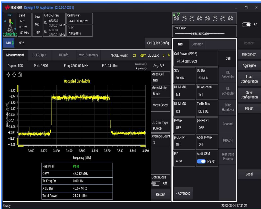
n78(3450-3550) SCS=30kHz DFT_BPSK BW=60MHz Channel=633334 RB=162@0
