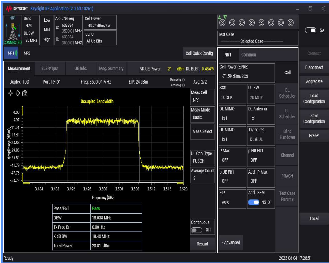
n78(3450-3550) SCS=30kHz DFT_BPSK BW=30MHz Channel=633334 RB=75@0
