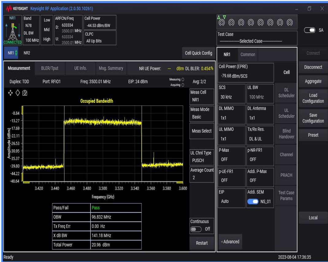
n78(3450-3550) SCS=30kHz DFT_QAM16 BW=10MHz Channel=633334 RB=24@0
