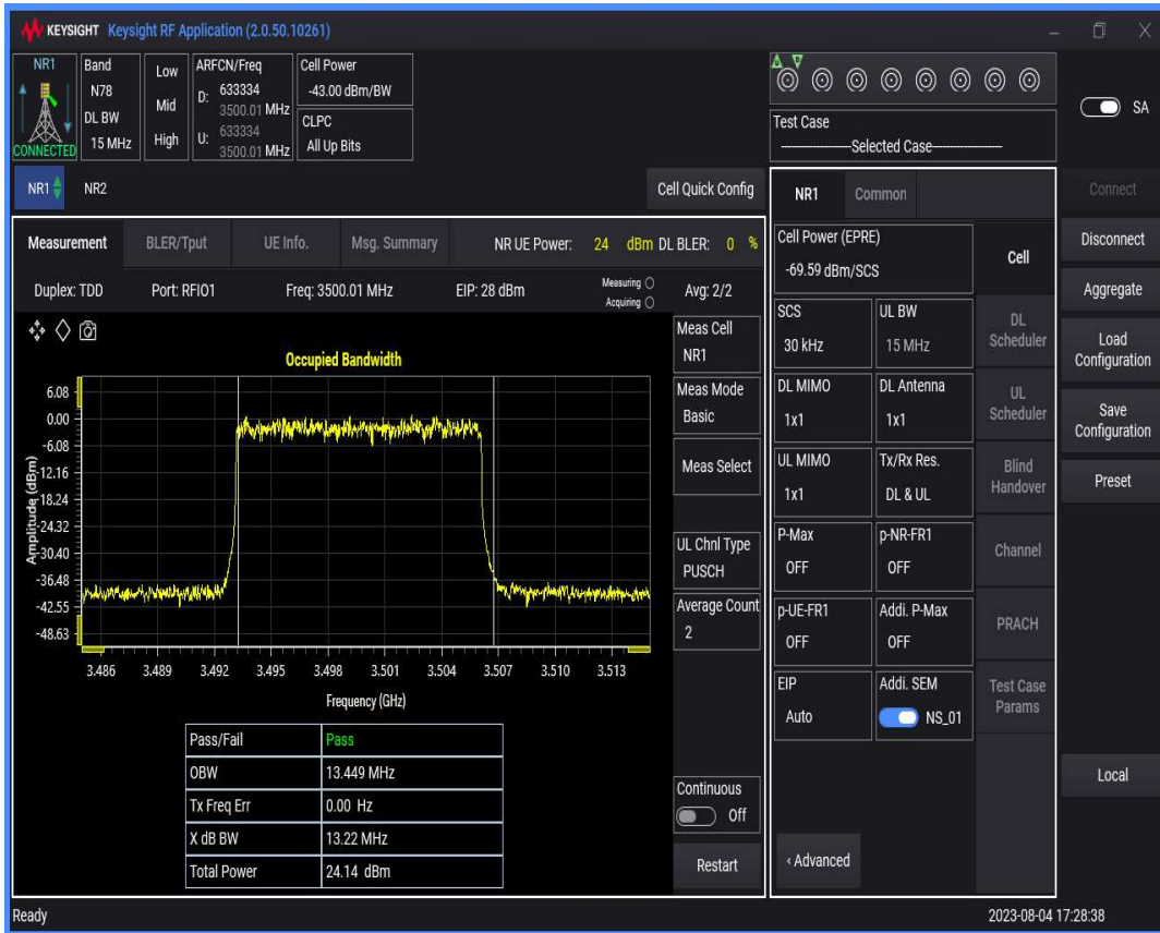
n78(3450-3550) SCS=30kHz DFT_QAM64 BW=20MHz Channel=633334 RB=50@0
