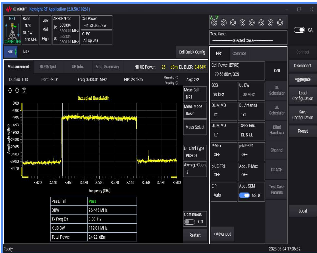
n78(3450-3550) SCS=30kHz DFT_QPSK BW=10MHz Channel=633334 RB=24@0
