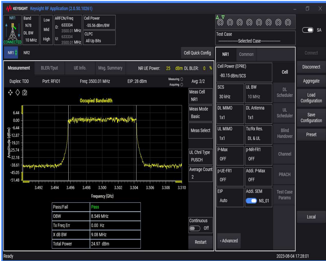
n78(3450-3550) SCS=30kHz DFT_QPSK BW=15MHz Channel=633334 RB=36@0
