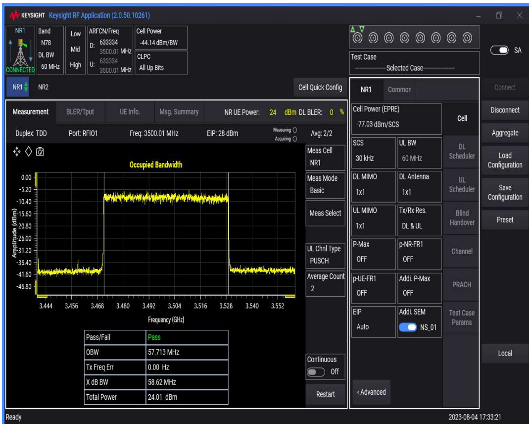
n78(3450-3550) SCS=30kHz DFT_QAM64 BW=70MHz Channel=633334 RB=
