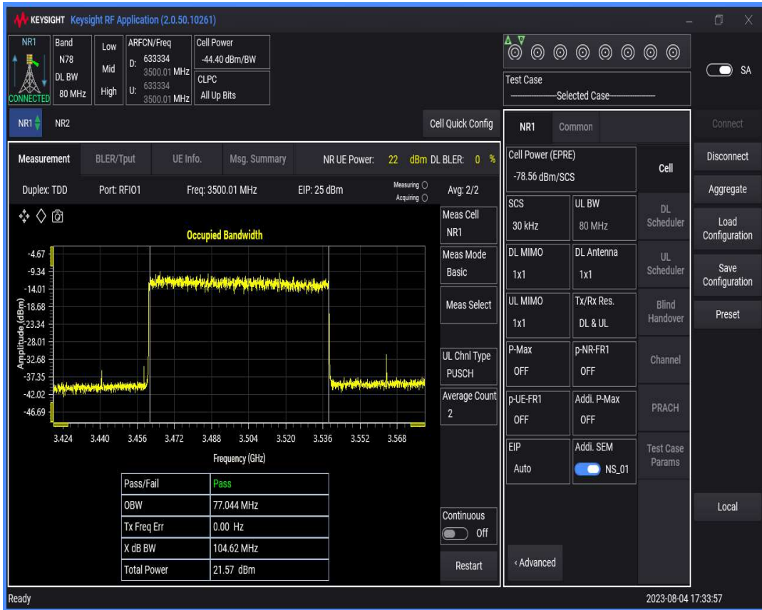
n78(3450-3550) SCS=30kHz DFT_QPSK BW=90MHz Channel=633334 RB=240@0
