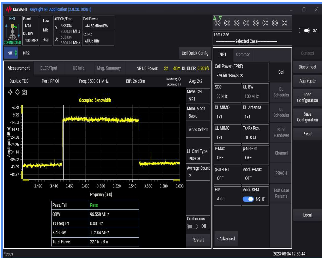
n78(3450-3550) SCS=30kHz DFT_QAM256 BW=10MHz Channel=633334 RB=24@0
