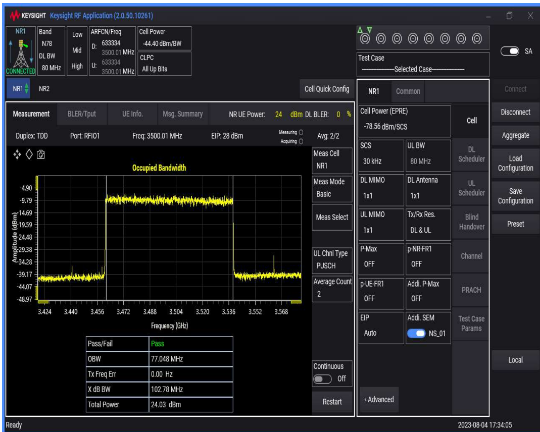
n78(3450-3550) SCS=30kHz DFT_QAM64 BW=90MHz Channel=633334 RB=240@0
