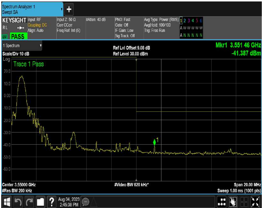
n78(3450-3550) SCS=30kHz CP_QPSK BW=10MHz Channel=636332 RB=1@23
