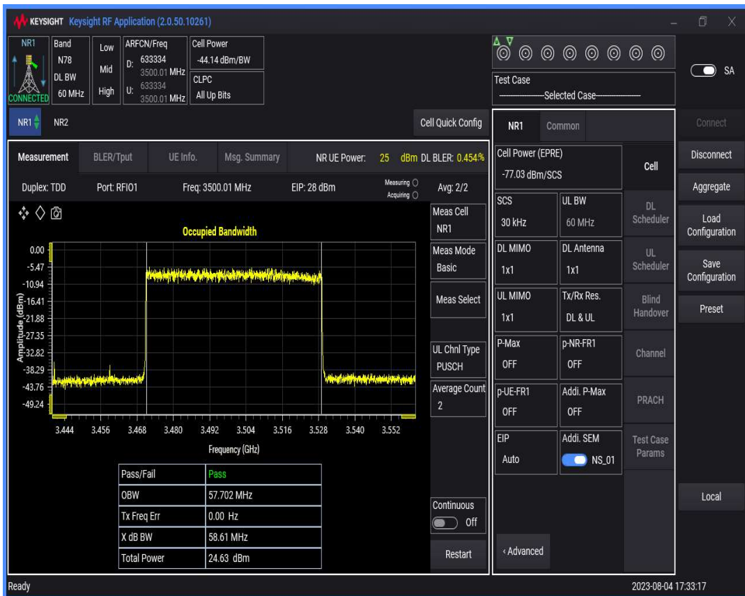
n78(3450-3550) SCS=30kHz DFT_QAM16 BW=70MHz Channel=633334 RB=
