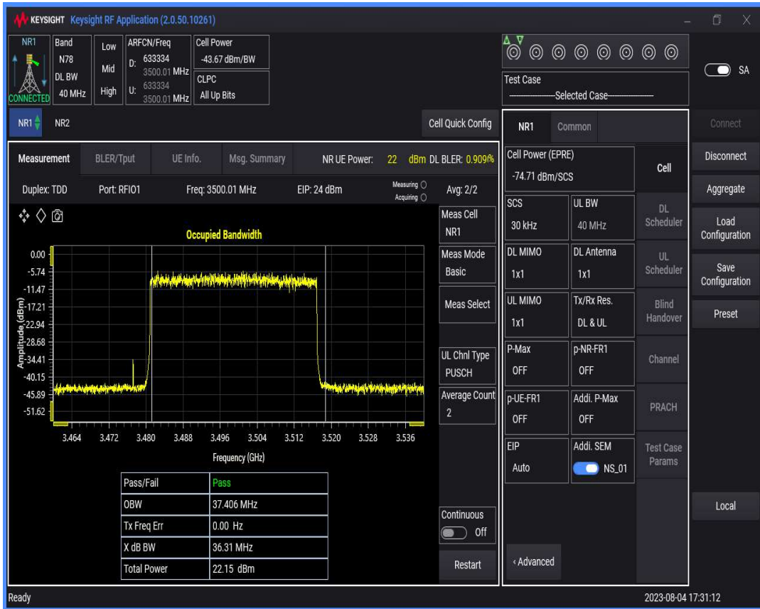
n78(3450-3550) SCS=30kHz DFT_QAM256 BW=50MHz Channel=633334 RB=128@0
