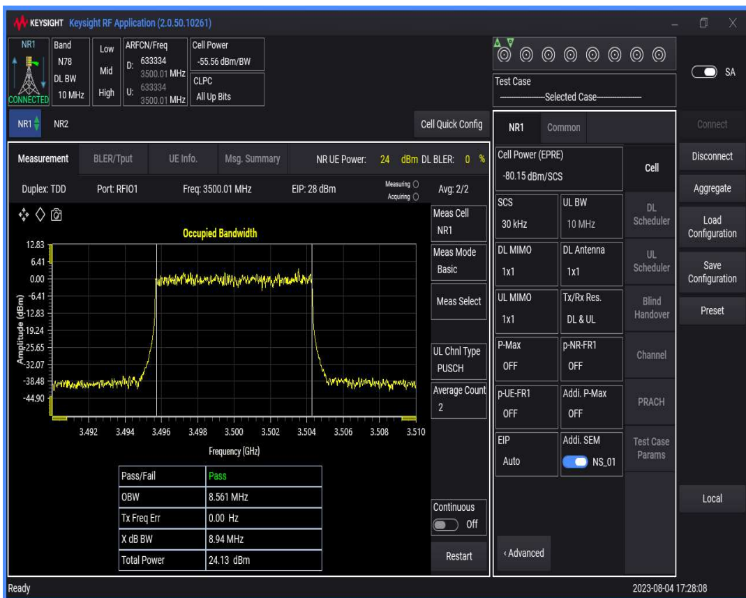
n78(3450-3550) SCS=30kHz DFT_QAM64 BW=15MHz Channel=633334 RB=36@0
