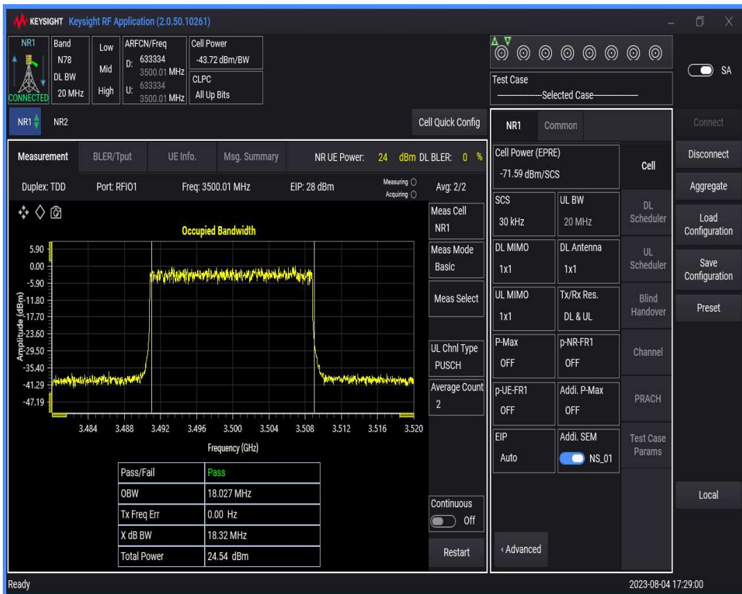
n78(3450-3550) SCS=30kHz DFT_QAM16 BW=30MHz Channel=633334 RB=75@0
