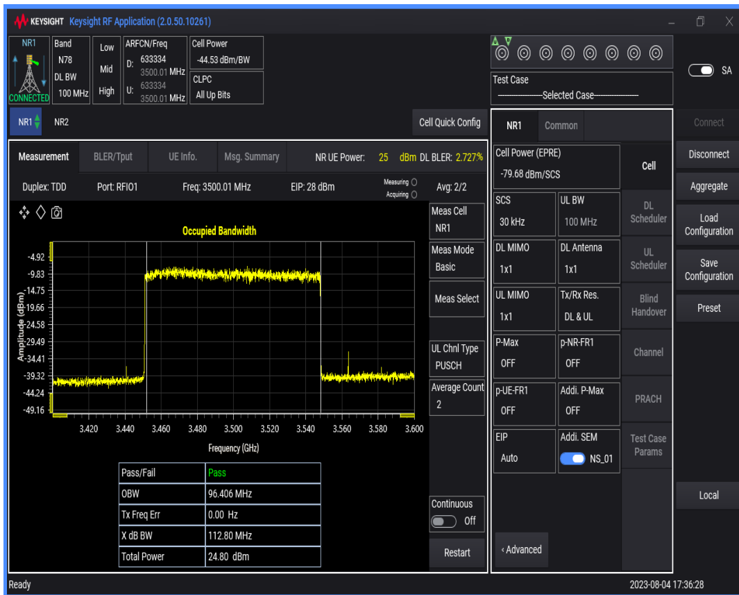
n78(3450-3550) SCS=30kHz DFT_BPSK BW=10MHz Channel=633334 RB=24@0
