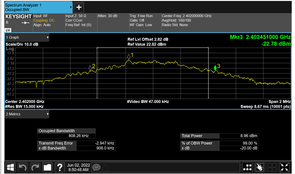
-20dB Bandwidth NVNT 1-DH1 2441MHz Ant1
