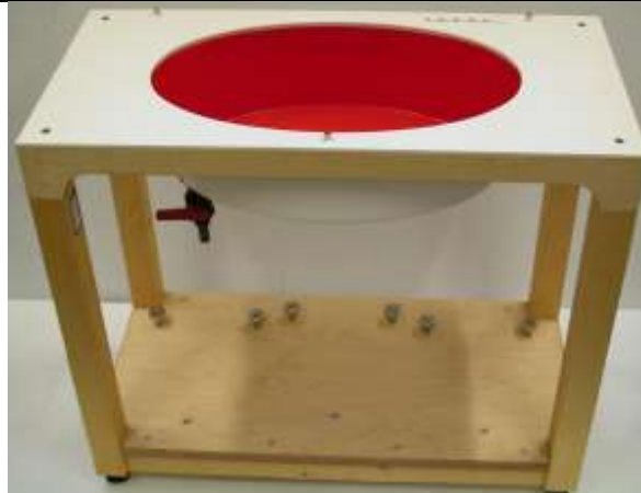
Fig.8.8 Photo of ELI4 Phantom
