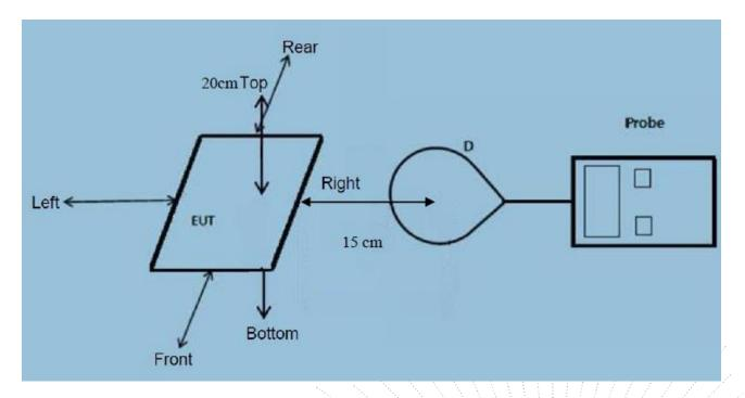
Note: Measurements should be made from all sides and the top of the primary/client pair, with the 15 cm measured from the center of the probe(s) to the edge of the device
