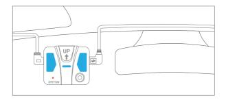
Finally, connect the power cable to the dash cam.
