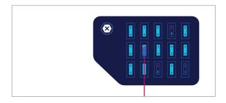
Find the switched fuse and connect the RED cable to it. This fuse has power only when the  $\mbox{car}$  is on.
