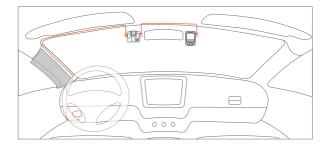
Run the wiring towards the fuse box with the included smart hardwire kit.
