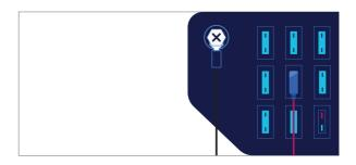
Attach the black fuse cable. Make sure to attached the GROUND cable to the bolt near the fuse box.
