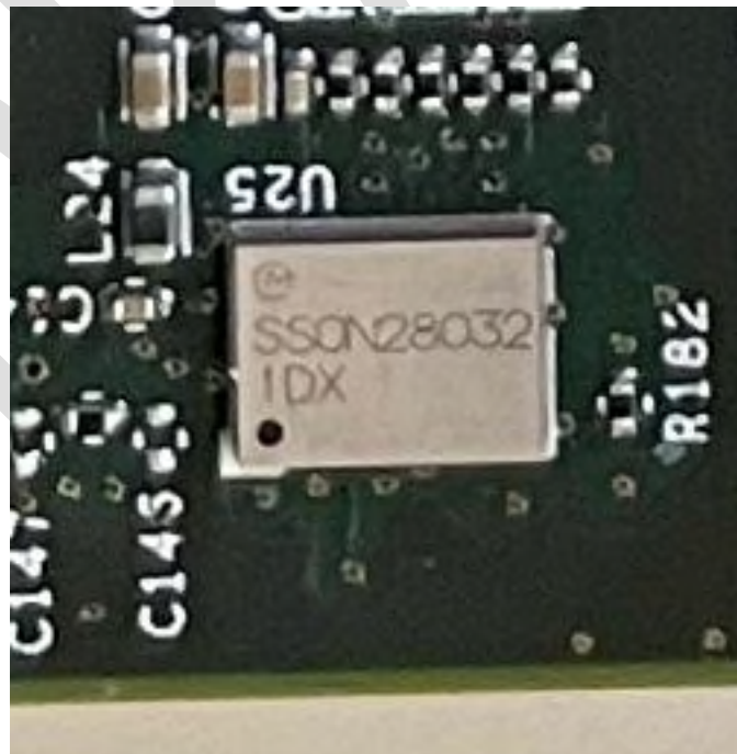
Figure 3 - Wi-Fi/Bluetooth module (detail)
