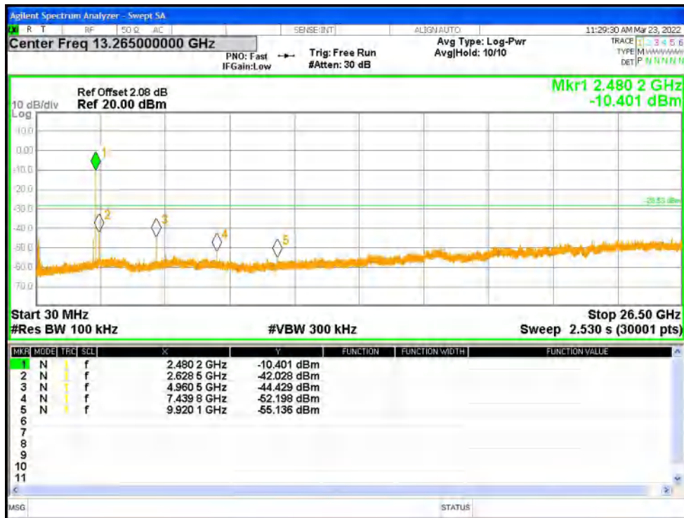
Tx. Spurious NVNT 3-DH1 2402MHz Ant1 Ref
