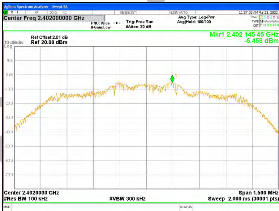
Tx. Spurious NVNT 3-DH1 2402MHz Ant1 Emission
