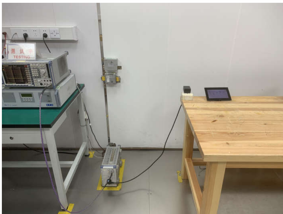
Conducted Emissions Test Setup
