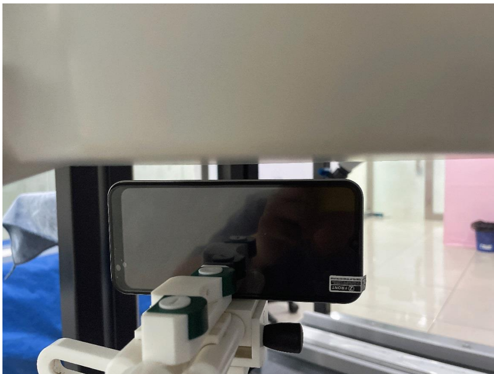
Body Left side(separation distance is 10mm)
