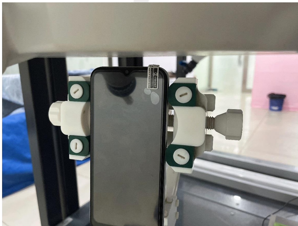
Body Top side(separation distance is 10mm)
