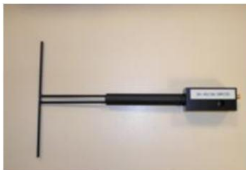
Figure 1 – Satimo COMOSAR Validation Dipole
