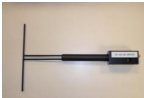
Figure 1 – Satimo COMOSAR Validation Dipole
