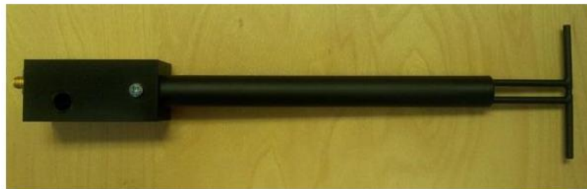
Figure 1 – MVG COMOSAR Validation Dipole
