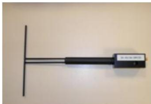
Figure 1 – Satimo COMOSAR Validation Dipole
