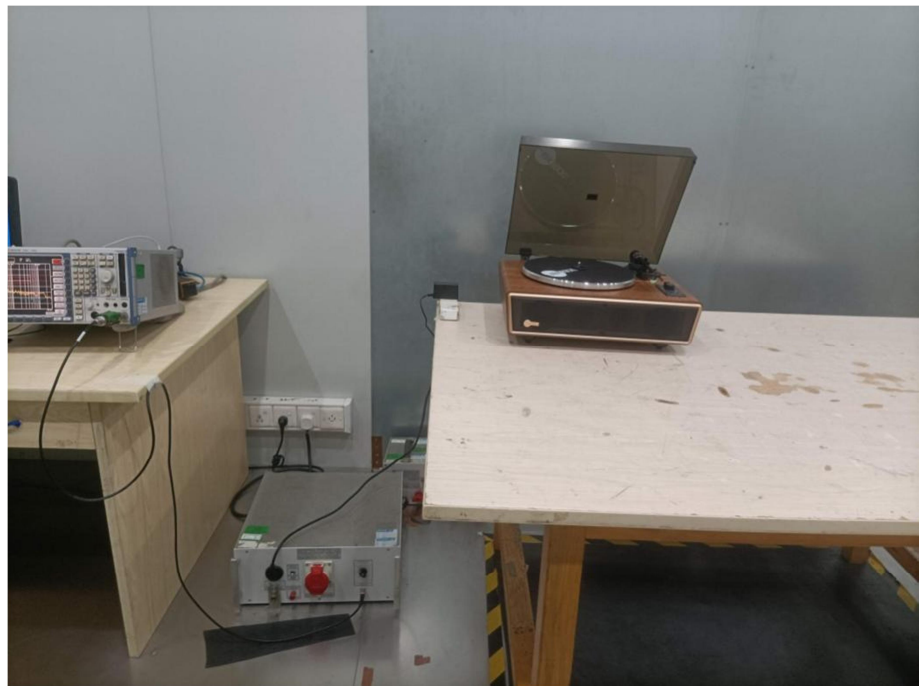
Conducted Emission Test Setup
