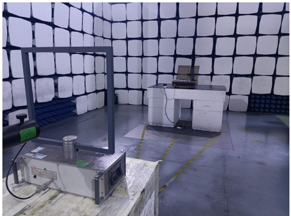
Radiation Emission Test Setup (Below 30MHz)
