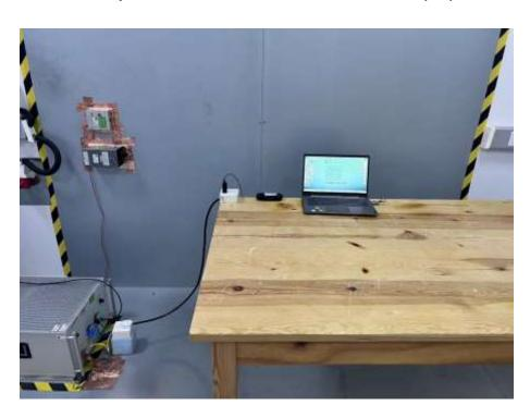
Set-up for Radiated Emission (RE), Below 1GHz
