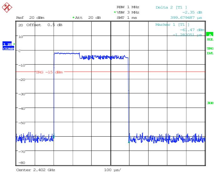
**EDR ( $\pi/4$ -DQPSK):Pulse time, Middle Channel, 2DH1**
