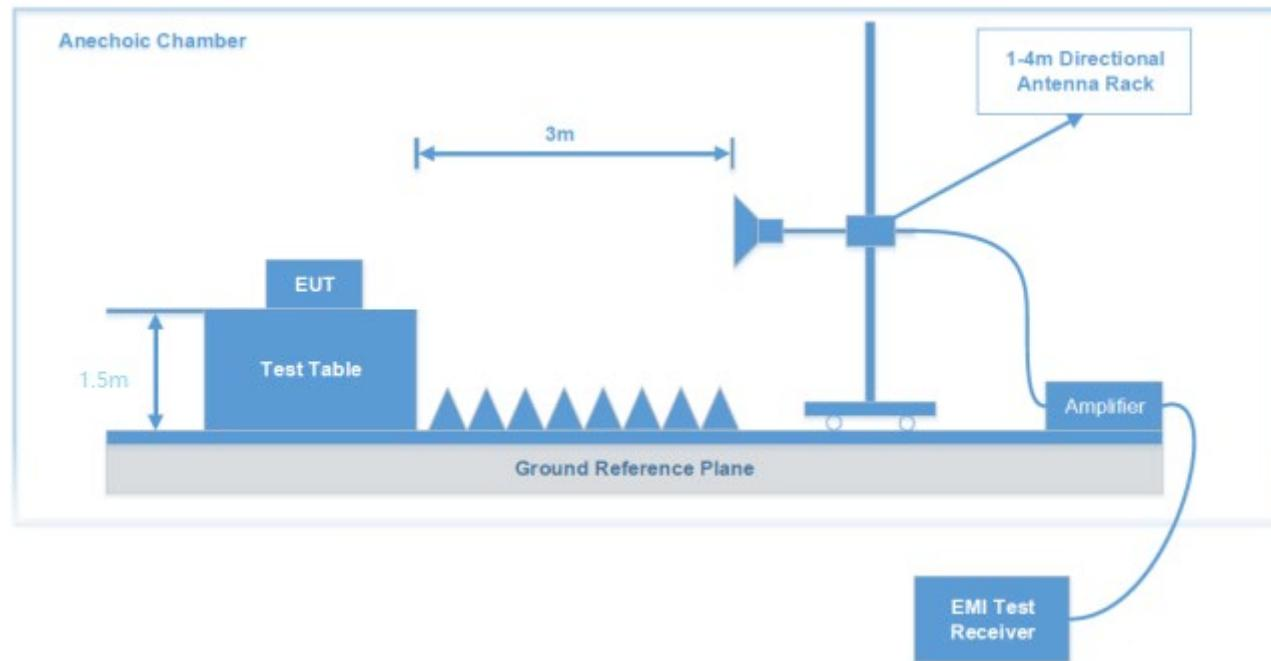
The radiated emission tests were performed in the 3 meters, using the setup accordance with the ANSI C63.10-2020. The specification used was the FCC 15.209 and FCC 15.247 limits.
