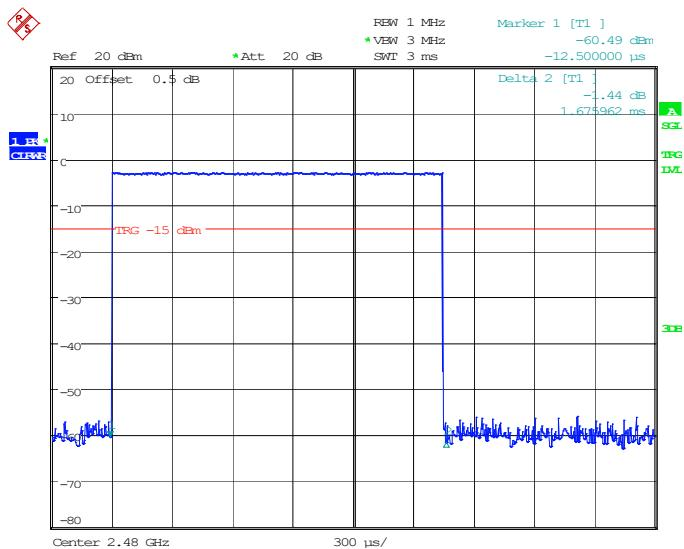
**BDR (GFSK): Pulse time, Low Channel, DH5**
