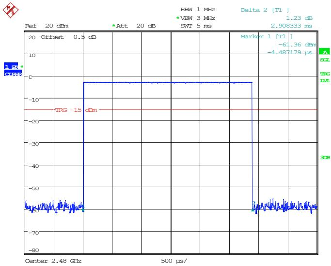
**EDR ( $\pi/4$ -DQPSK): Pulse time, Low Channel, 2DH1**
