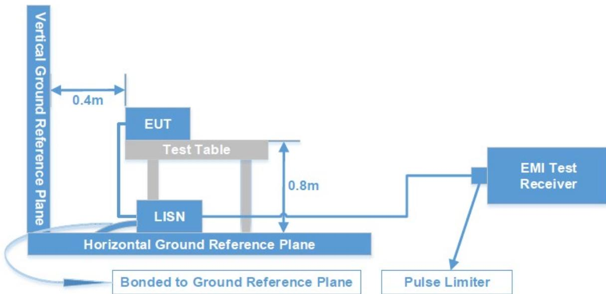
The measurement procedure of EUT setup is according with ANSI C63.10-2020. The related limit was specified in FCC Part 15.207.
