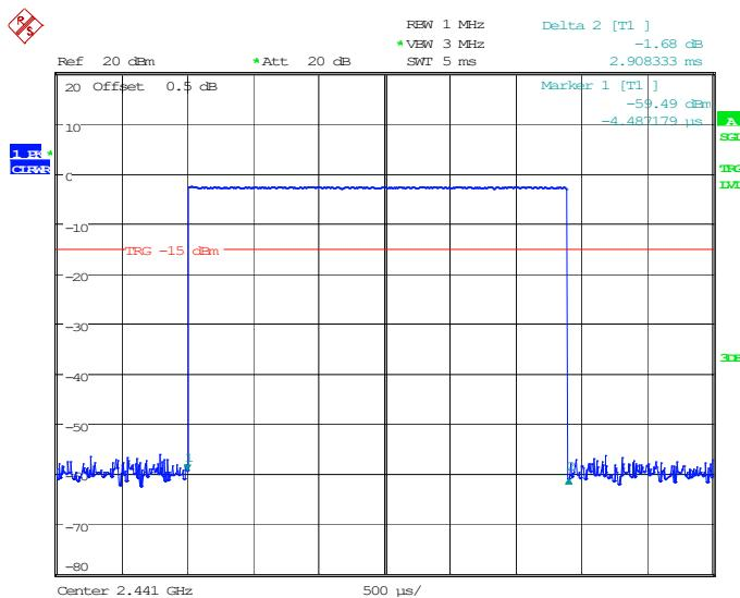
**BDR (GFSK): Pulse time, High Channel, DH5**
