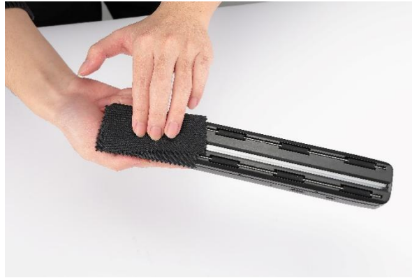
Figure 3- 1 Clean The CIS
