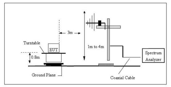
(C) Radiated Emission Test-Up Frequency Above 1GHz
