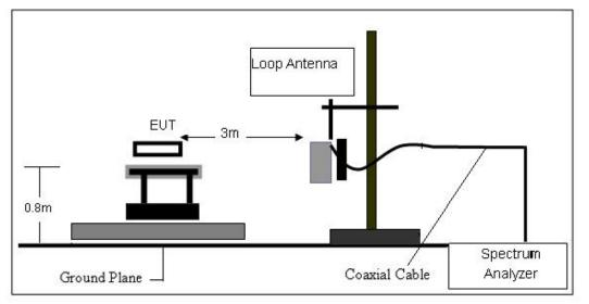
(B) Radiated Emission Test-Up Frequency 30MHz~1GHz
