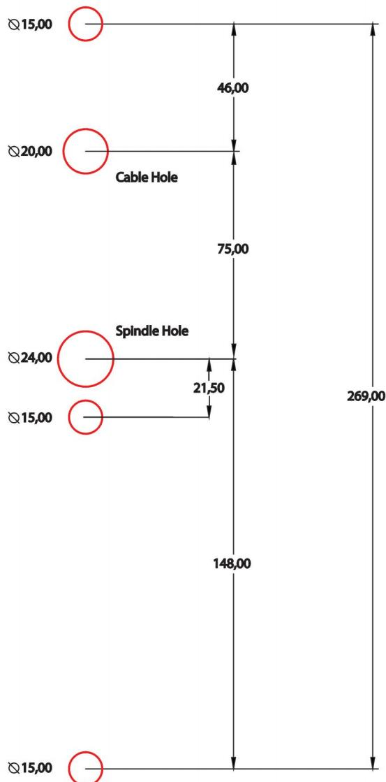
Location of drilling on the door is usually 1 meter from ground to the lever handle. The back set is determined by the chosen lock
