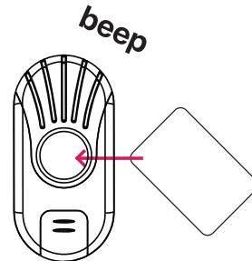
If the RFID credential is valid when presented to the front panel it will sound a "beep" and activate the motor so the lever can be rotated downwards and in turn retracts the latch. The lock will also display a blue LED. Invalid credentials will show a red LED and blink a number of times, it is important to count the quantity of red blinks as this helps to diagnose the reason why access was rejected.
