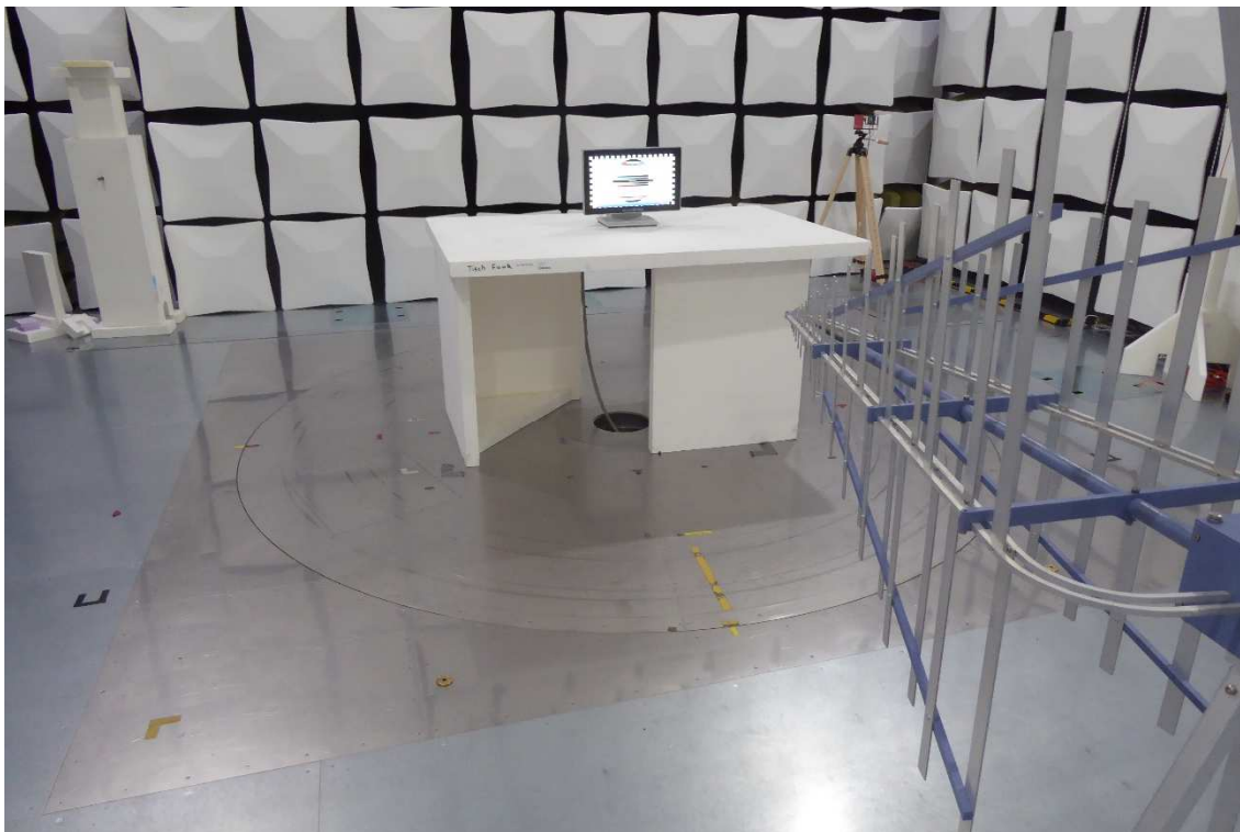
Test setup 1: Radiated Emission/Turntable position 0
