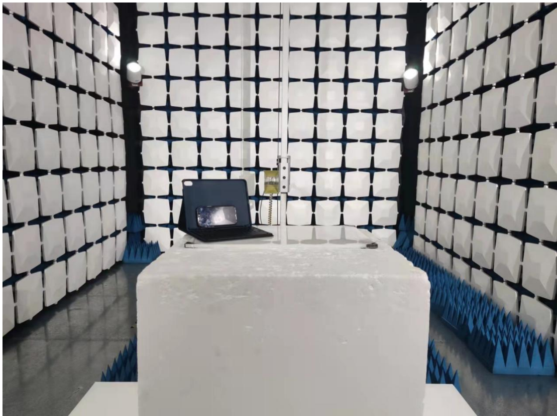
Above 1GHz for radiated emission test setup
