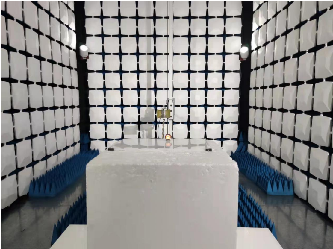
Above 1GHz for radiated emission test setup
