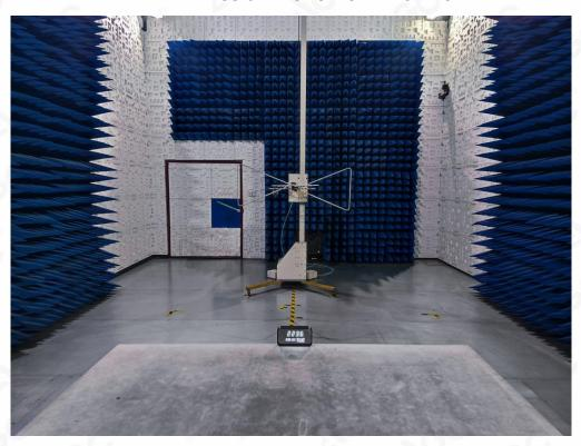
RADIATED EMISSION TEST SETUP ABOVE 1GHz
