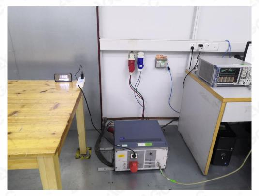
RF CONDUCTED TEST SETUP
