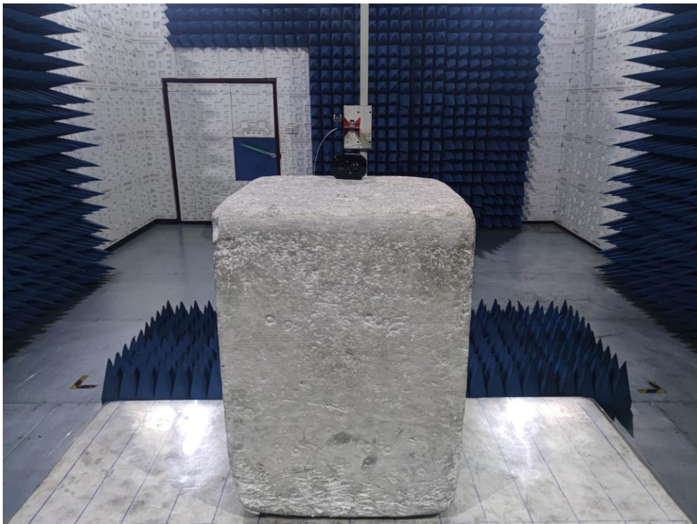
RADIATED EMISSION TEST SETUP ABOVE 1GHz
