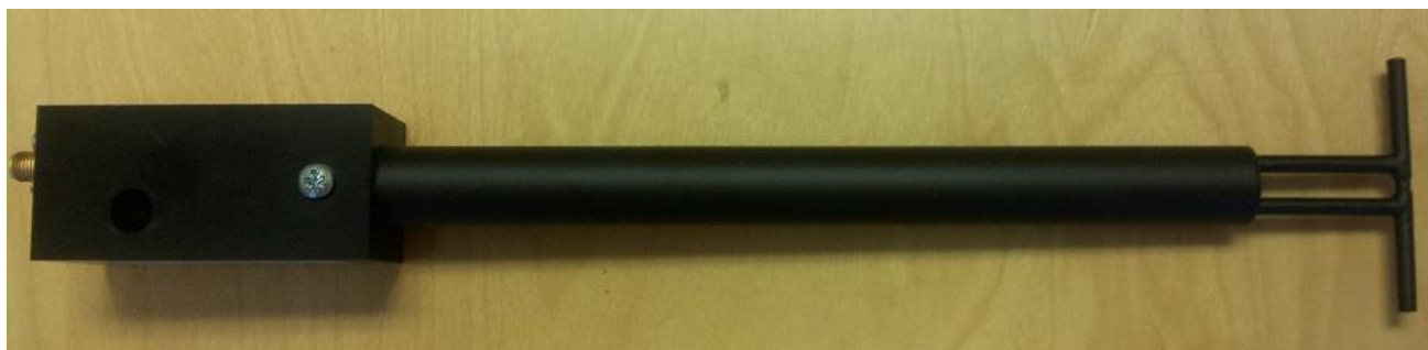
Figure 1 – MVG COMOSAR Validation Dipole
