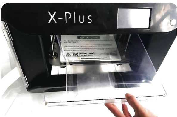
11. Open the front door and take out the 3d printer's top cover .
