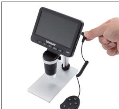
4. Attach the wired remote into the 3.5 mm jack.
