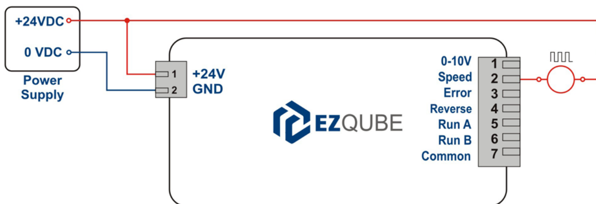
Figure 14 – SpeedOut NPN module wiring
