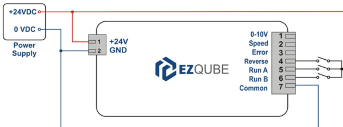
Figure 17 - PNP module wiring with Common connection
