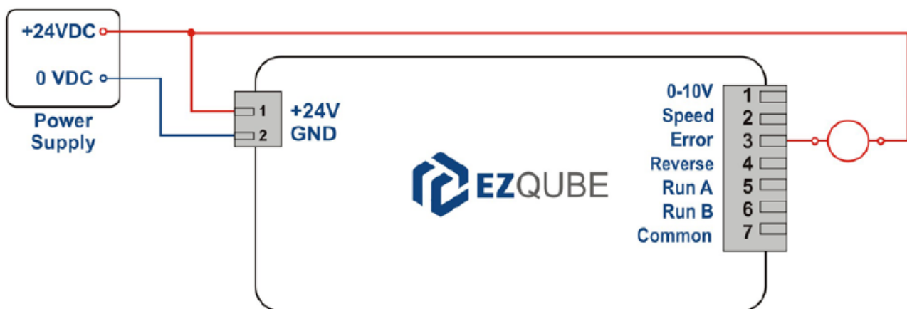
Figure 16 – ErrorOut NPN module wiring
