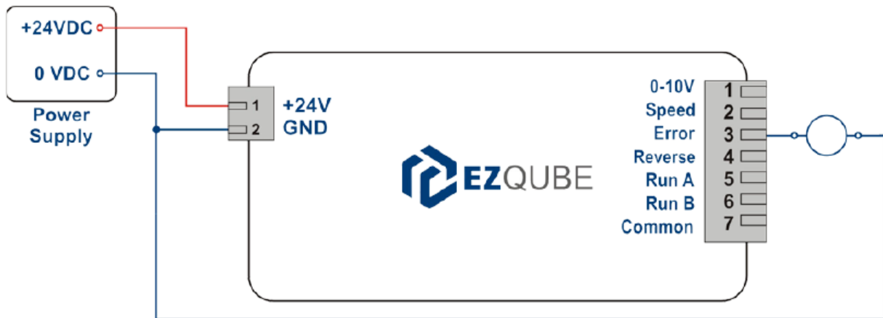
Figure 15 – ErrorOut PNP module wiring
