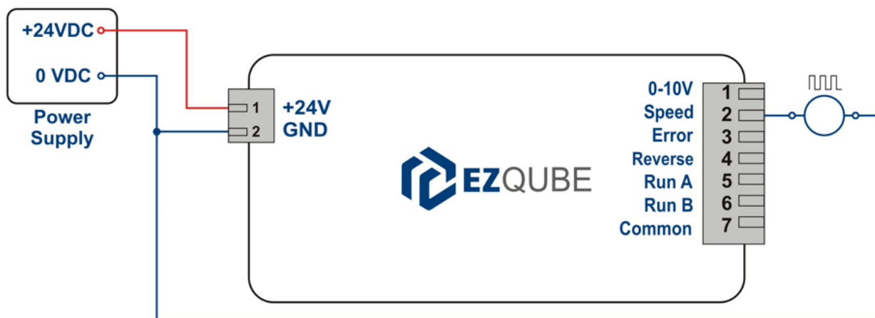
Figure 13 – SpeedOut PNP module wiring
