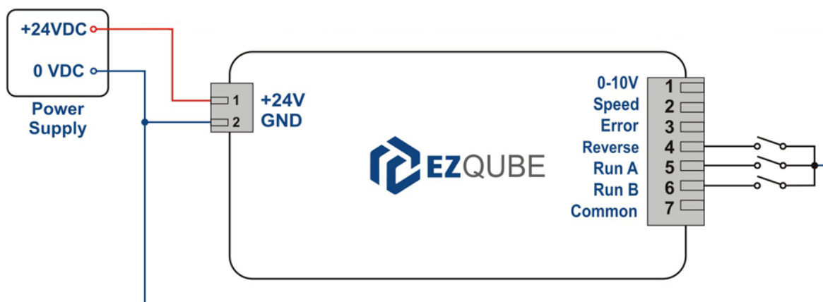
Figure 20 - NPN module wiring without Common connection
