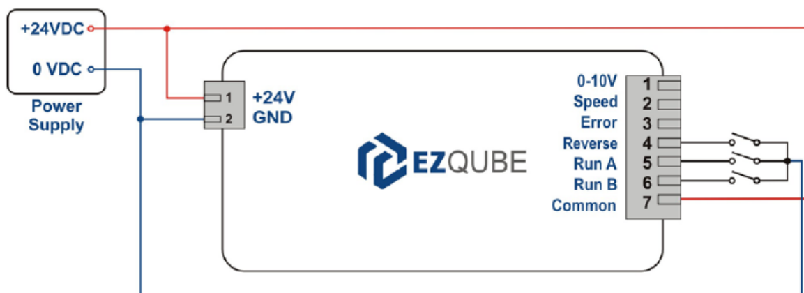
Figure 19 - NPN module wiring with Common connection
