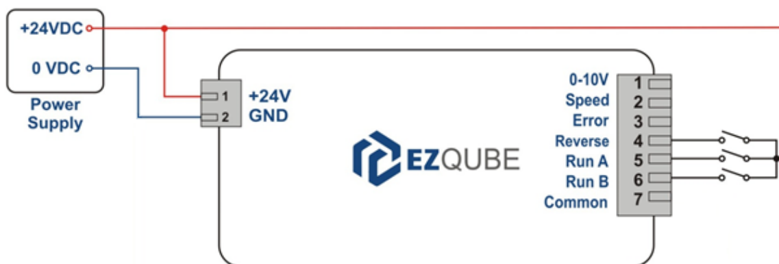
Figure 18 - PNP module wiring without Common connection
