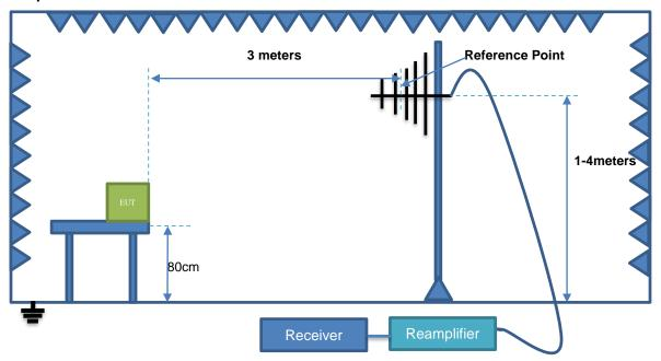
Radiation Test (30MHz - 1GHz)
