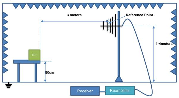
Radiation Test (30MHz - 1GHz)
