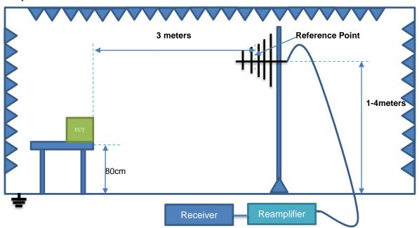
Radiation Test (30MHz - 1GHz)
