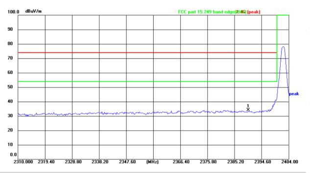
Site Polarization: Vertical Temperature: 24(℃) Limit: FCC part 15.249 band edge 2.4G (peak) DC 3.7 V Power: Humidity: 52 % Frequency Reading Factor Limit Margin Detector P/F Remark No. (MHz) (dB/m) (dBuV) (dBuV/m)(dBuV/m)(dB)
