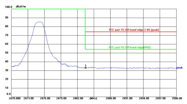
Site Polarization: Horizontal Temperature: 24(°C) Limit: FCC part 15.249 band edge 2.4G (peak) Power: DC 3.7 V Humidity: 52 %
