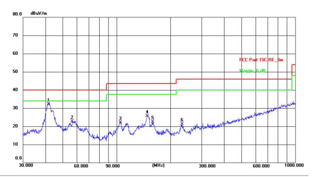
Site #2 3m Anechoic Chamber Polarization: Vertical Temperature: 24.8(C) Humidity: 49 %
