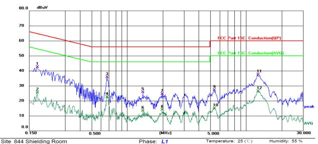
Limit: FCC Part 15C Conduction(QP)
