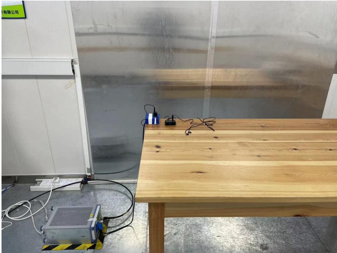
Conducted emission test setup
