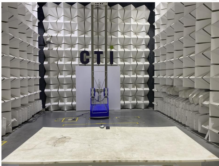
Radiated Spurious Emissions Test Setup (30MHz~1GHz)
