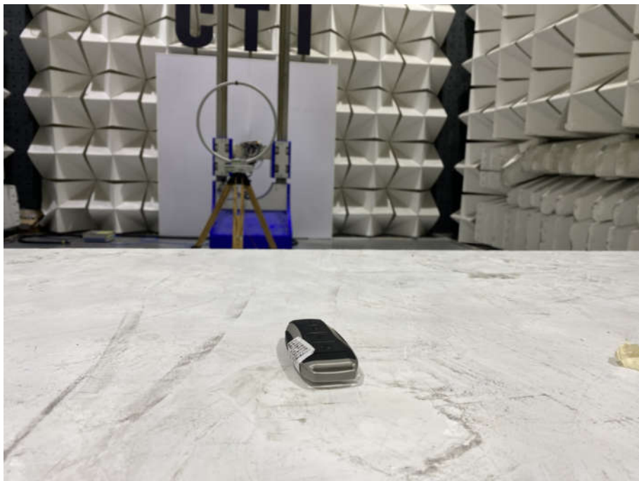
Radiated emission Test Setup-2(9kHz~30MHz)close up photo
