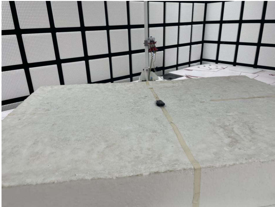
Radiated spurious emission Test Setup-3(Above 1GHz)
