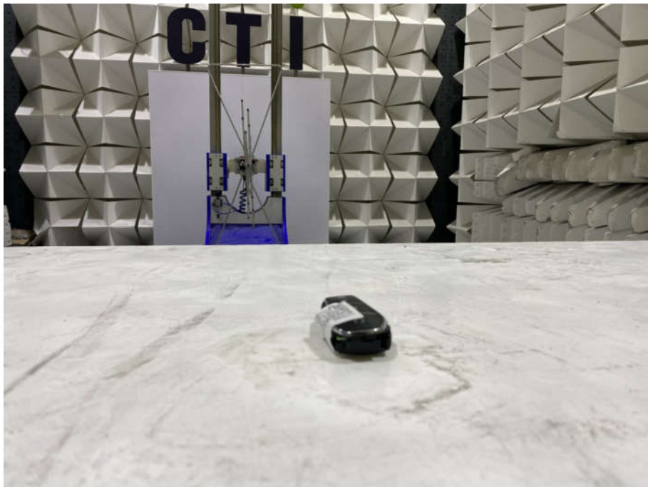
Radiated emission Test Setup-4(30MHz~1GHz)close up photo
