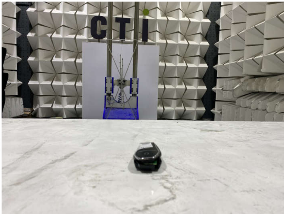
Radiated emission Test Setup-4(30MHz~1GHz)close up photo
