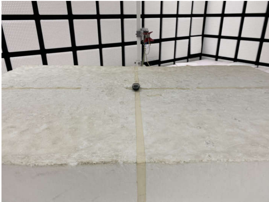
Radiated spurious emission Test Setup-3(Above 1GHz)
