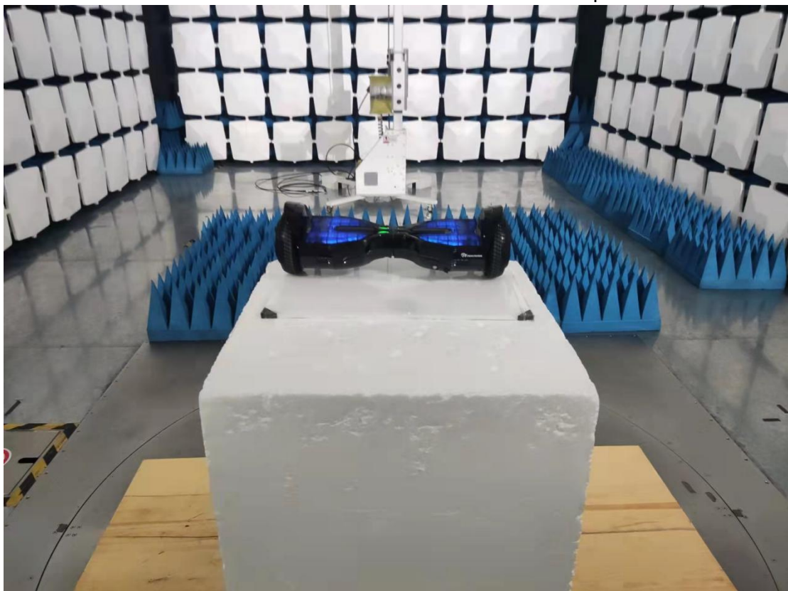
Above 1GHz for radiated emission test setup
