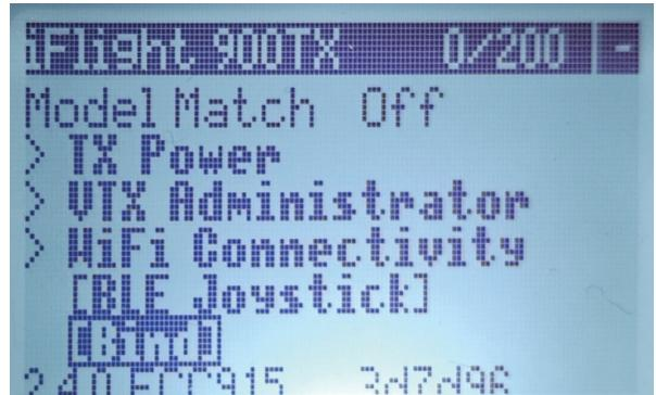
Hold down System Setings to go to the TOOLS screen, move the cursor to the ExpressLRS option, and hold down Enter to go to the next option
