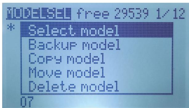
▲ Move to a model you have set up then press and hold the right 5-Axis button (Enter).
