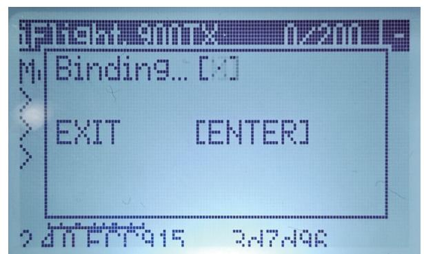
▲ 6. Binding screen appears. The blue LED on the receiver will turn to solid blue. Bind was successful.
