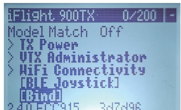
▲ 5. Scroll down to Bind, press the right 5-Axis button to enter. BIND mode active.
