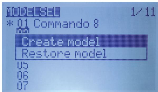
▲ Move to a free entry then press and hold the right 5-Axis button (Enter).
