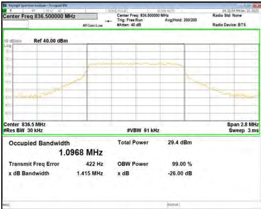
Band5 QPSK BW=1.4MHz Channel=20643 RB Size=6 Position=#0
