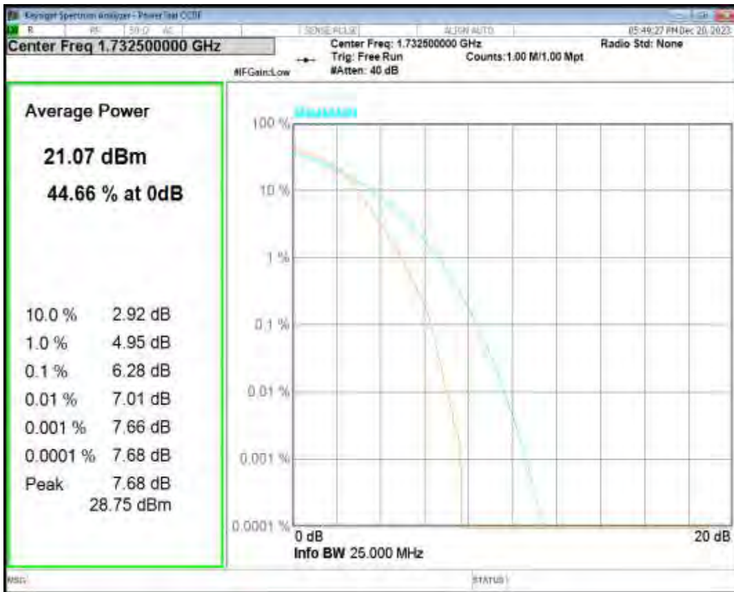
Band4 QPSK BW=3MHz Channel=20175 RB Size=1 Position=#0
