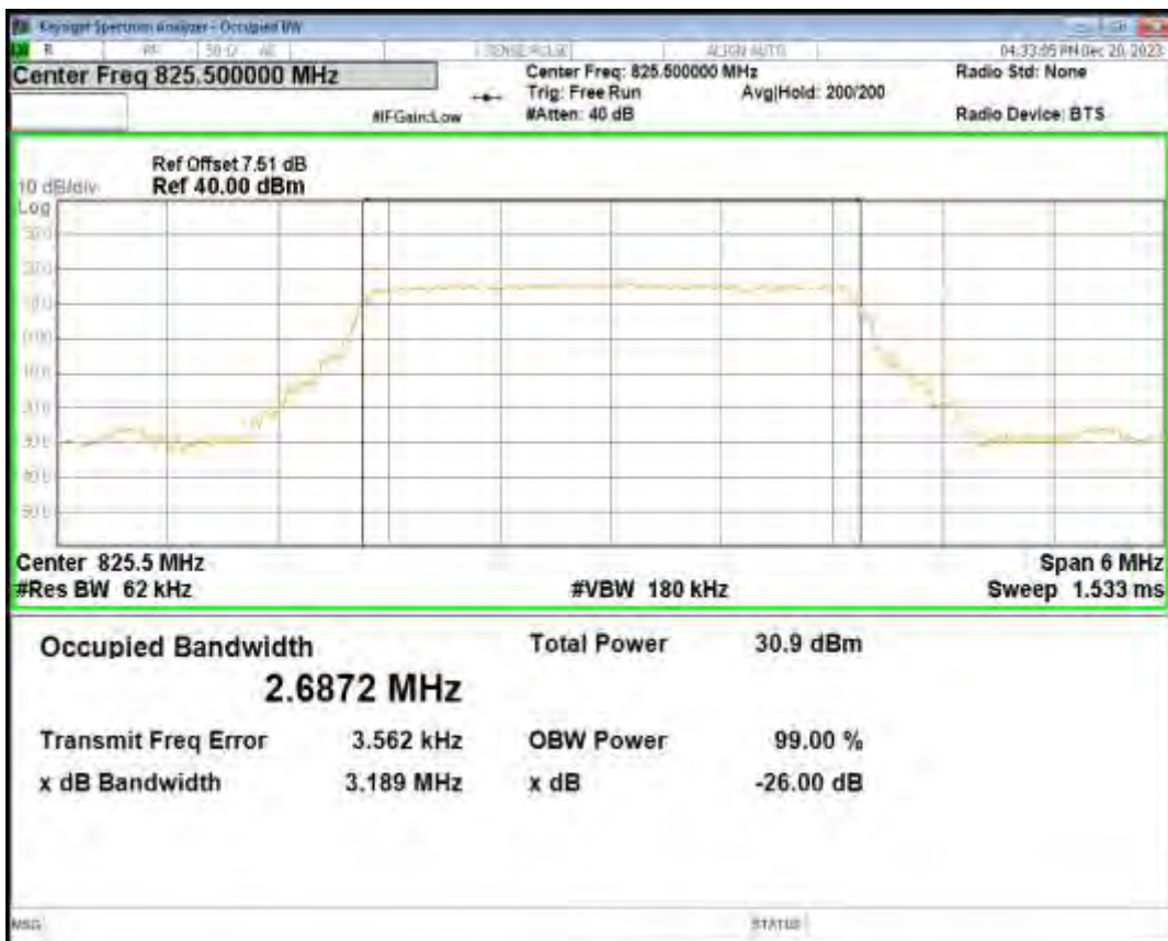
Band5 16QAM BW=3MHz Channel=20415 RB Size=15 Position=#0
