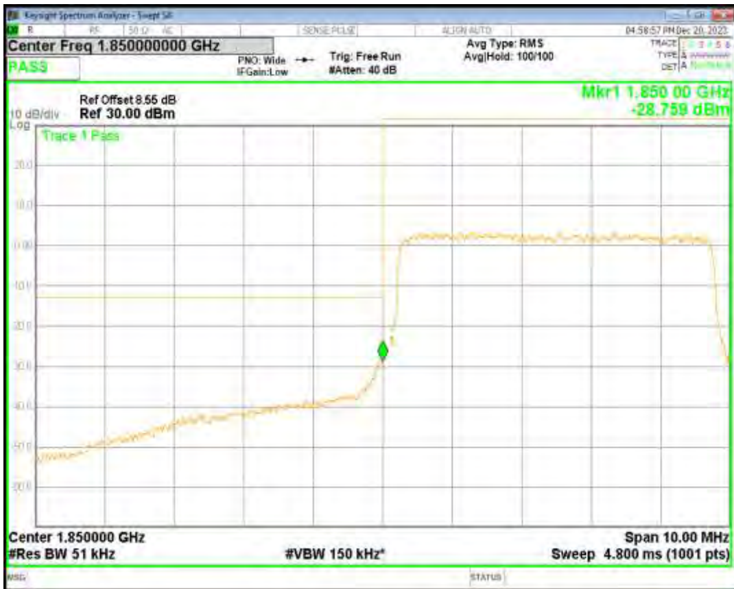
Band2 16QAM BW=5MHz Channel=18625 RB Size=25 Position=#0
