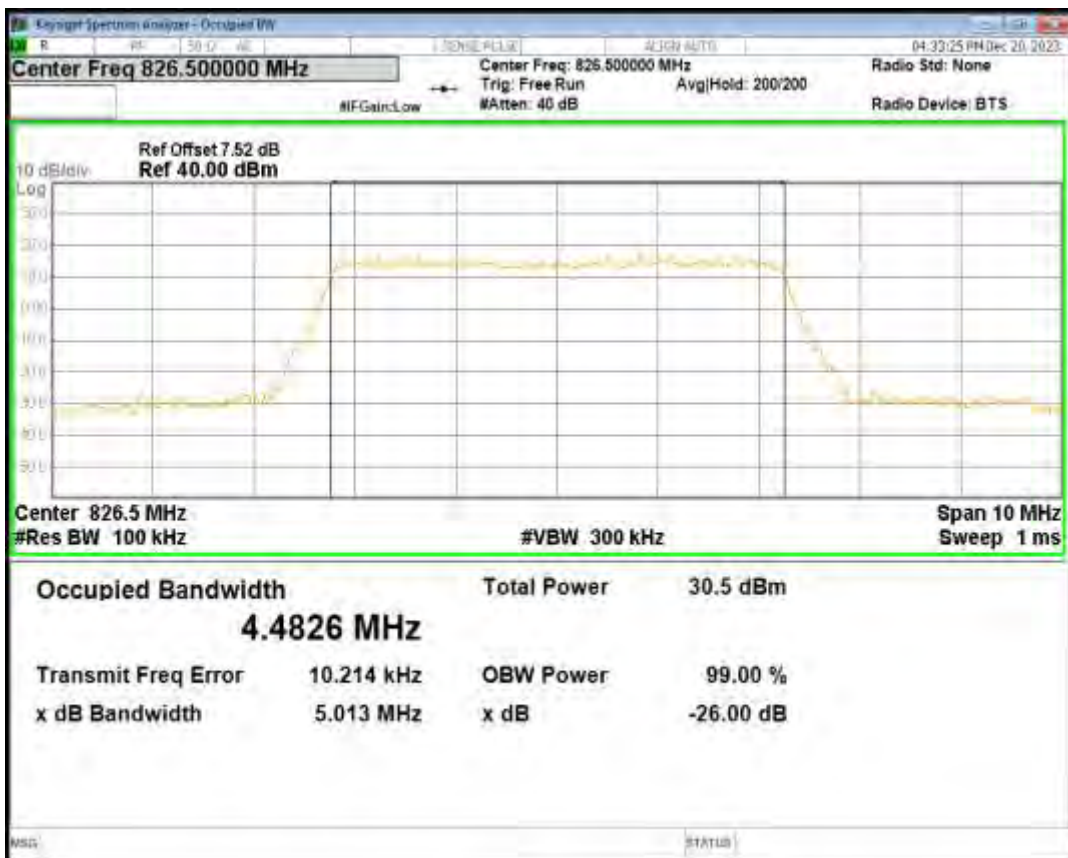
Band5 16QAM BW=5MHz Channel=20425 RB Size=25 Position=#0
