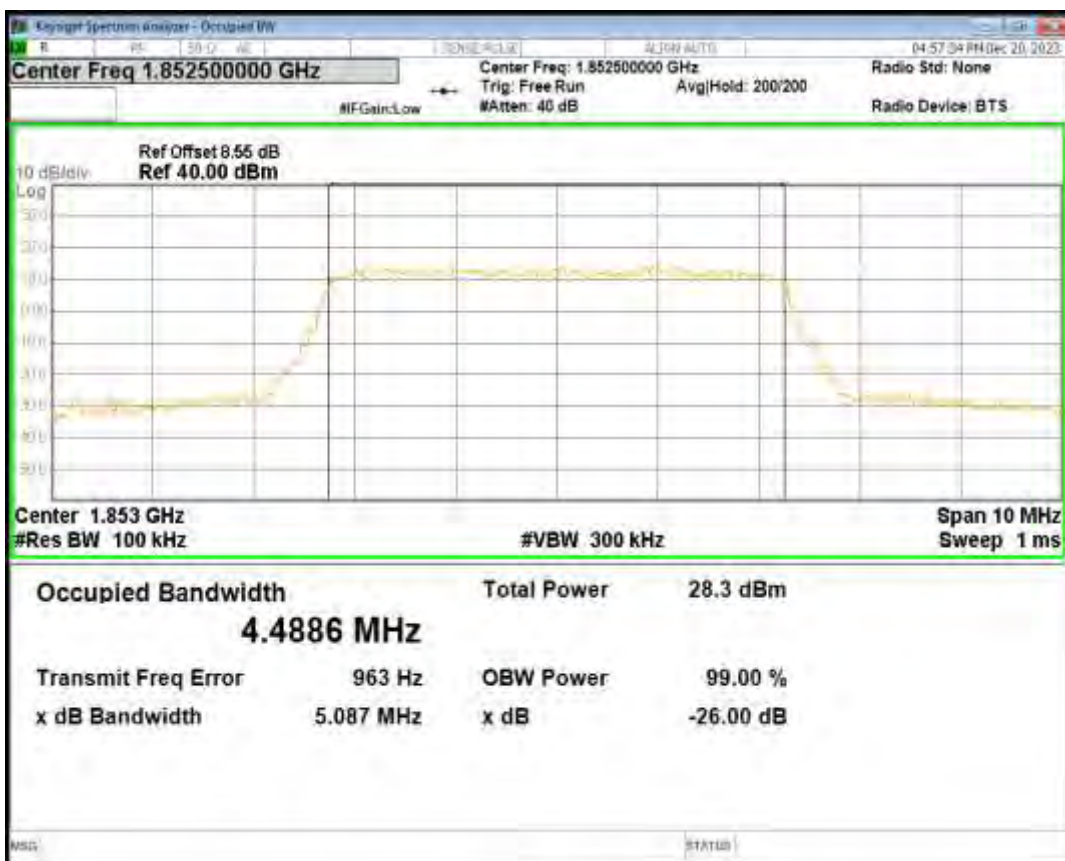
Band2 QPSK BW=5MHz Channel=18900 RB Size=25 Position=#0
