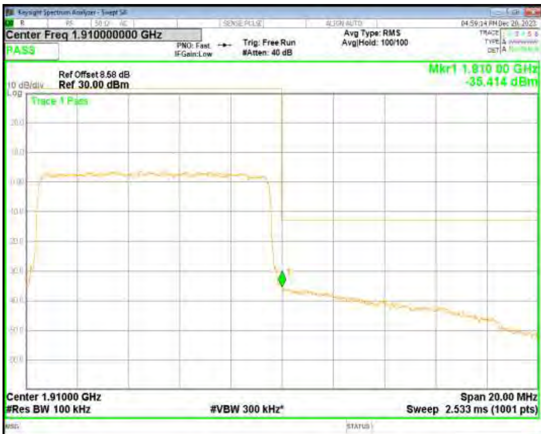
Band2 QPSK BW=15MHz Channel=18675 RB Size=75 Position=#0
