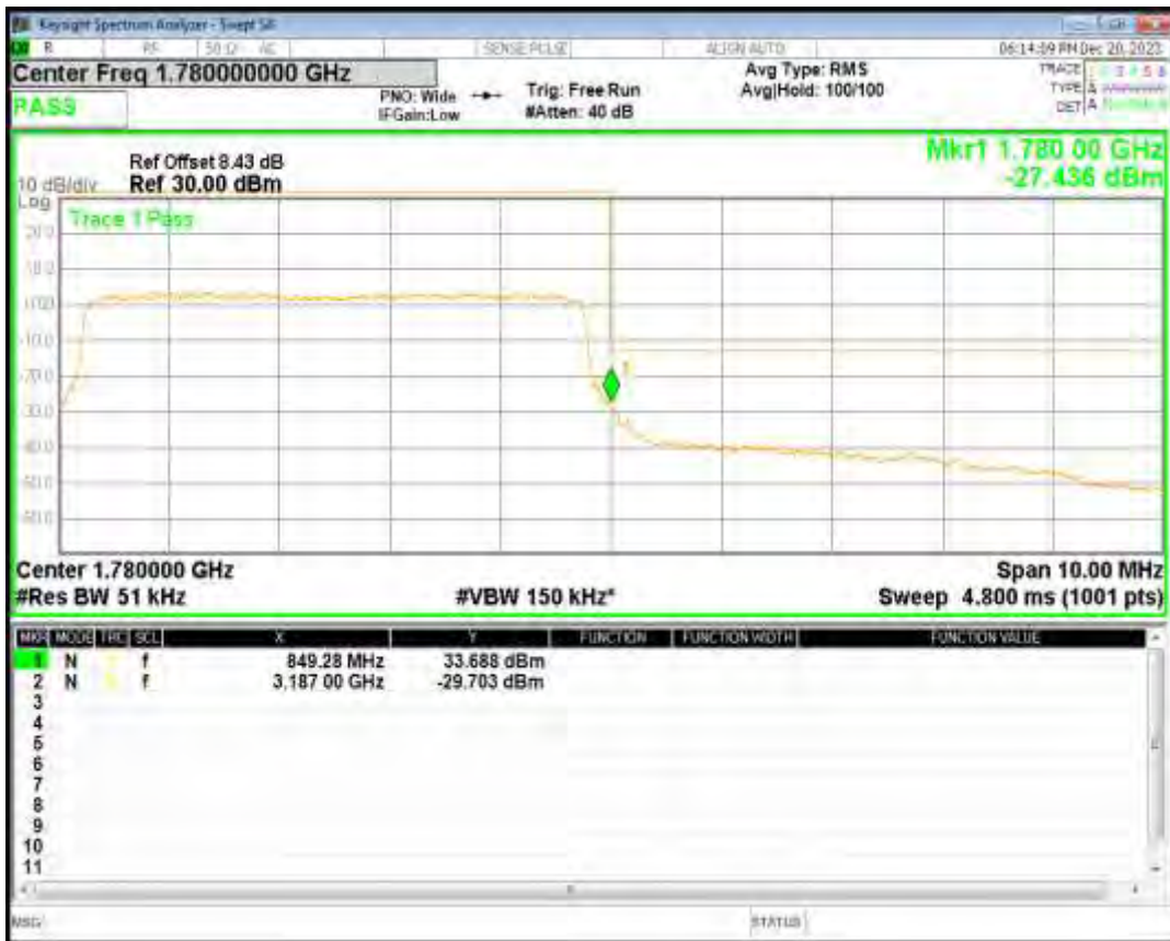
Band66 16QAM BW=5MHz Channel=132647 RB Size=25 Position=#0
