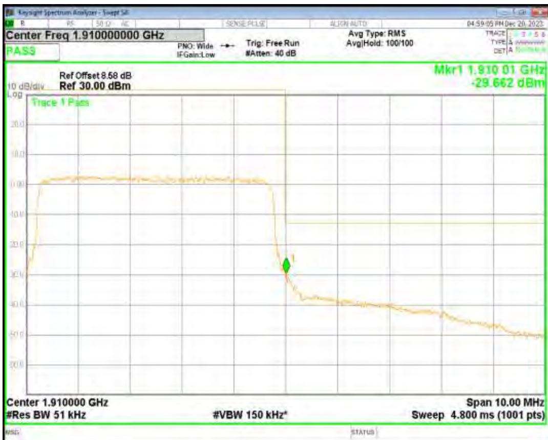
Band2 QPSK BW=10MHz Channel=18650 RB Size=50 Position=#0
