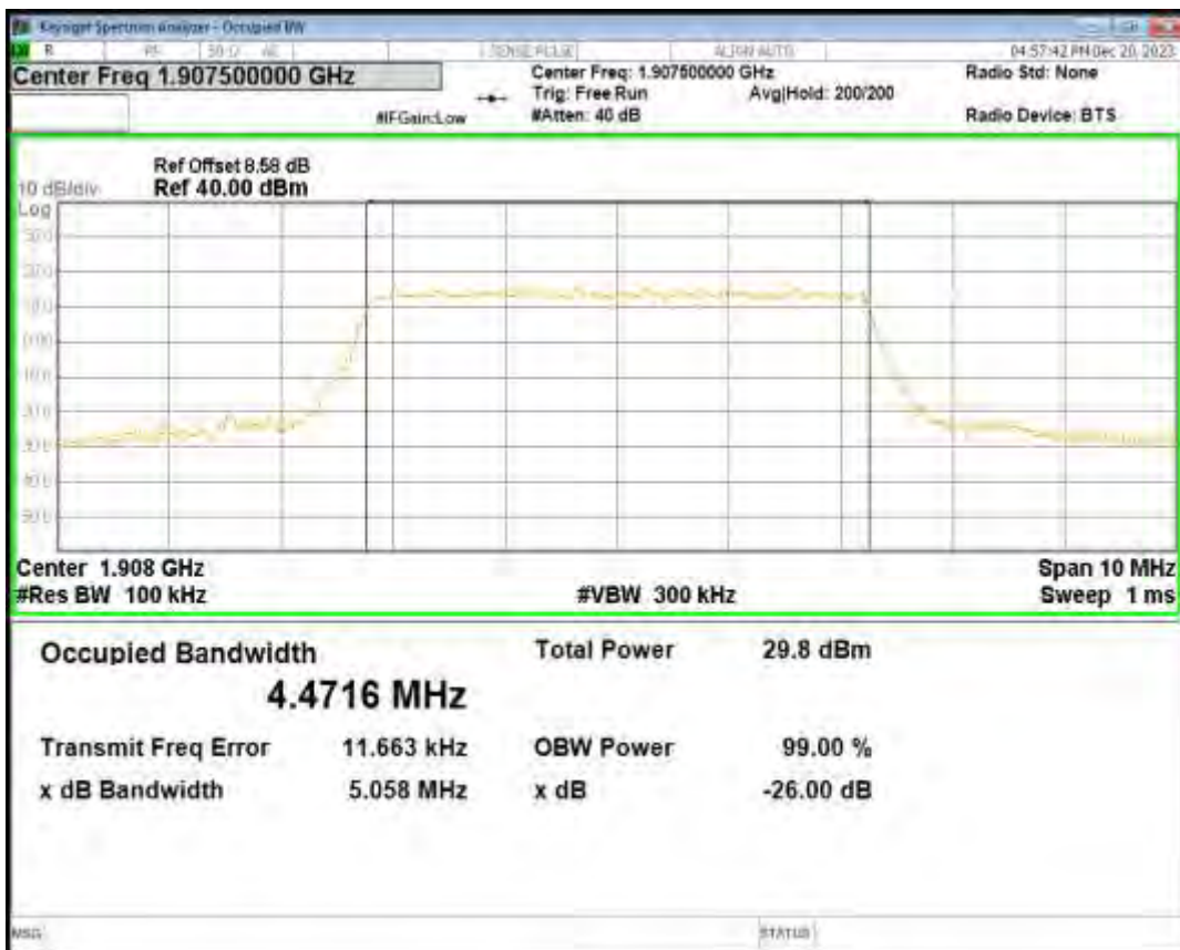
Band2 16QAM BW=5MHz Channel=19175 RB Size=25 Position=#0
