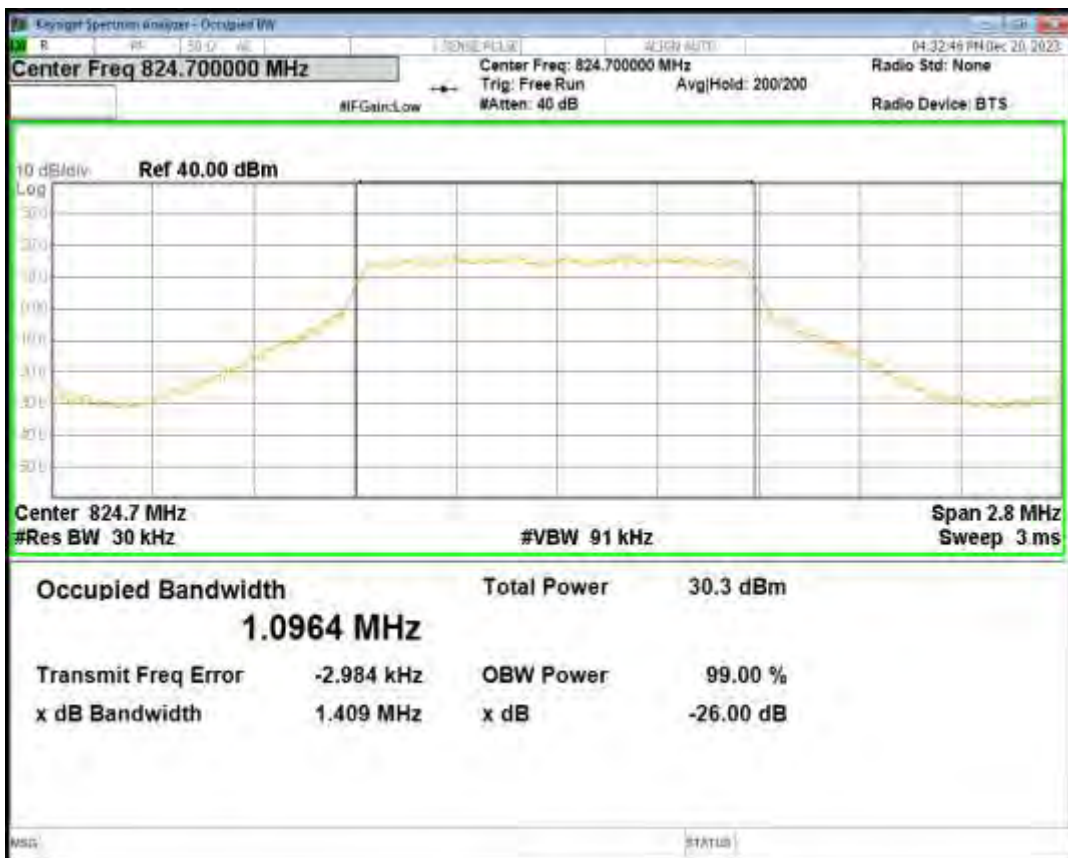
Band5 16QAM BW=1.4MHz Channel=20407 RB Size=6 Position=#0
