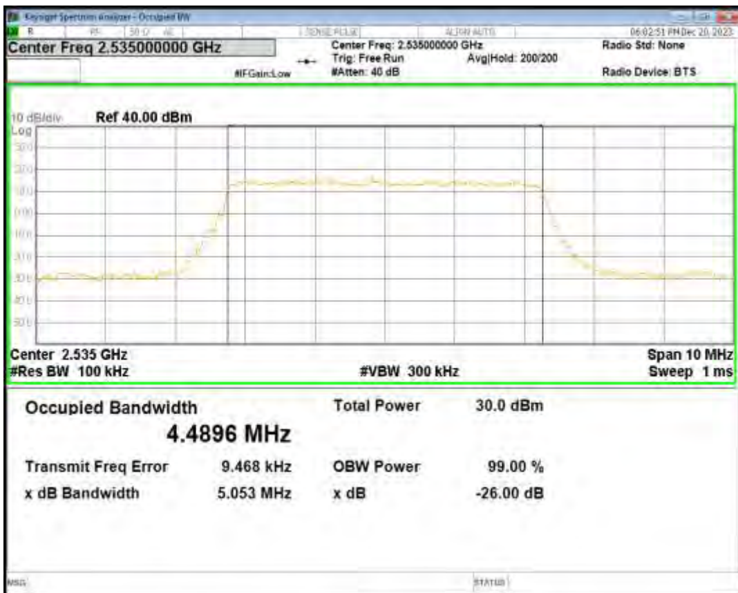
Band7 16QAM BW=5MHz Channel=21100 RB Size=25 Position=#0
