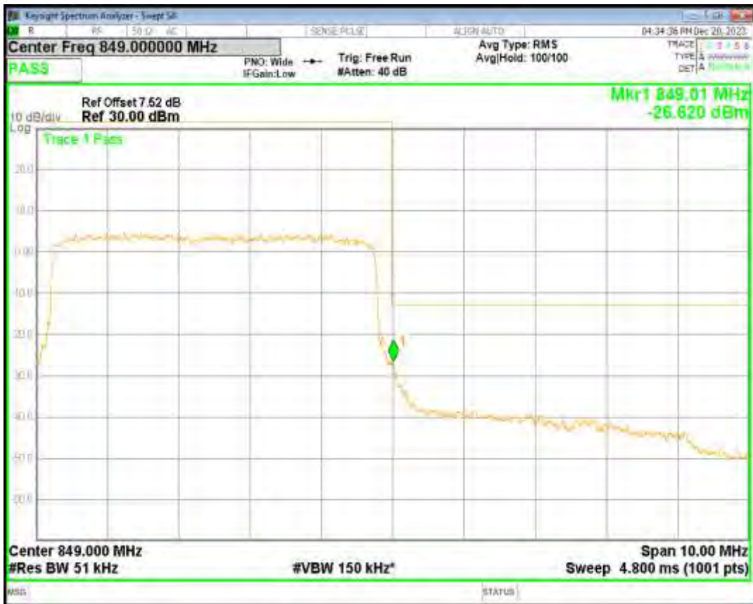
Band5 16QAM BW=5MHz Channel=20625 RB Size=25 Position=#0
