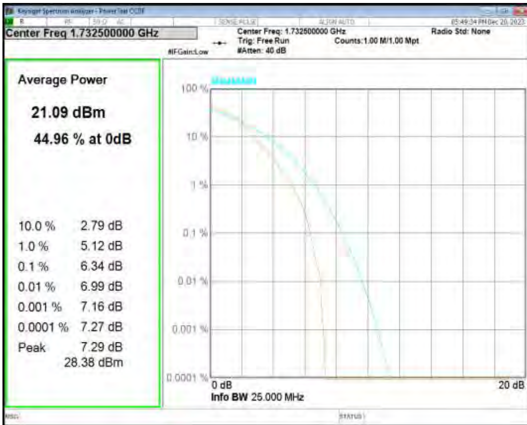
Band4 QPSK BW=5MHz Channel=20175 RB Size=1 Position=#0
