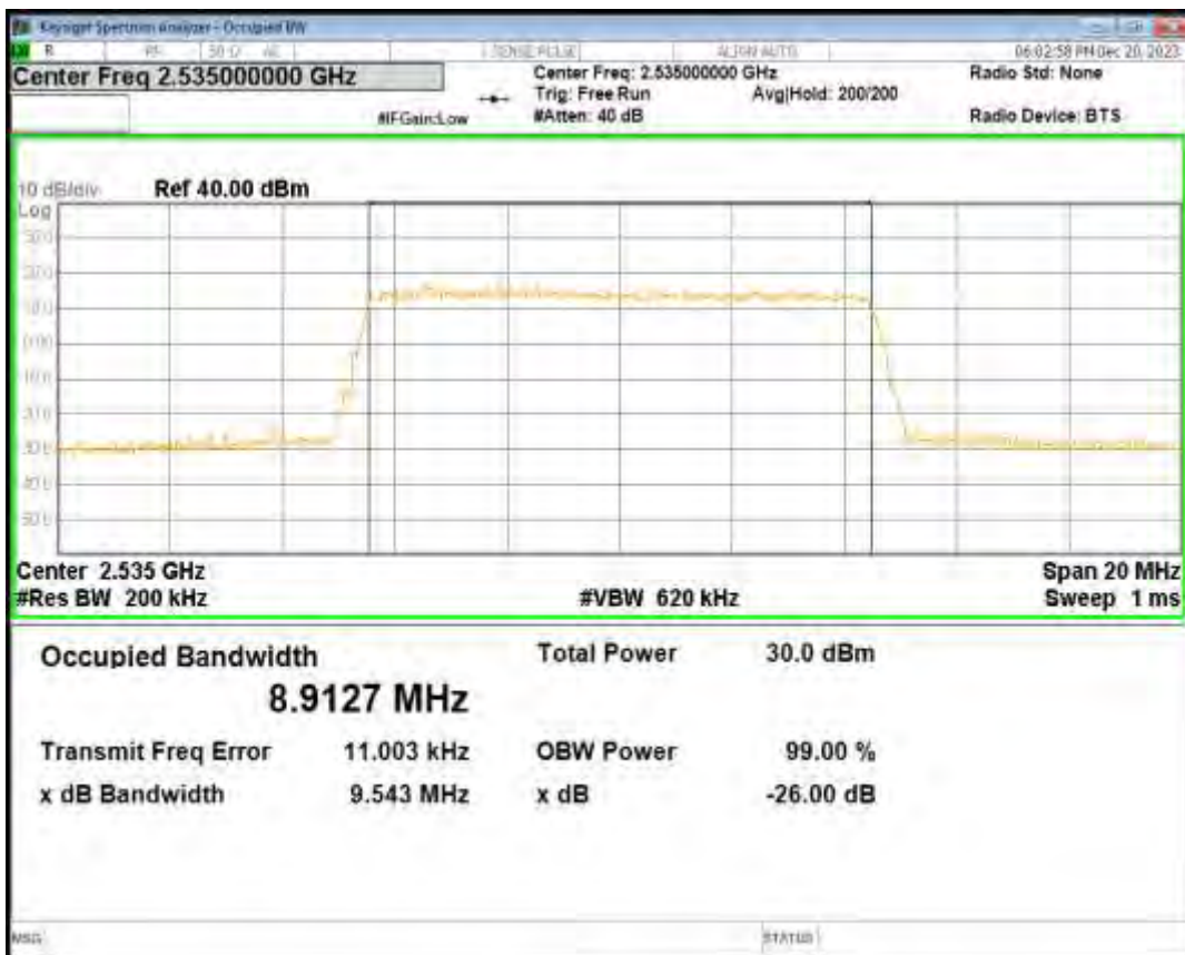
Band7 QPSK BW=15MHz Channel=21100 RB Size=75 Position=#0
