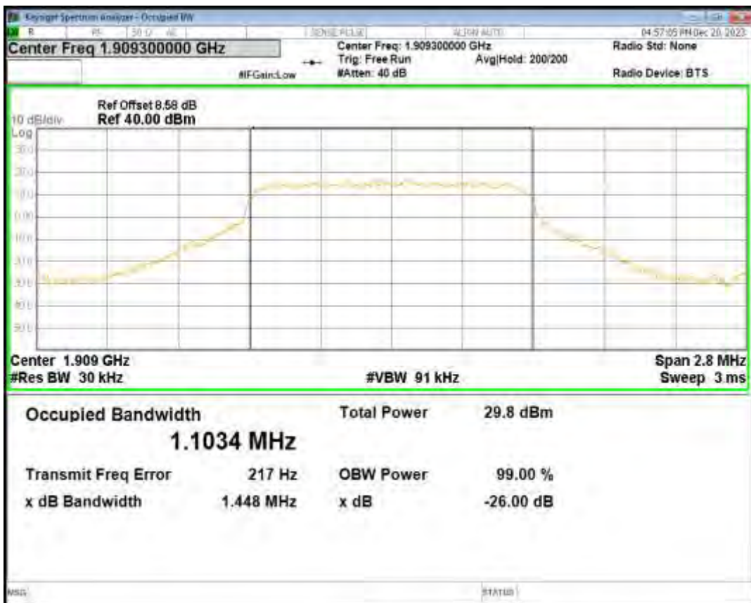
Band2 16QAM BW=1.4MHz Channel=19193 RB Size=6 Position=#0
