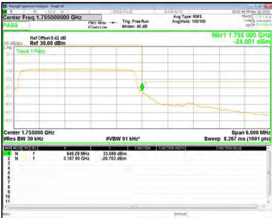
Band4 QPSK BW=5MHz Channel=19975 RB Size=25 Position=#0
