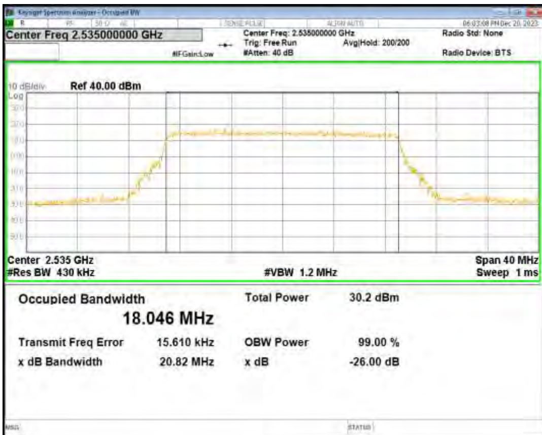
Band7 QPSK BW=20MHz Channel=21100 RB Size=100 Position=#0
