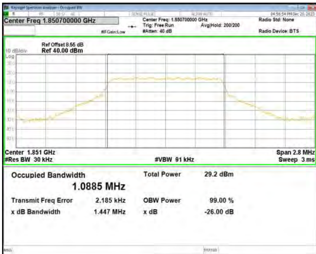
Band2 16QAM BW=1.4MHz Channel=18607 RB Size=6 Position=#0
