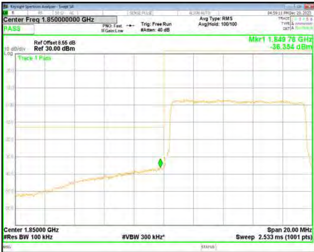
Band2 QPSK BW=10MHz Channel=19150 RB Size=50 Position=#0
