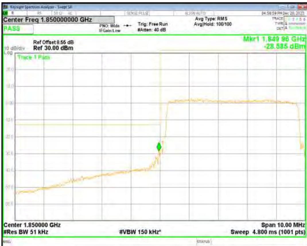
Band2 QPSK BW=5MHz Channel=19175 RB Size=25 Position=#0
