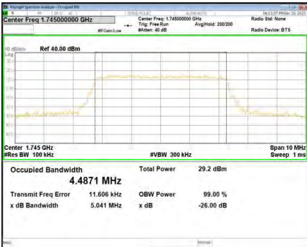
Band66 QPSK BW=10MHz Channel=132322 RB Size=50 Position=#0
