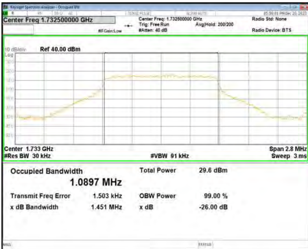
Band4 16QAM BW=1.4MHz Channel=20175 RB Size=6 Position=#0
