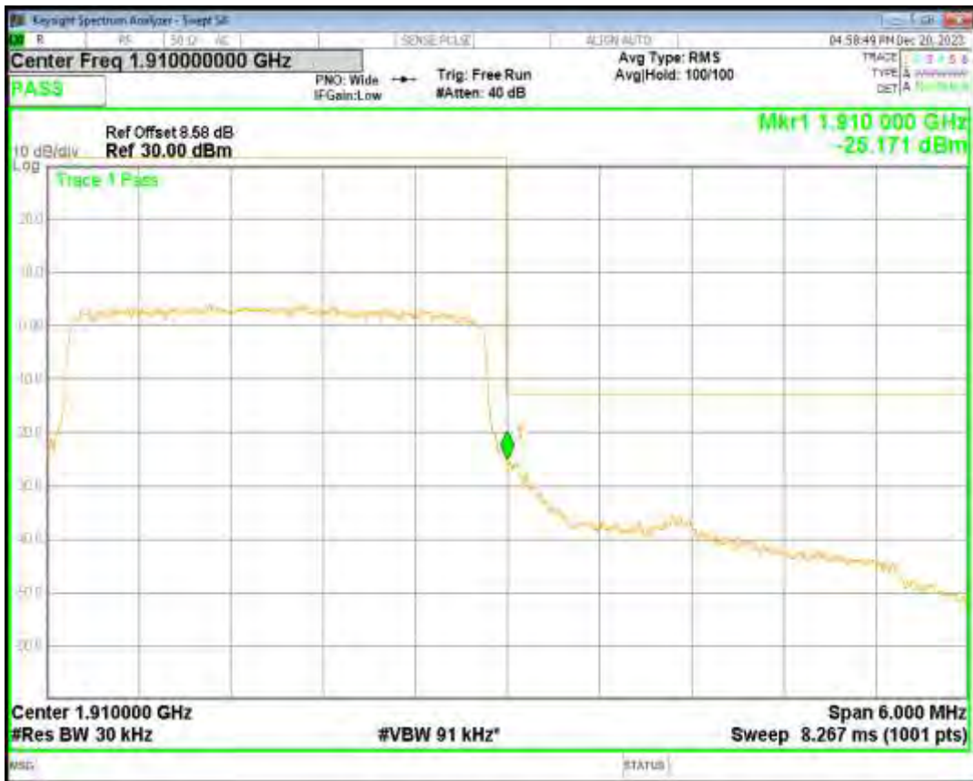
Band2 16QAM BW=3MHz Channel=19185 RB Size=15 Position=#0
