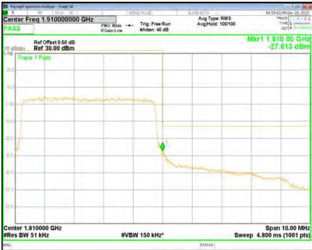
Band2 16QAM BW=5MHz Channel=19175 RB Size=25 Position=#0
