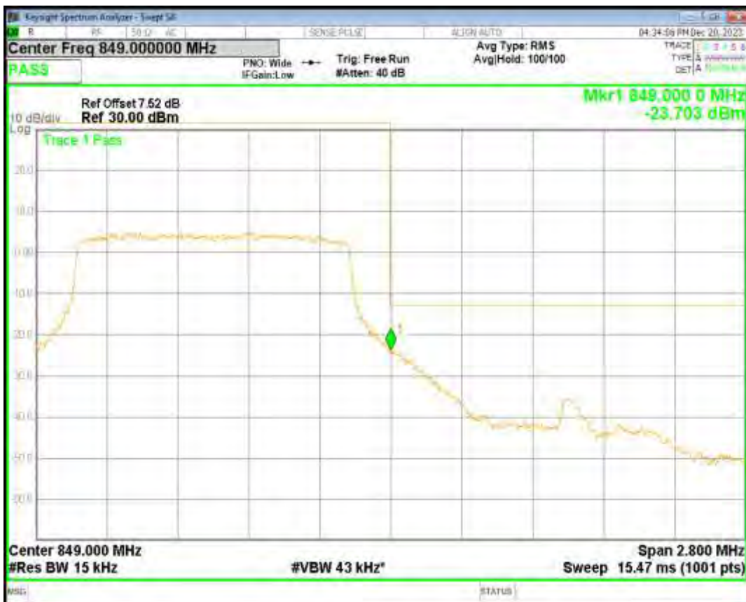
Band5 16QAM BW=1.4MHz Channel=20643 RB Size=6 Position=#0
