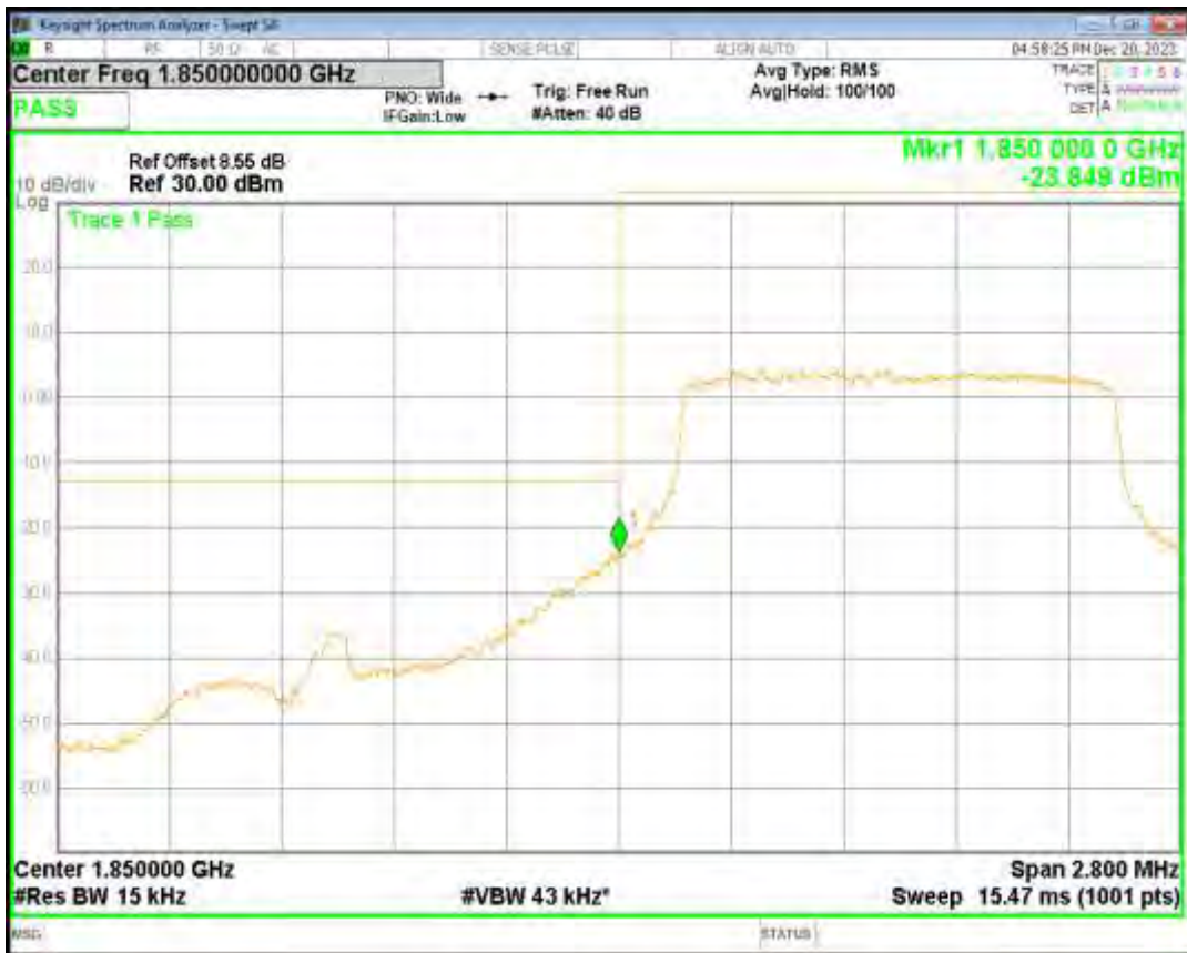
Band2 16QAM BW=1.4MHz Channel=18607 RB Size=6 Position=#0
