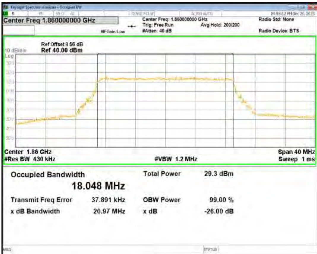
Band2 QPSK BW=20MHz Channel=18900 RB Size=100 Position=#0
