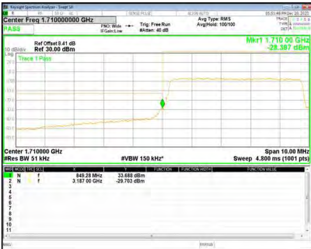
Band4 QPSK BW=5MHz Channel=20375 RB Size=25 Position=#0
