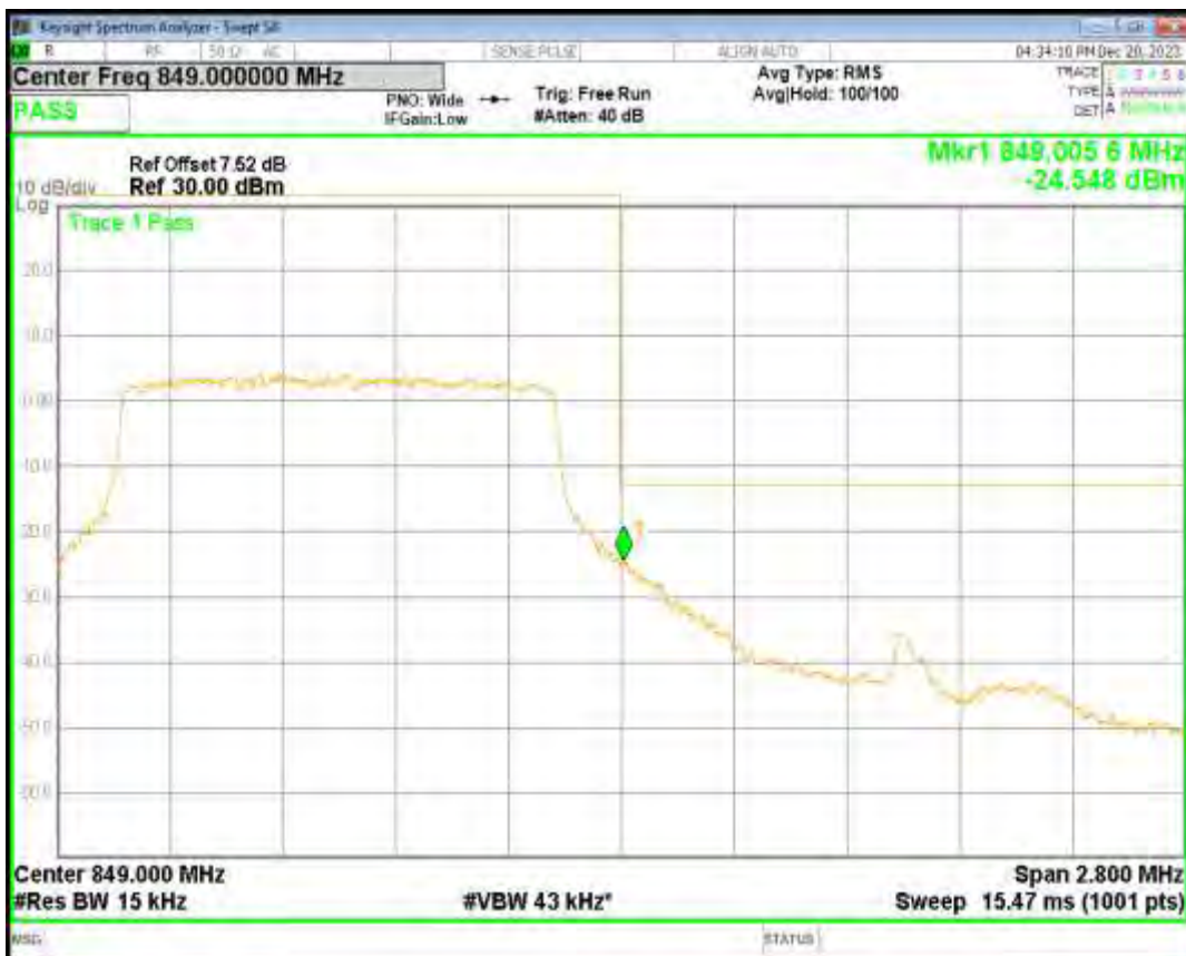
Band5 QPSK BW=3MHz Channel=20415 RB Size=15 Position=#0
