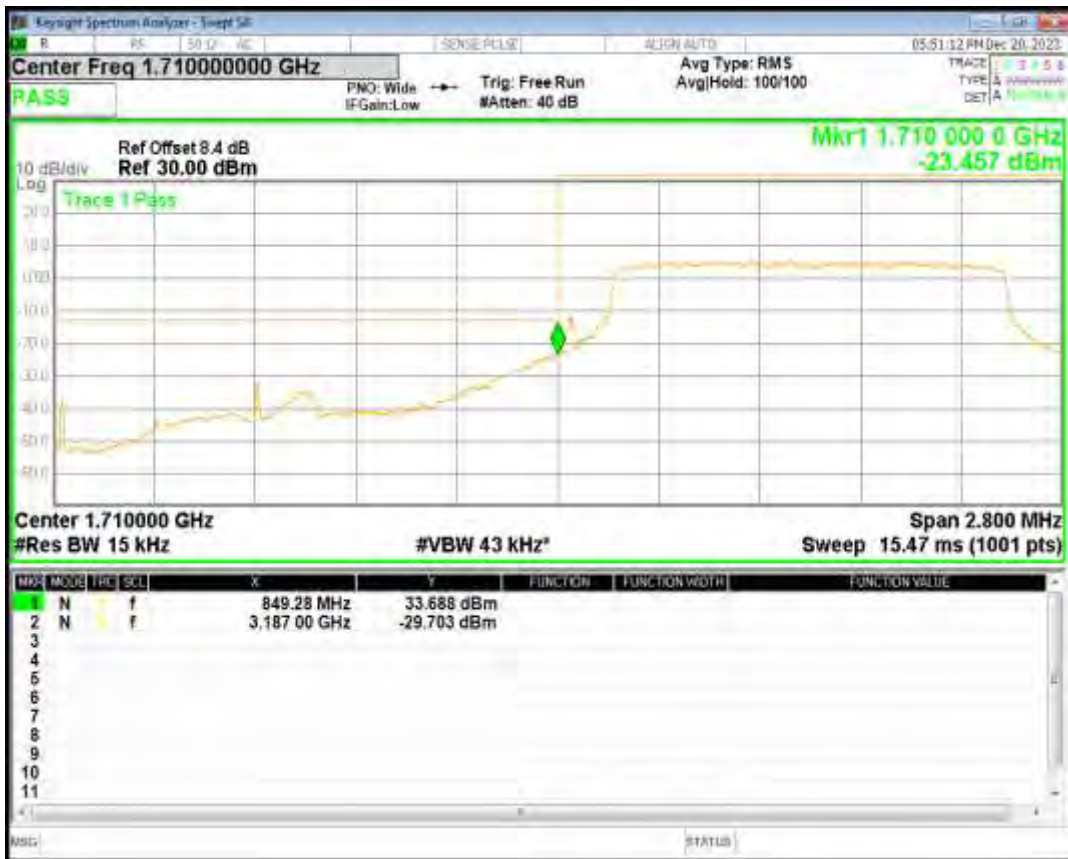
Band4 16QAM BW=1.4MHz Channel=19957 RB Size=6 Position=#0
