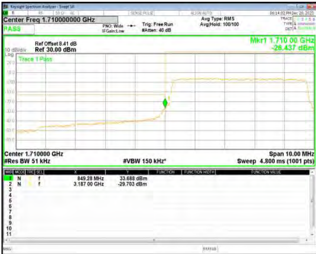
Band66 16QAM BW=5MHz Channel=131997 RB Size=25 Position=#0
