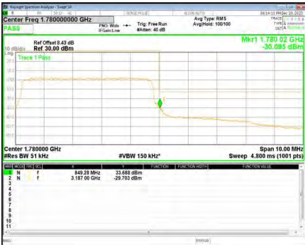
Band66 QPSK BW=10MHz Channel=132022 RB Size=50 Position=#0
