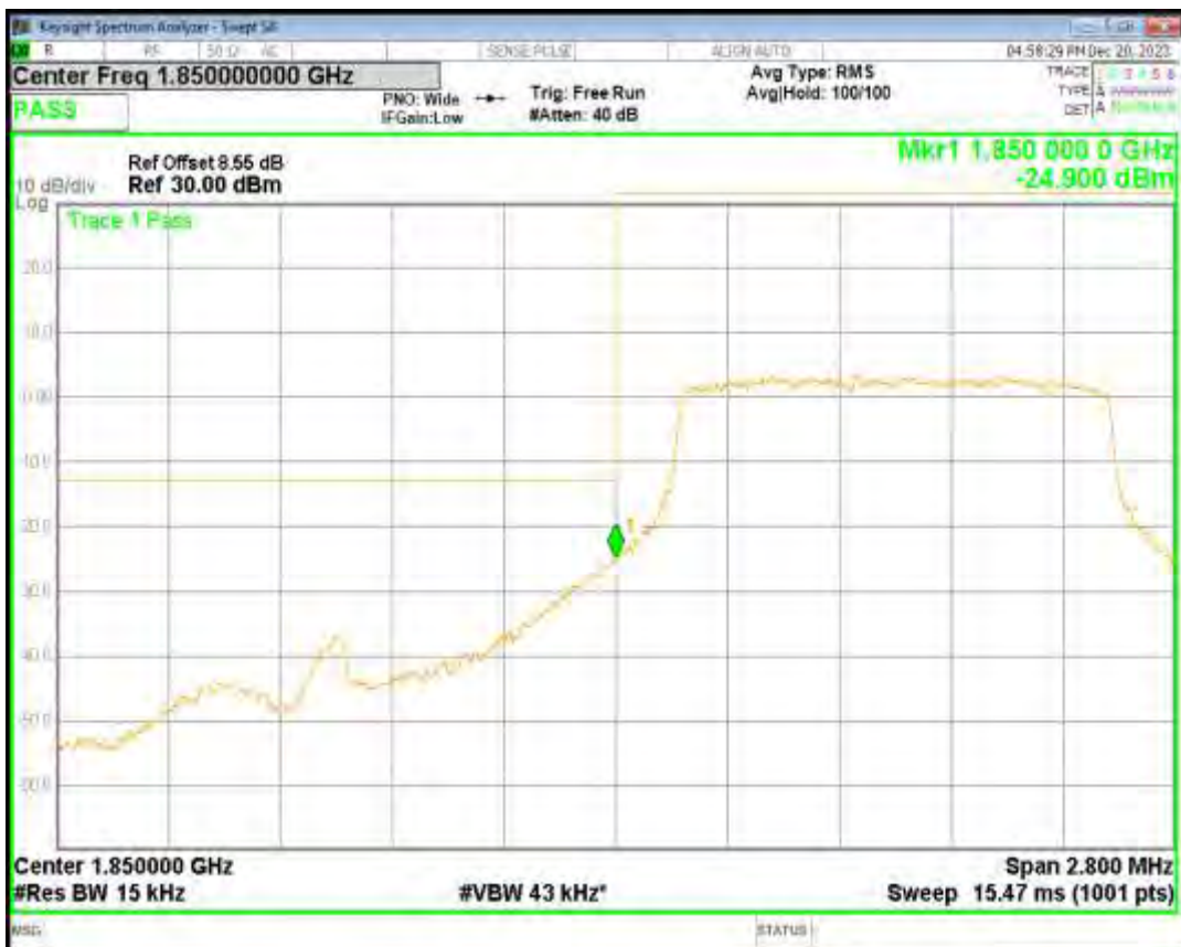
Band2 QPSK BW=1.4MHz Channel=19193 RB Size=6 Position=#0
