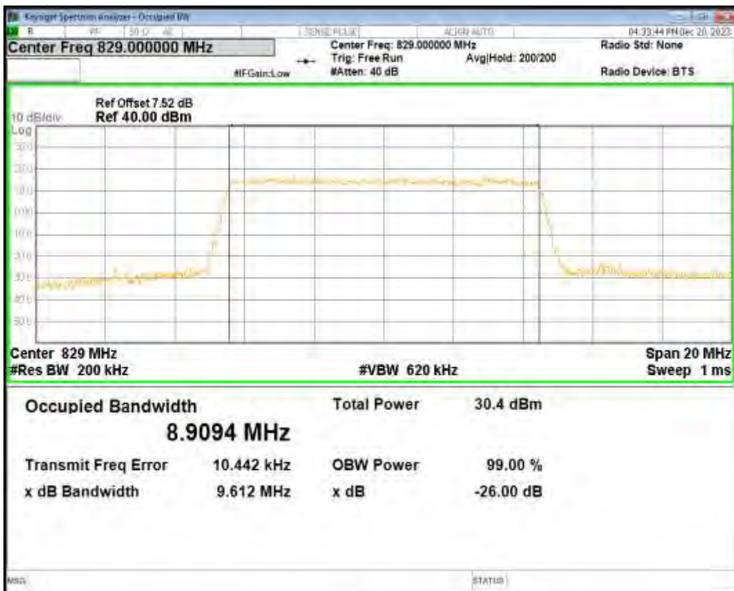
Band5 QPSK BW=10MHz Channel=20525 RB Size=50 Position=#0
