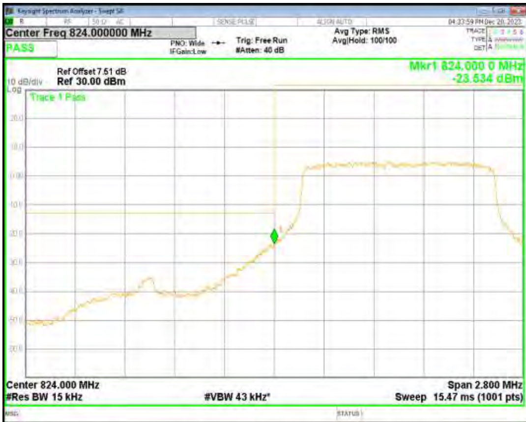
Band5 16QAM BW=1.4MHz Channel=20407 RB Size=6 Position=#0
