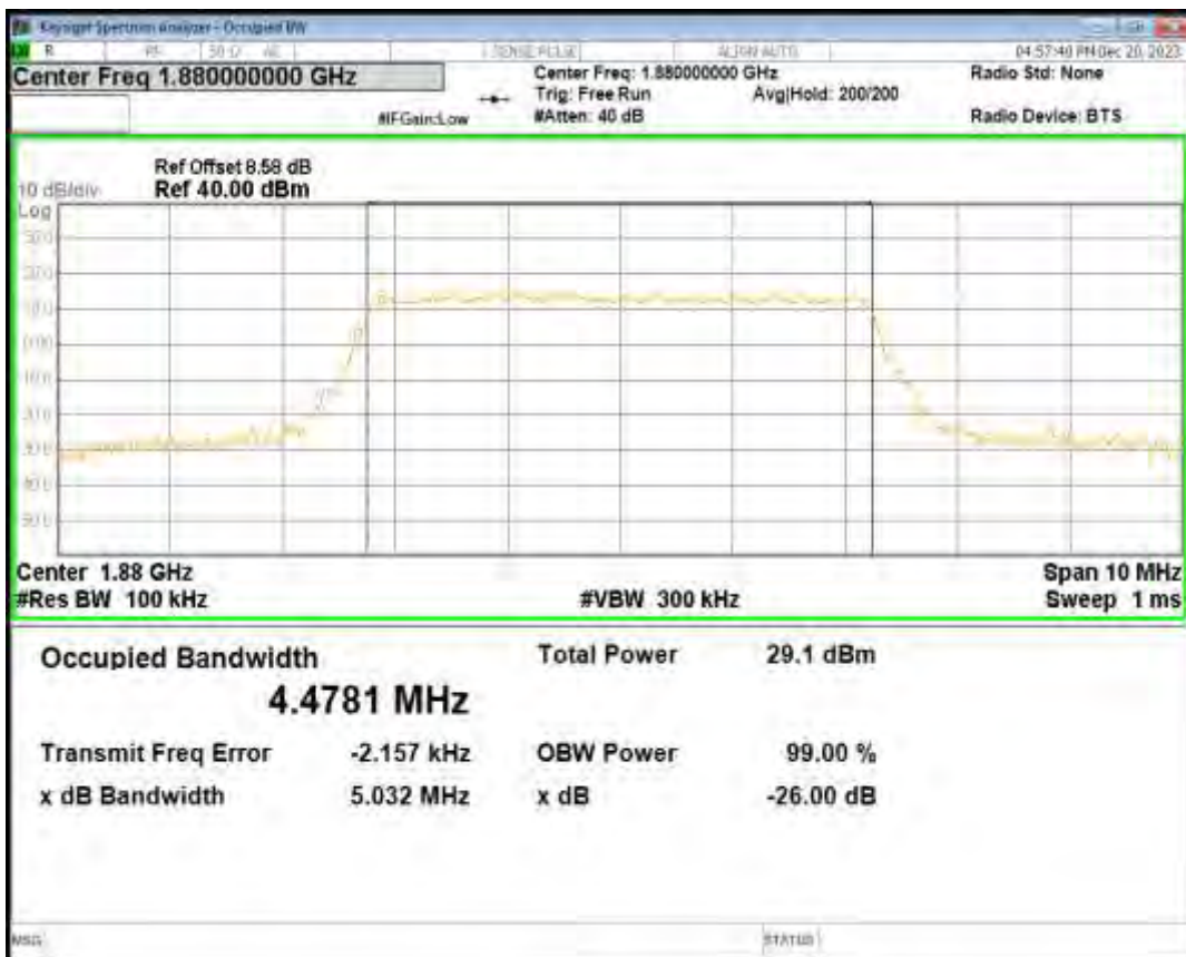
Band2 QPSK BW=5MHz Channel=19175 RB Size=25 Position=#0
