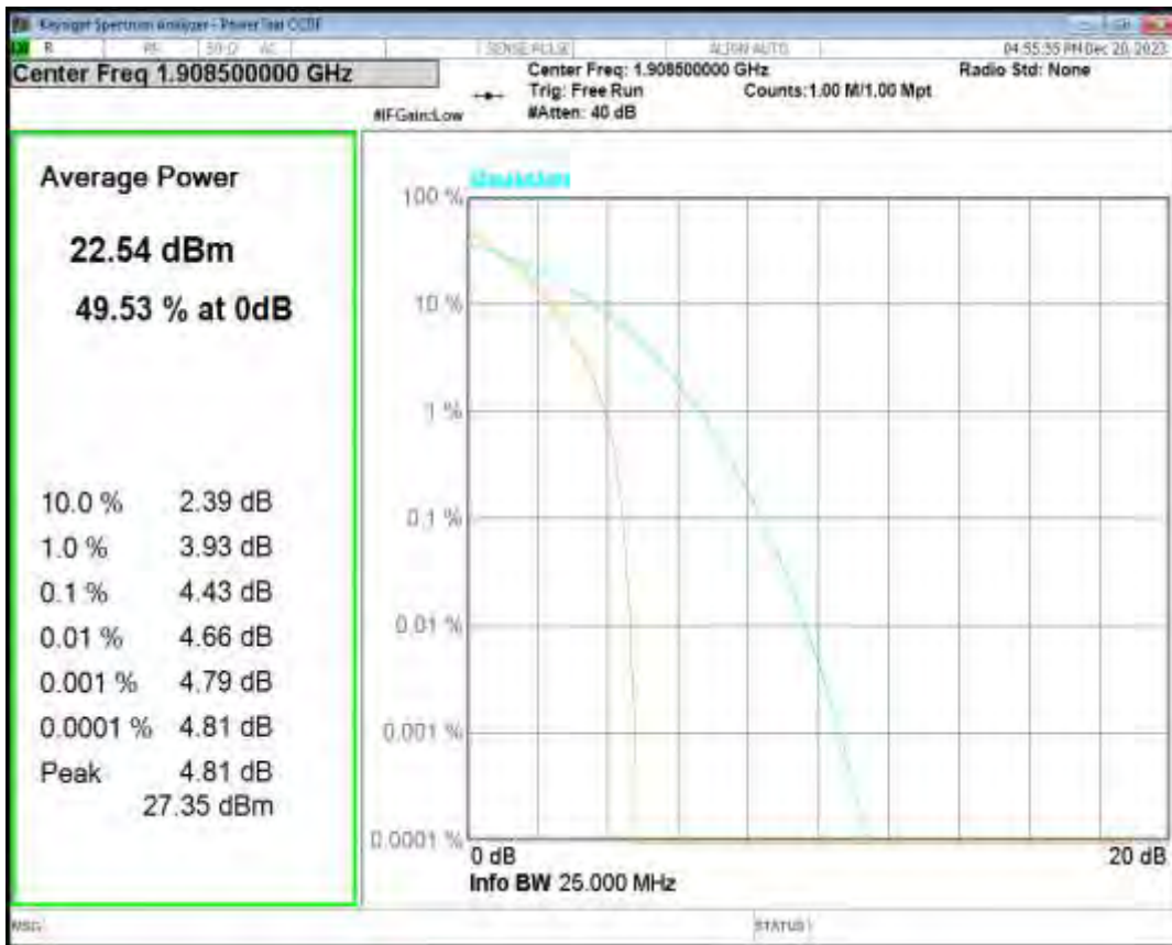
Band2 16QAM BW=3MHz Channel=19185 RB Size=1 Position=#0
