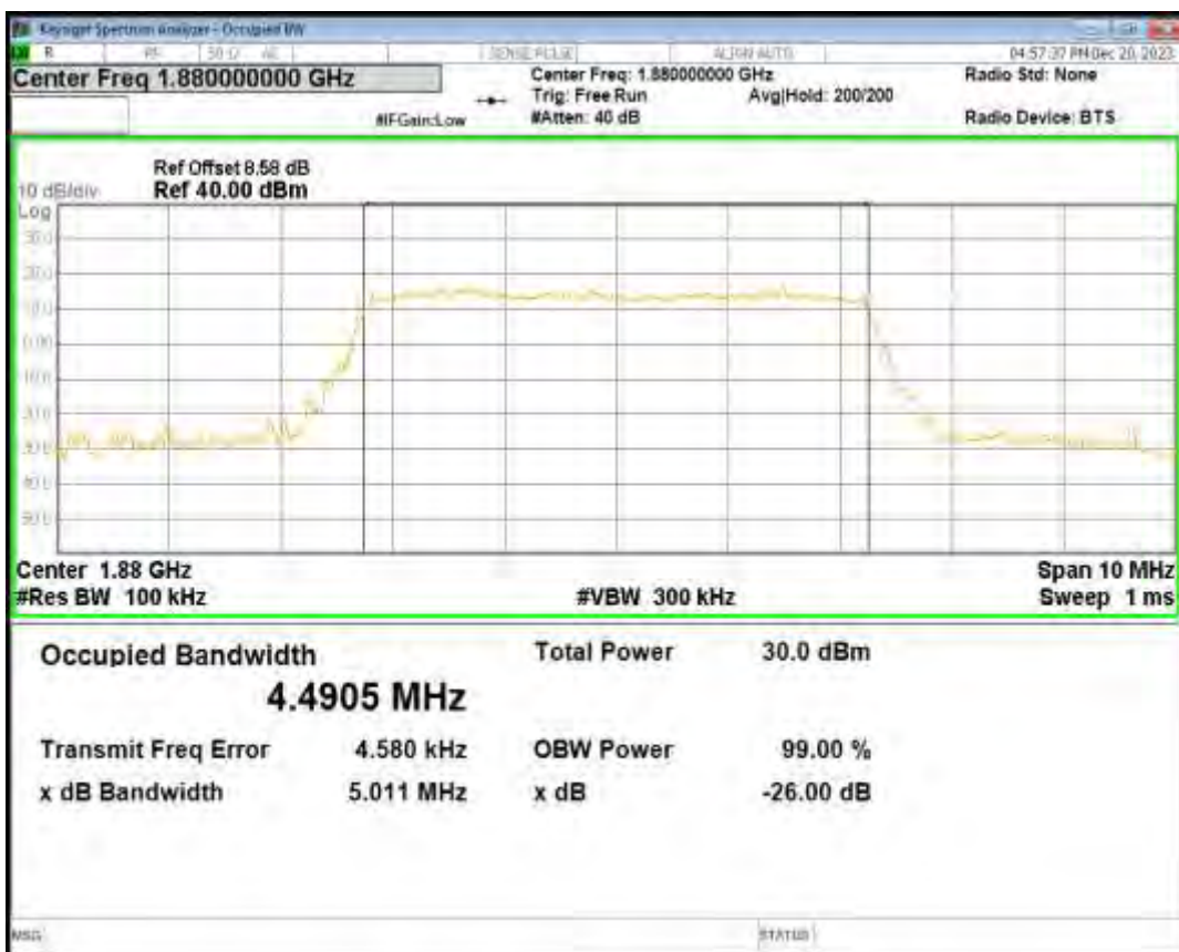
Band2 16QAM BW=5MHz Channel=18900 RB Size=25 Position=#0
