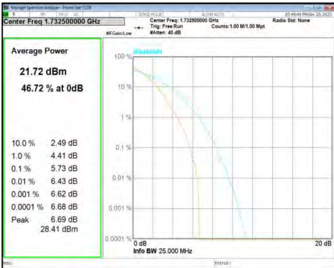
Band4 QPSK BW=15MHz Channel=20175 RB Size=1 Position=#0
