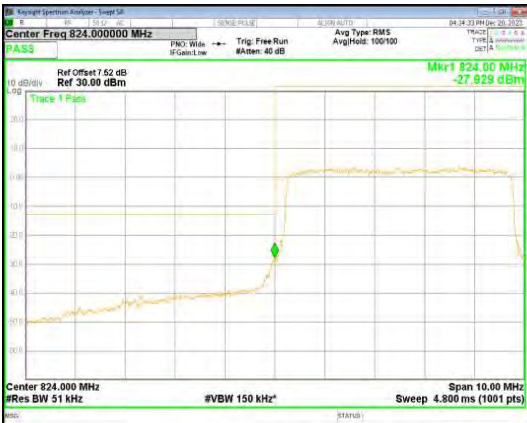
Band5 QPSK BW=5MHz Channel=20625 RB Size=25 Position=#0
