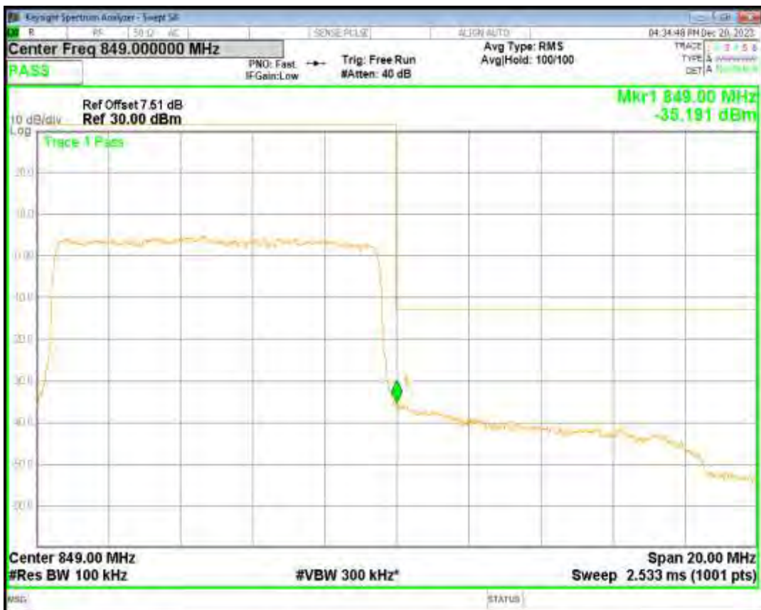
Band66 QPSK BW=1.4MHz Channel=131979 RB Size=6 Position=#0
