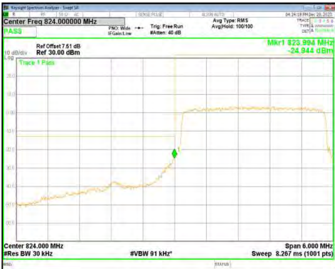
Band5 QPSK BW=3MHz Channel=20635 RB Size=15 Position=#0
