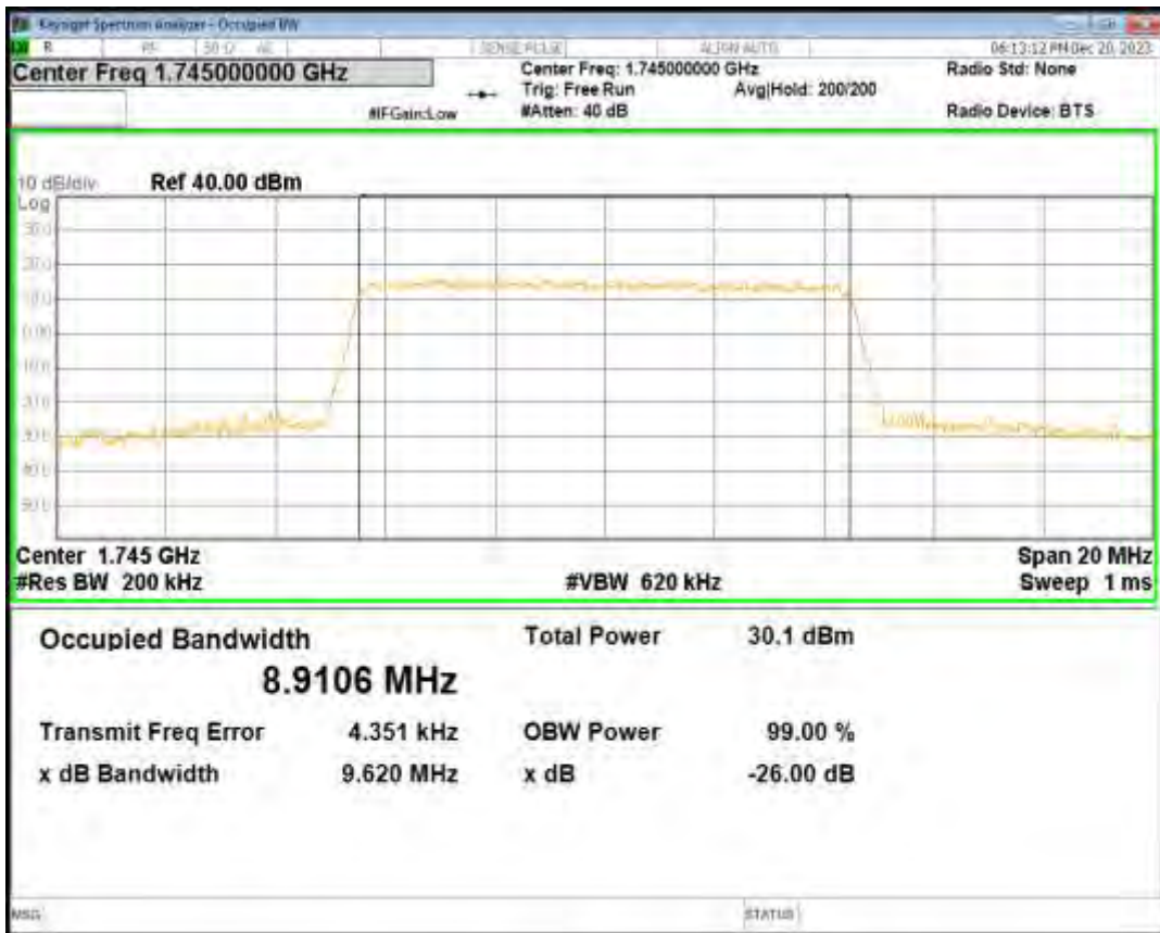
Band66 QPSK BW=15MHz Channel=132322 RB Size=75 Position=#0
