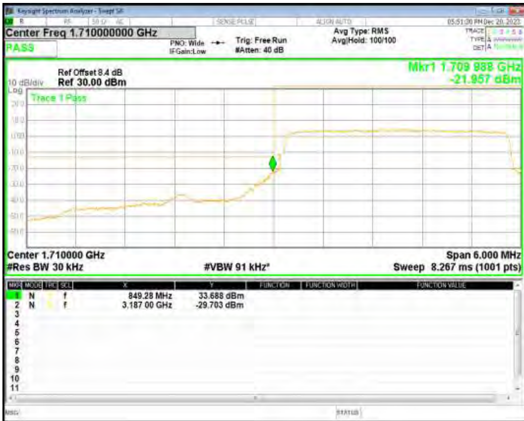
Band4 16QAM BW=3MHz Channel=19965 RB Size=15 Position=#0
