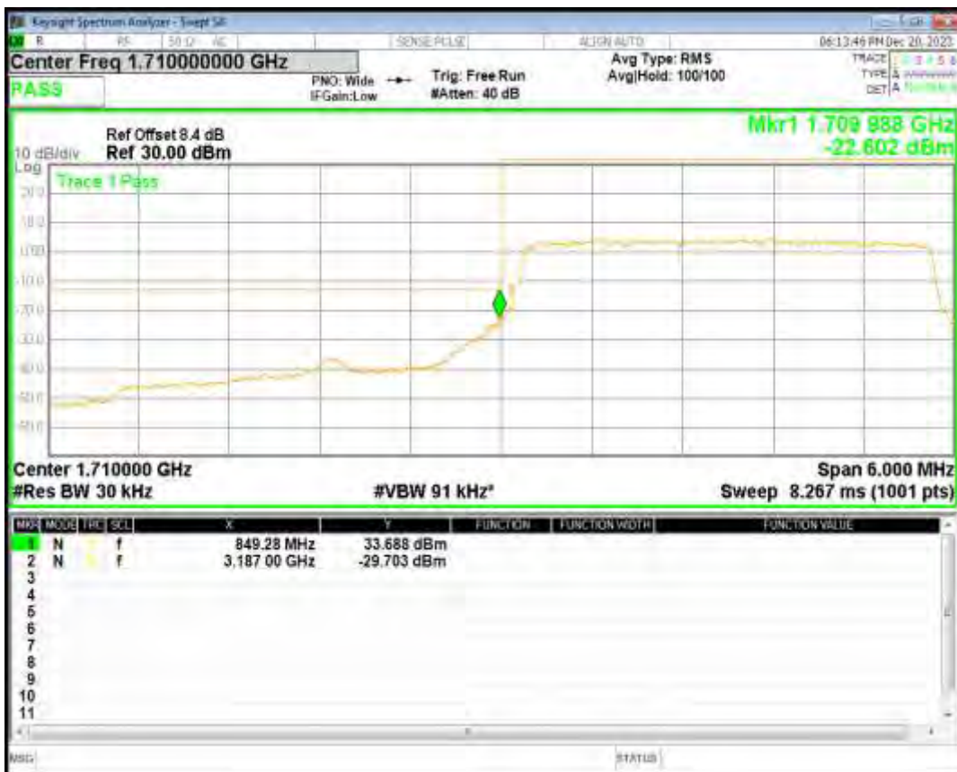
Band66 16QAM BW=3MHz Channel=131987 RB Size=15 Position=#0
