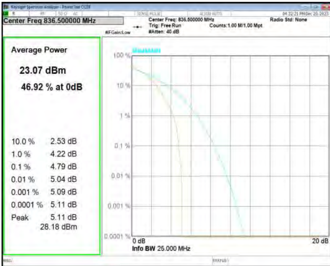
Band5 16QAM BW=5MHz Channel=20525 RB Size=1 Position=#0
