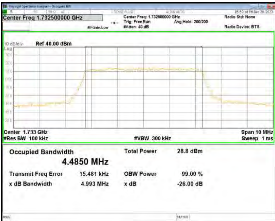
Band4 QPSK BW=10MHz Channel=20175 RB Size=50 Position=#0
