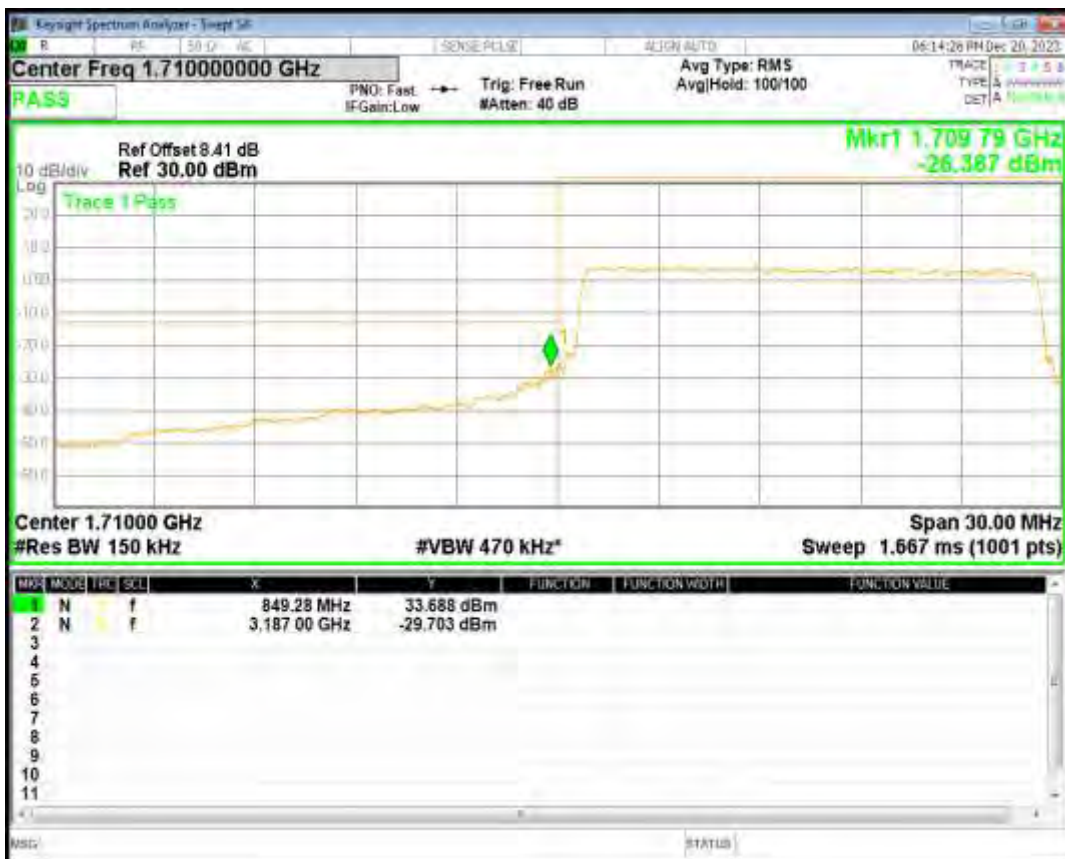
Band66 QPSK BW=15MHz Channel=132597 RB Size=75 Position=#0
