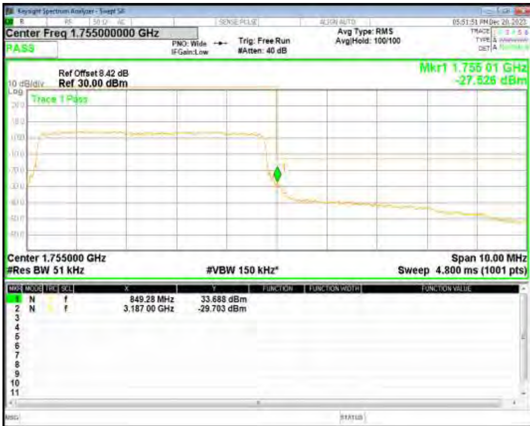
Band4 16QAM BW=5MHz Channel=20375 RB Size=25 Position=#0
