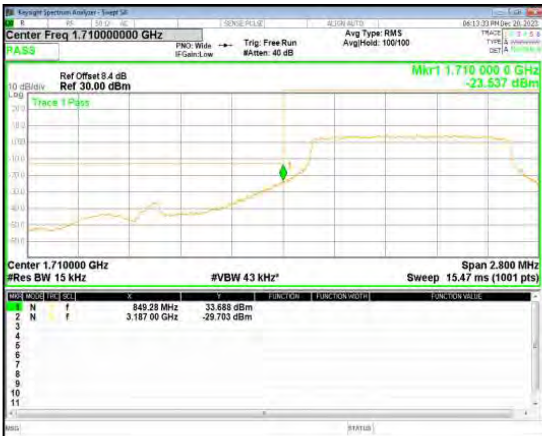
Band66 QPSK BW=1.4MHz Channel=132665 RB Size=6 Position=#0
