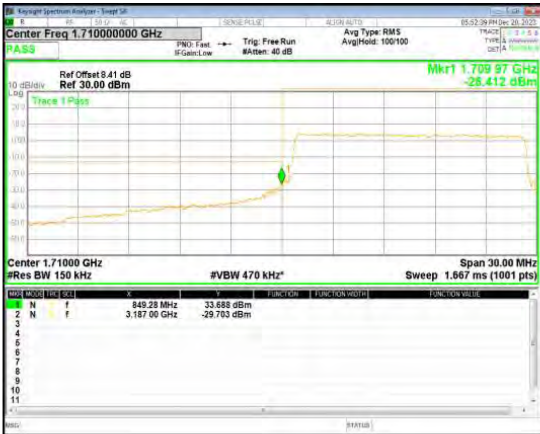
Band4 QPSK BW=15MHz Channel=20325 RB Size=75 Position=#0
