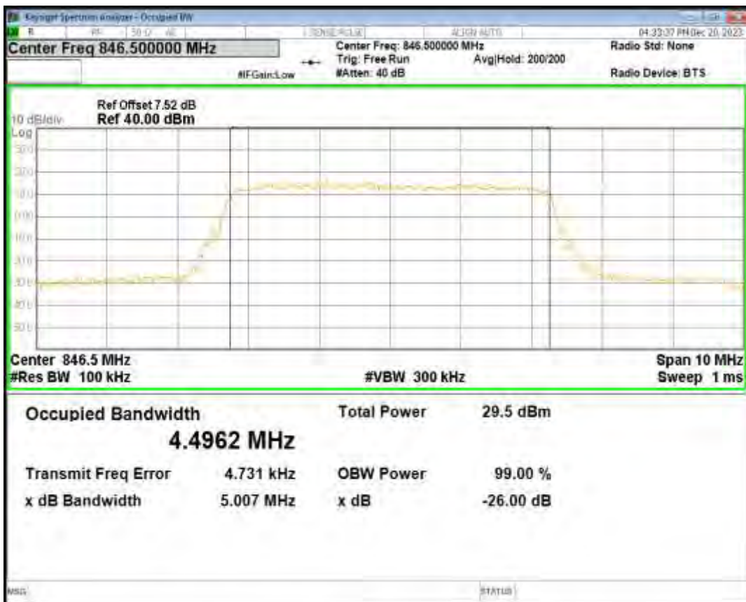
Band5 QPSK BW=10MHz Channel=20450 RB Size=50 Position=#0
