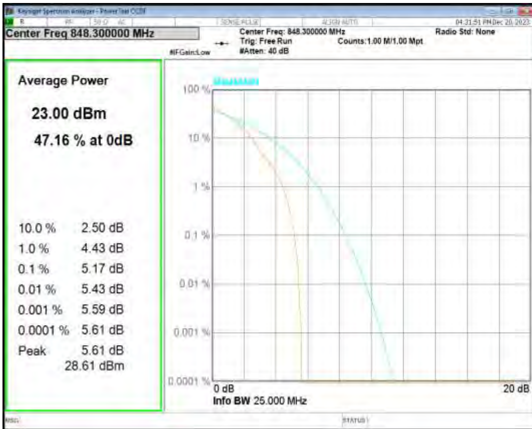
Band5 16QAM BW=1.4MHz Channel=20643 RB Size=1 Position=#0
