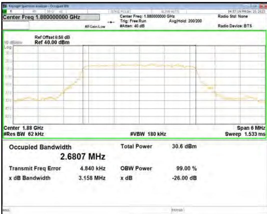
Band2 16QAM BW=3MHz Channel=18900 RB Size=15 Position=#0
