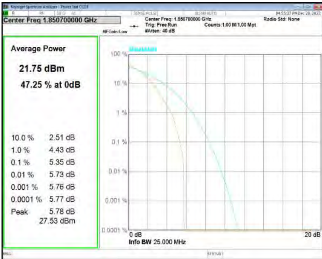
Band2 16QAM BW=1.4MHz Channel=18607 RB Size=1 Position=#0
