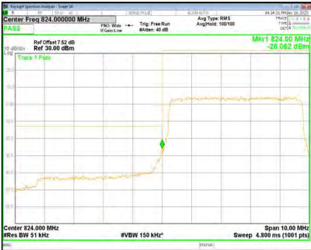
Band5 16QAM BW=5MHz Channel=20425 RB Size=25 Position=#0
