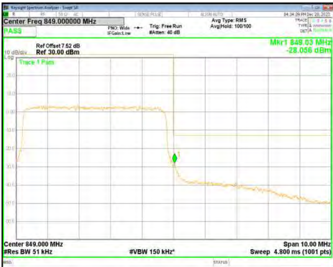
Band5 QPSK BW=10MHz Channel=20450 RB Size=50 Position=#0
