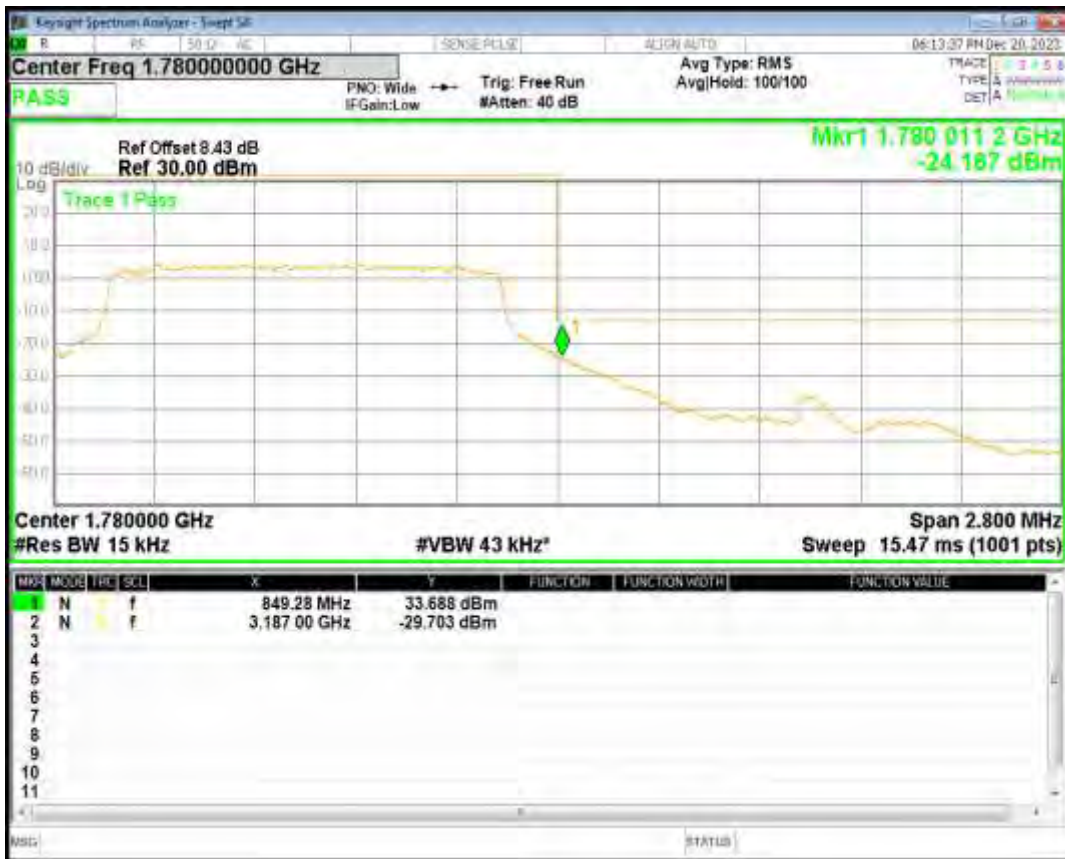
Band66 16QAM BW=1.4MHz Channel=132665 RB Size=6 Position=#0
