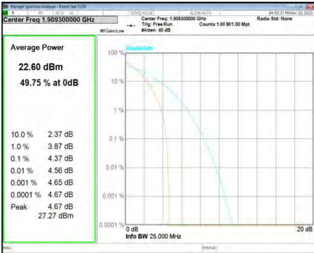
Band2 16QAM BW=1.4MHz Channel=19193 RB Size=1 Position=#0
