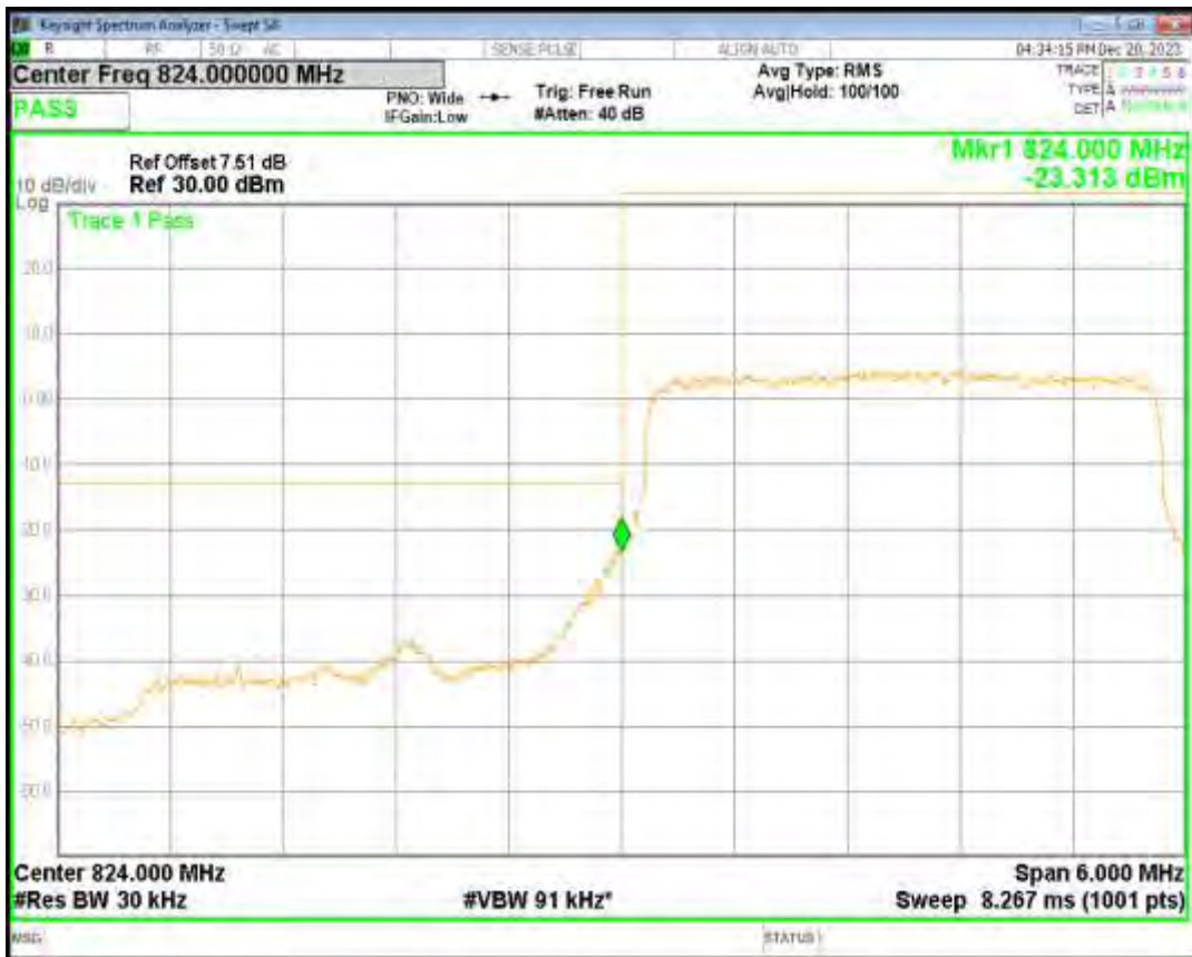
Band5 16QAM BW=3MHz Channel=20415 RB Size=15 Position=#0
