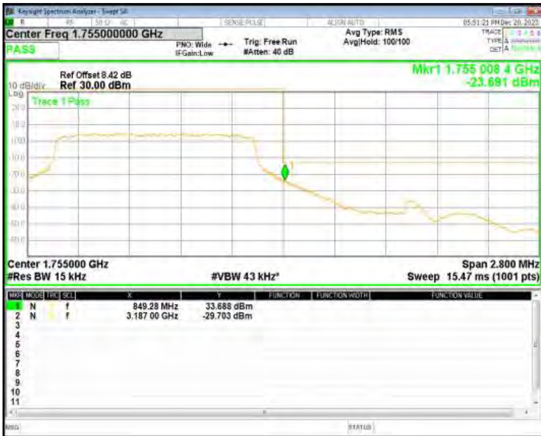
Band4 16QAM BW=1.4MHz Channel=20393 RB Size=6 Position=#0
