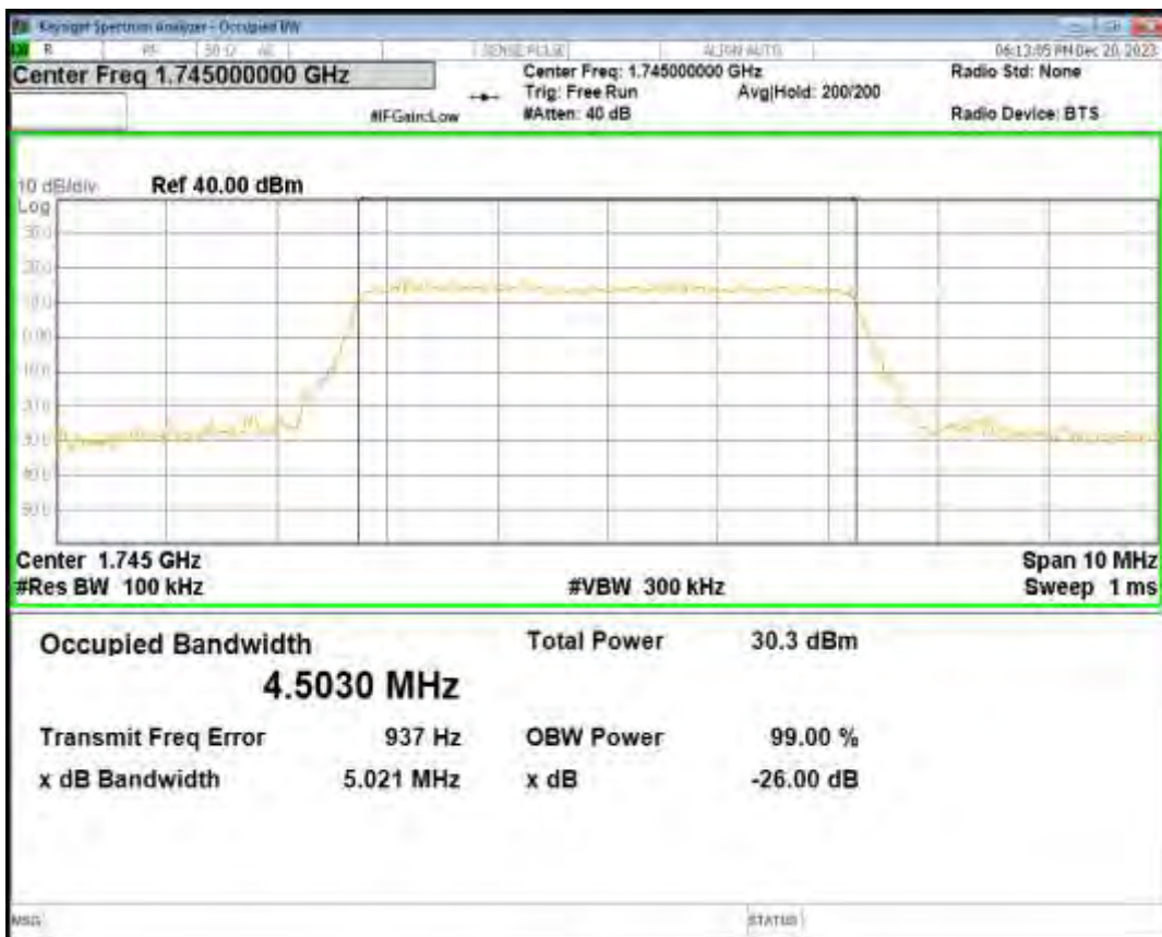
Band66 16QAM BW=5MHz Channel=132322 RB Size=25 Position=#0
