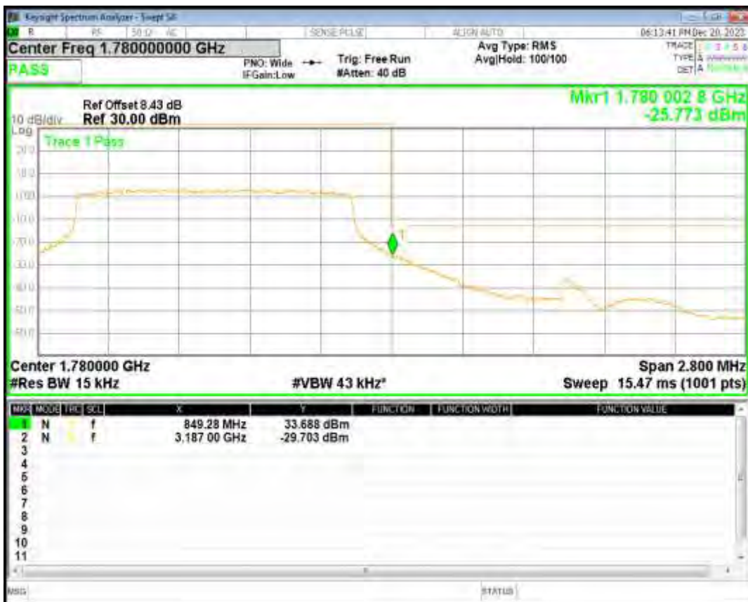
Band66 QPSK BW=3MHz Channel=131987 RB Size=15 Position=#0
