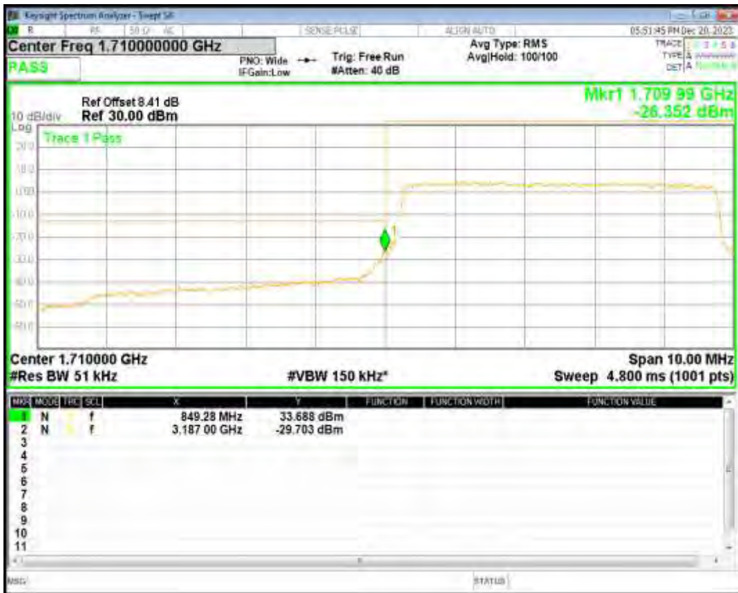
Band4 16QAM BW=5MHz Channel=19975 RB Size=25 Position=#0
