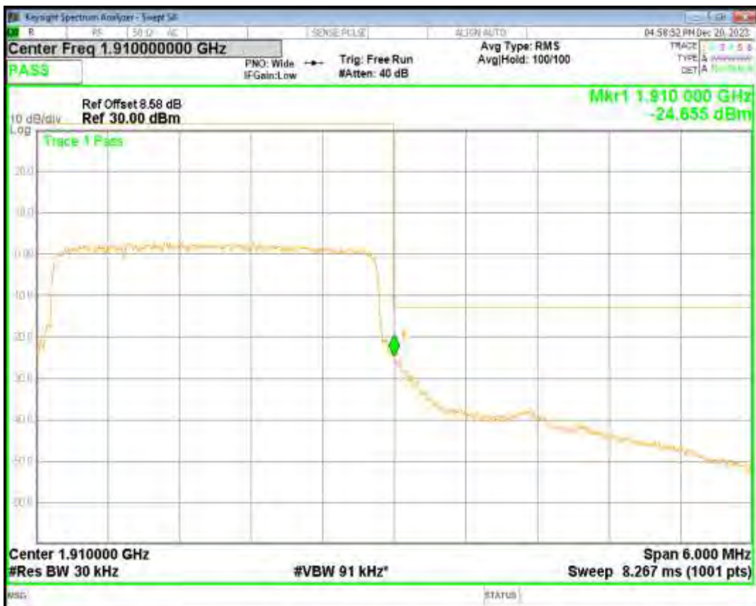
Band2 QPSK BW=5MHz Channel=18625 RB Size=25 Position=#0
