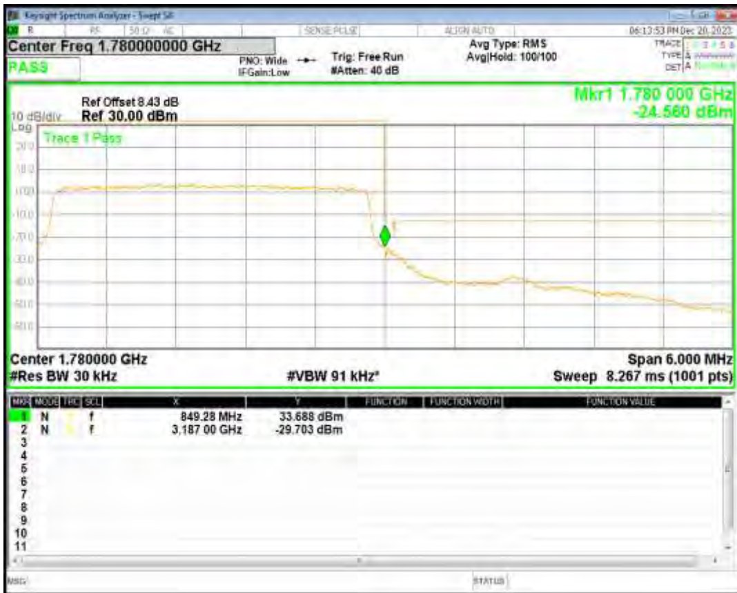
Band66 16QAM BW=3MHz Channel=132657 RB Size=15 Position=#0
