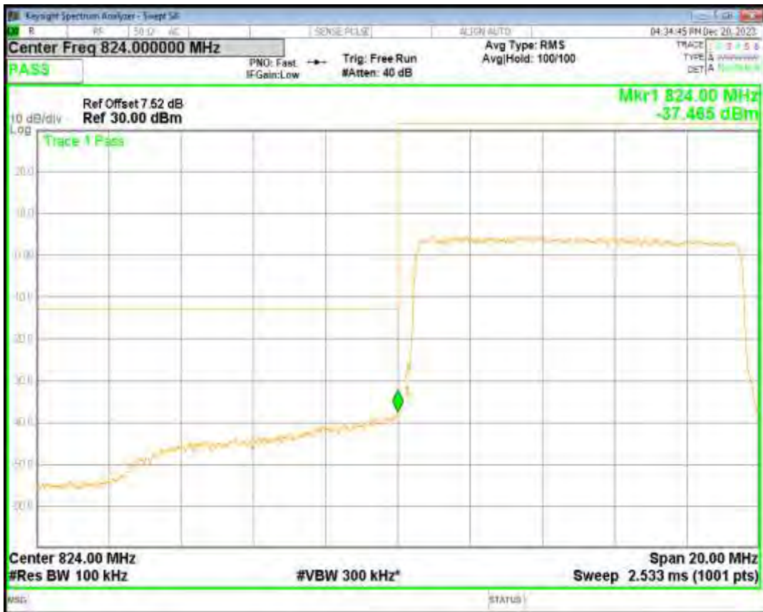
Band5 QPSK BW=10MHz Channel=20600 RB Size=50 Position=#0
