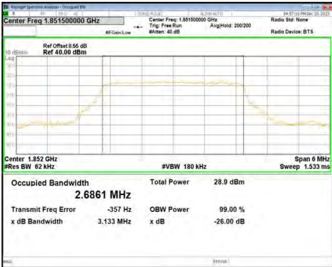
Band2 QPSK BW=3MHz Channel=18900 RB Size=15 Position=#0
