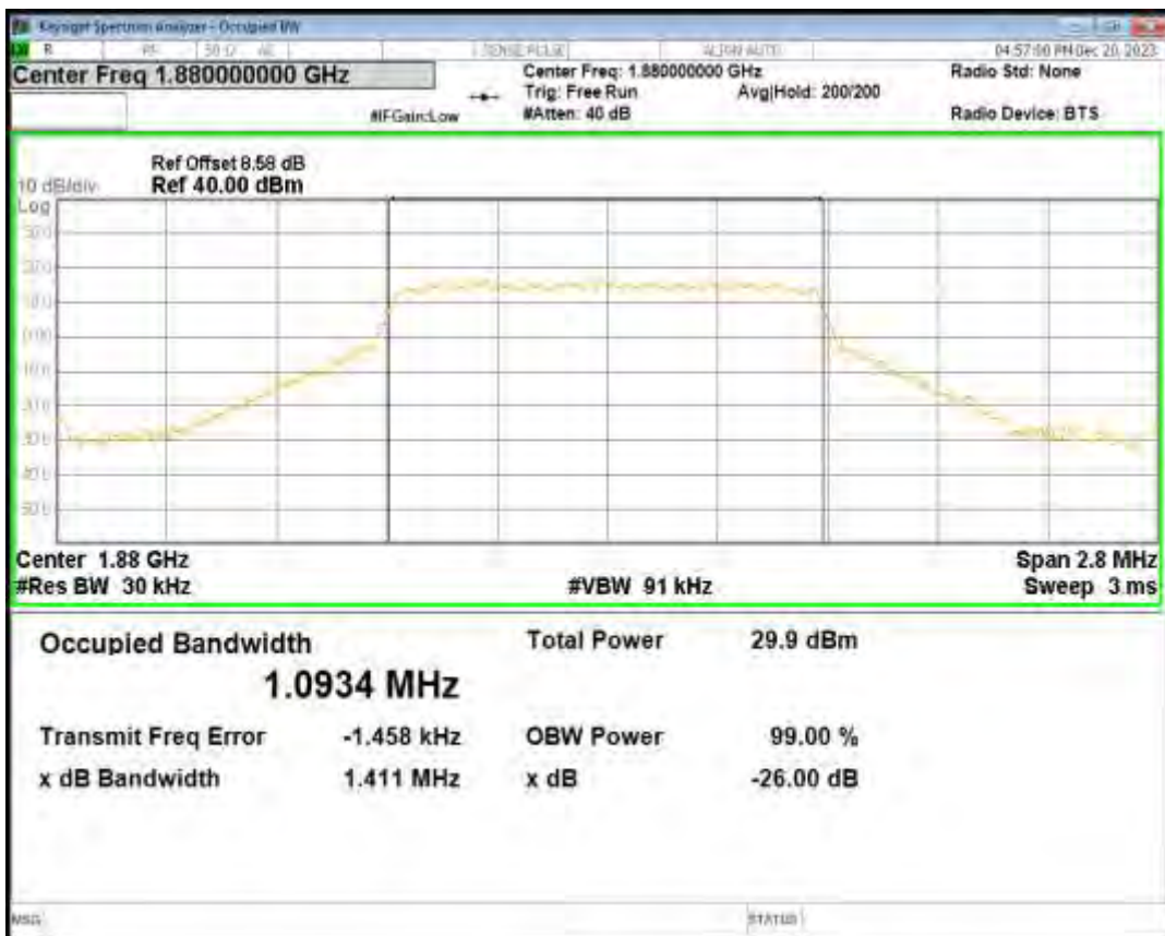
Band2 16QAM BW=1.4MHz Channel=18900 RB Size=6 Position=#0
