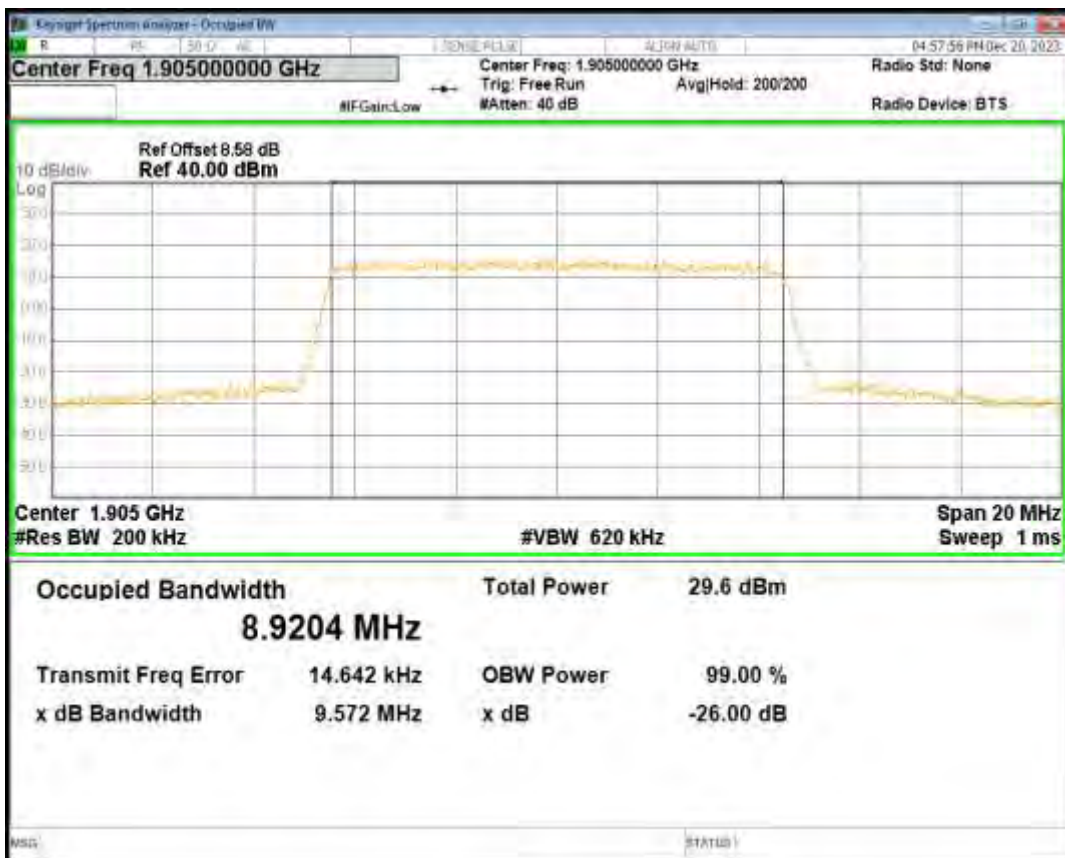
Band2 QPSK BW=15MHz Channel=18675 RB Size=75 Position=#0
