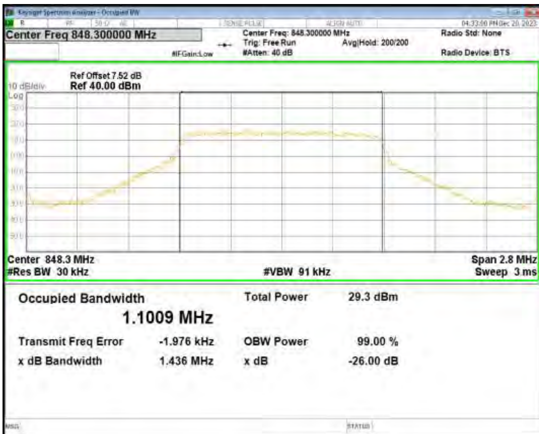
Band5 QPSK BW=3MHz Channel=20415 RB Size=15 Position=#0
