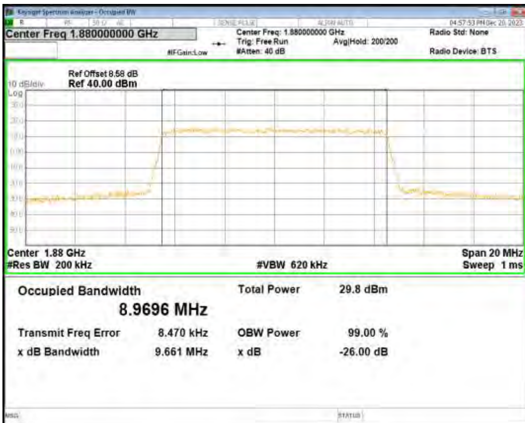
Band2 QPSK BW=10MHz Channel=19150 RB Size=50 Position=#0
