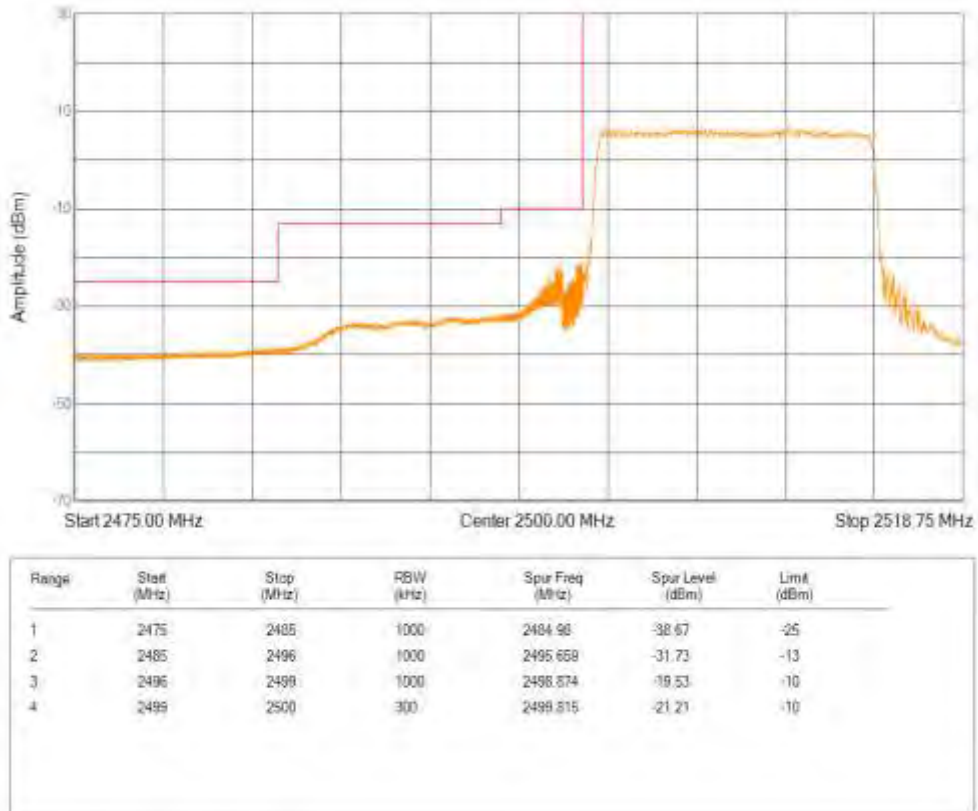
Band7 QPSK BW=15MHz Channel=21375 RB Size=75 Position=#0
