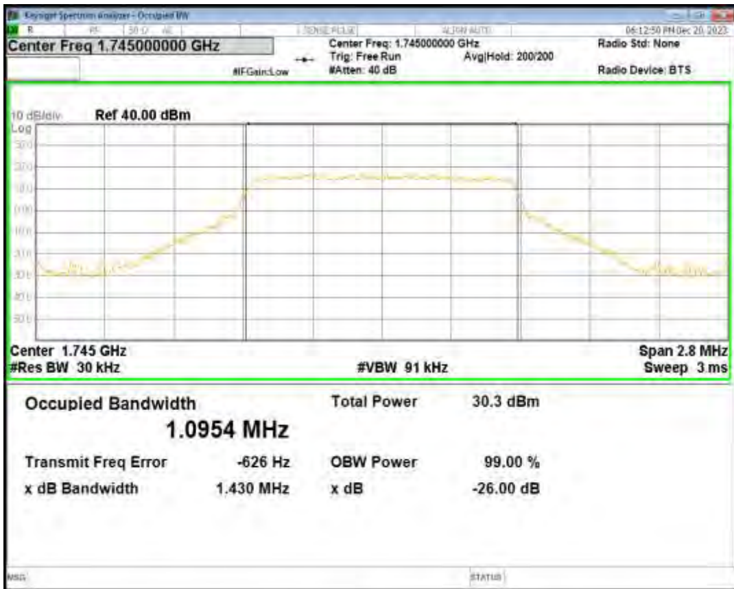
Band66 16QAM BW=1.4MHz Channel=132322 RB Size=6 Position=#0
