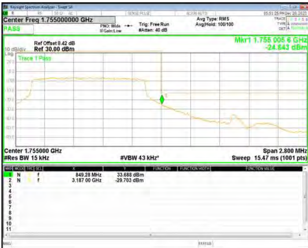
Band4 QPSK BW=3MHz Channel=19965 RB Size=15 Position=#0
