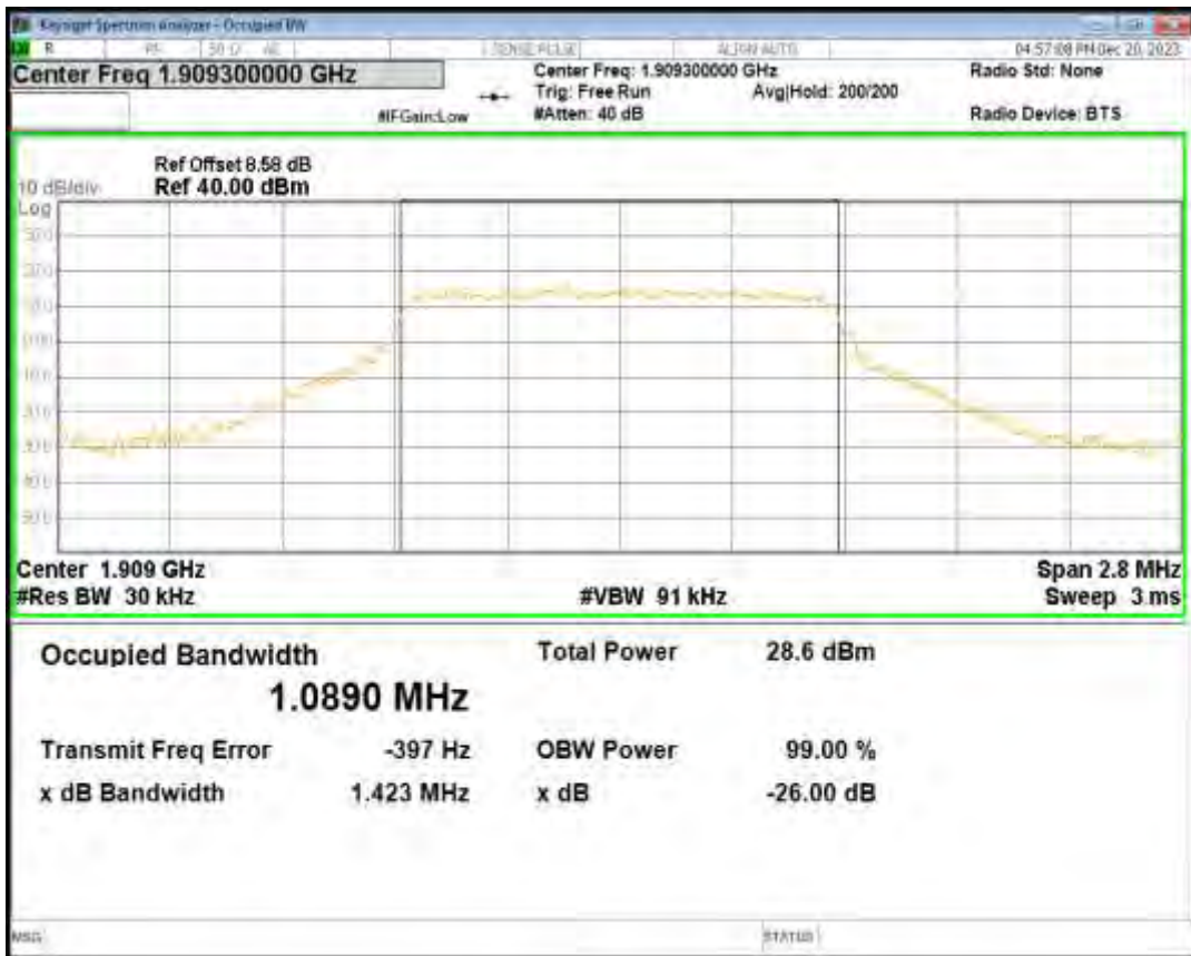
Band2 QPSK BW=3MHz Channel=18615 RB Size=15 Position=#0
