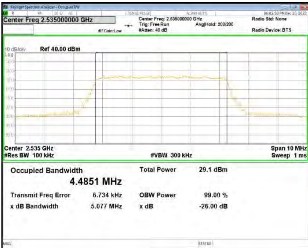
Band7 QPSK BW=10MHz Channel=21100 RB Size=50 Position=#0
