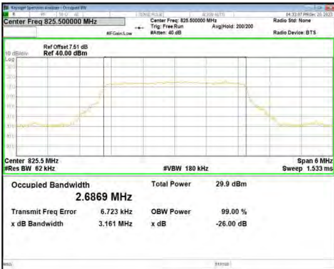
Band5 QPSK BW=3MHz Channel=20525 RB Size=15 Position=#0
