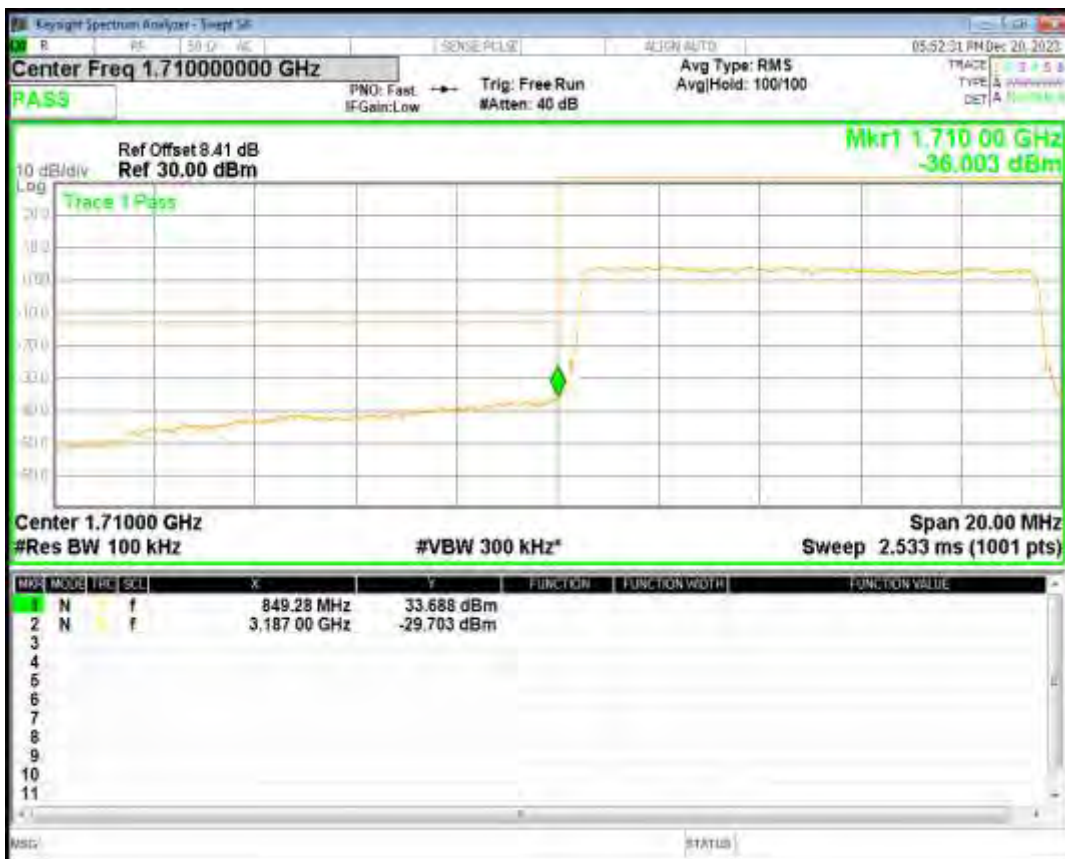
Band4 QPSK BW=10MHz Channel=20350 RB Size=50 Position=#0
