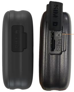
Insert the SIM card according to the direction of this picture, press the SIM card to the end, and hear the click before it is in place.
